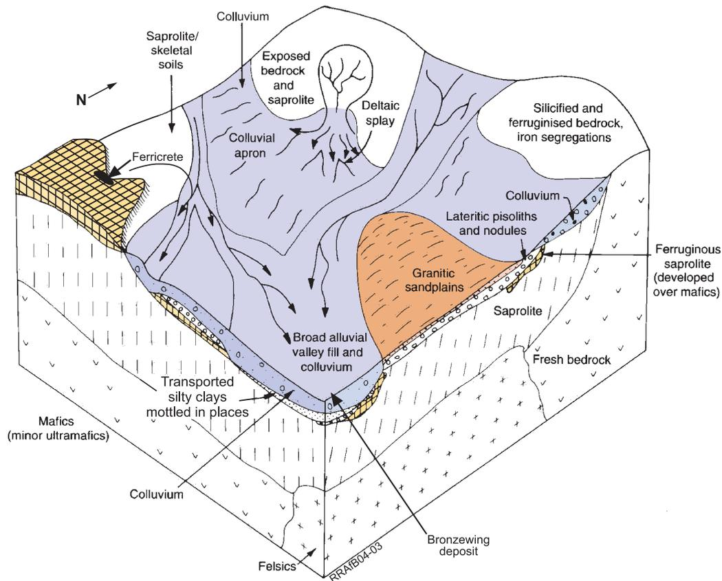
Figure 4. Idealised block diagram model showing regolith–landform relationship for the Bronzewing district.
