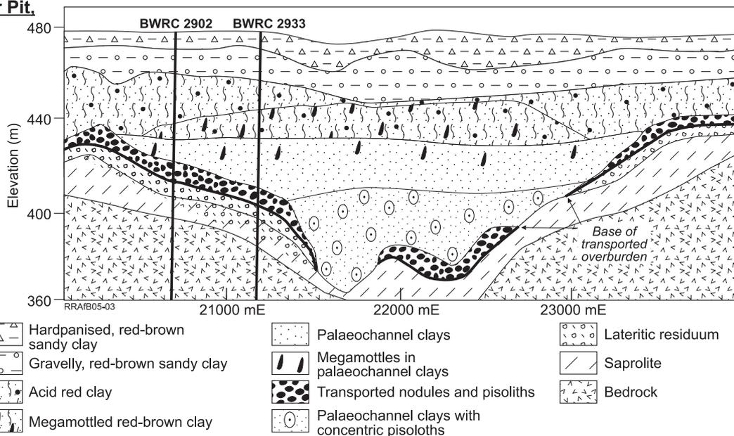
Figure 5. Regolith stratigraphy for the Discovery and Central Pits, and the Sundowner prospect.
