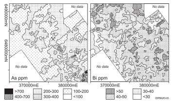
Figure 3. Contoured plots of gridded As and Bi fine fraction (<200 µm) soil data, using a partial dilute HCl digest, showing depletion haloes.
