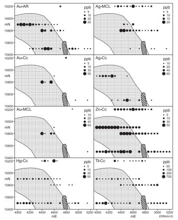
Figure 5. Circle plots of magnetic lag samples analysed for Au and Ag after Aqua regia (AR), Conc. HCl (Cc) and Micro cyanide leach (MCL) digests on orientation traverses N of the McKinnons Au Mine. The IP chargeability anomaly is the stippled area, the Au mineralization intercept is the cross-hatched zone and potential lode Au trends outlined.
