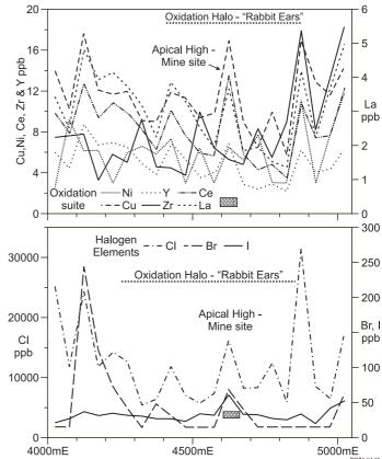
Figure 4. Plots of Enzyme Leach® oxidation suite in fine fraction soil samples on Traverse 15500N showing that apical high values correspond with the Au intercept at depth (shaded box) occurring within a broad chargeability anomaly outlined by distinctive 'rabbit ears' anomalies for most of the elements.
