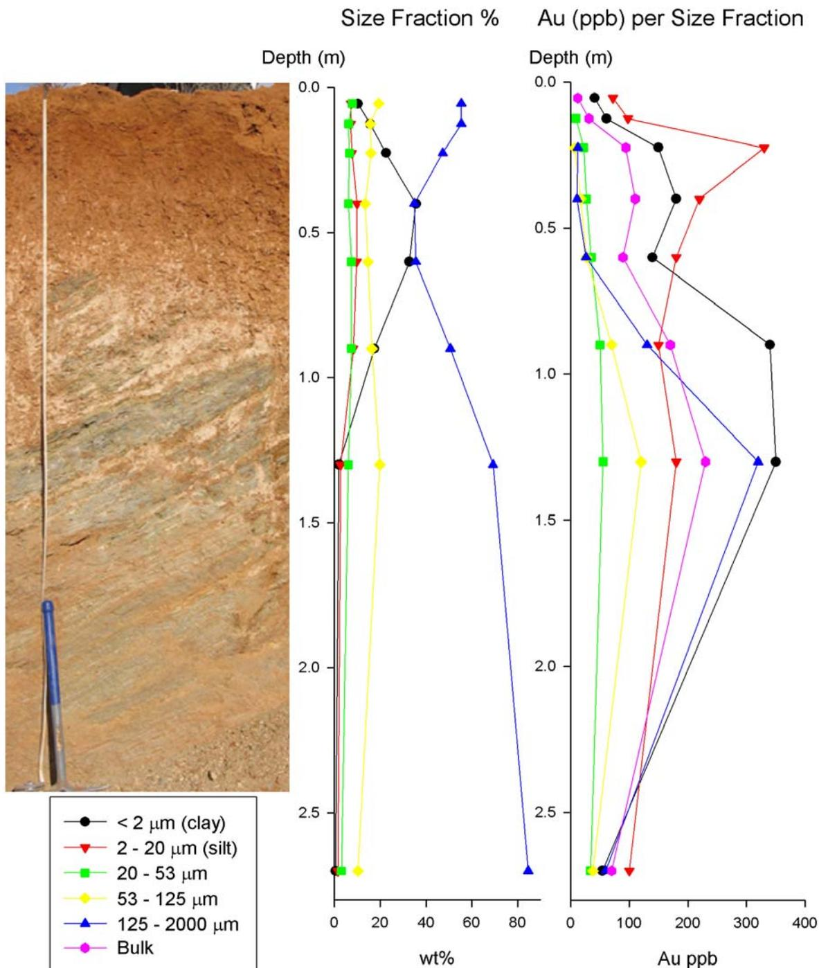
**Figure 24. Profile 2 – costean located just off the main zone of mineralisation (Dart et al., 2006).** See Figure 22 for geographic location.
