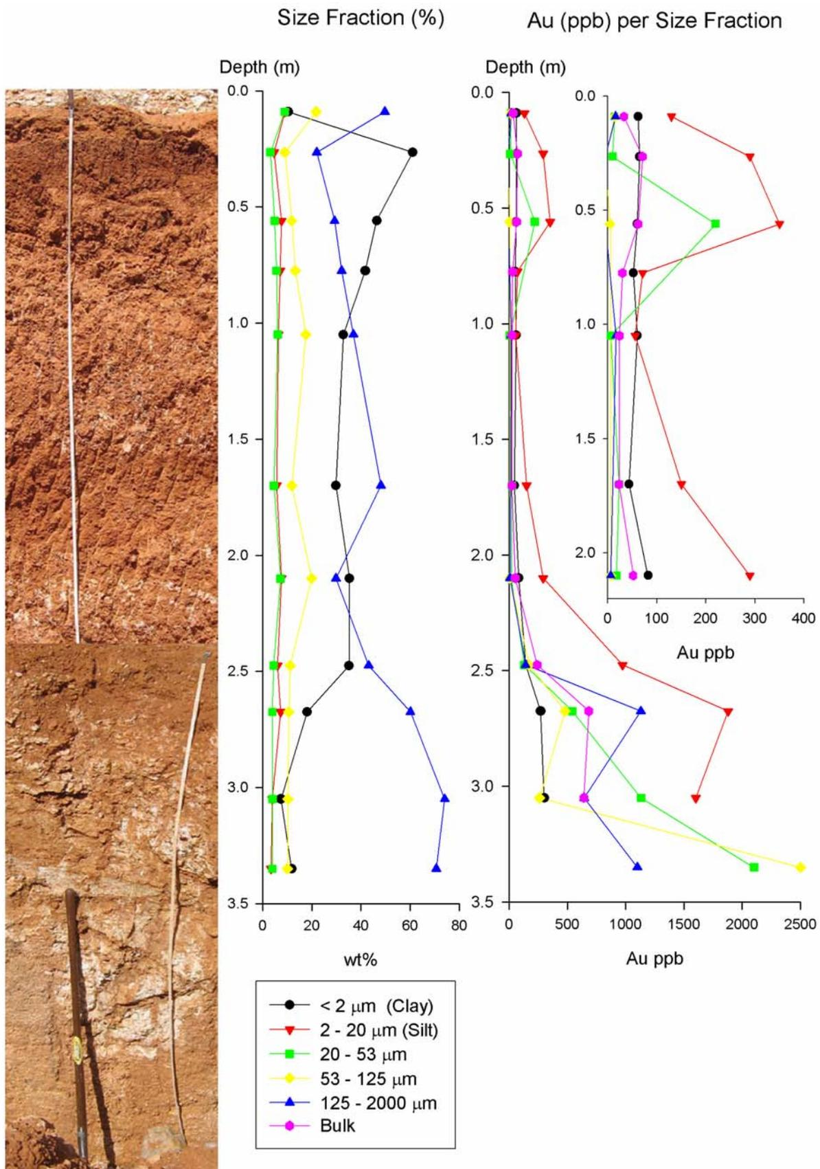
**Figure 23. Profile 1 – costean located directly over mineralisation (Dart et al., 2006). See Figure 22 for geographic location.**
