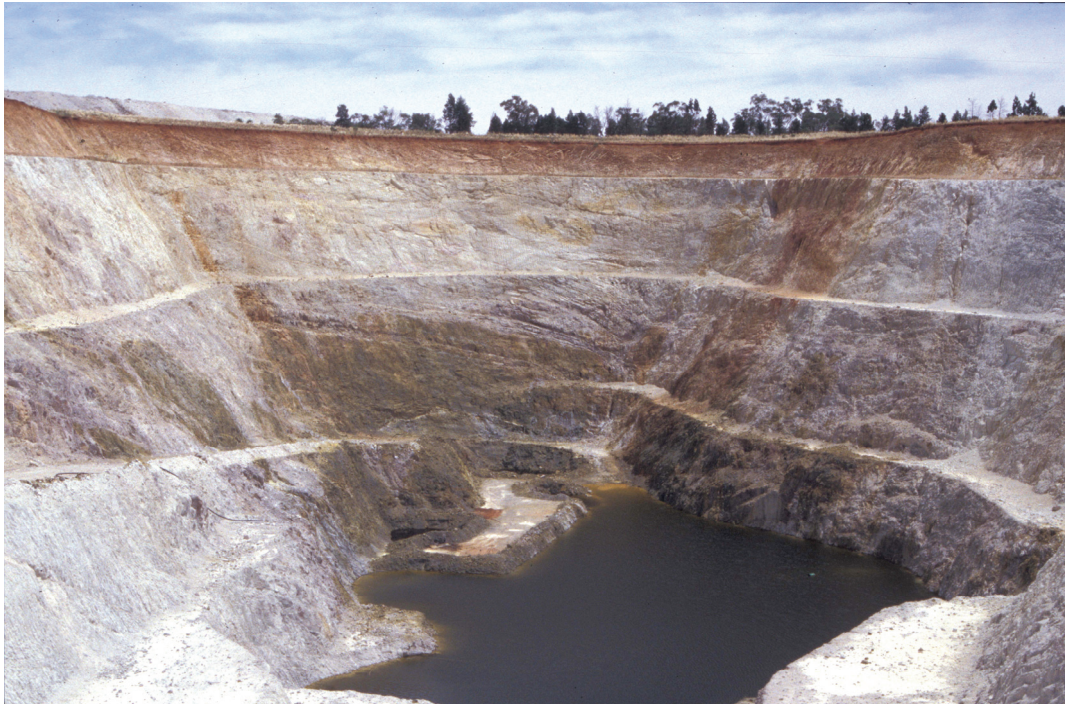
Figure 16.2. View to north-west end of McKinnons Pit showing remnant pyritic mineralisation in the base of the pit and blocks of ferruginous material after low-grade mineralisation within the saprolite/saprock. Also visible is bedding and some cross-cutting and ferruginised fault zones (photo Ken McQueen).
