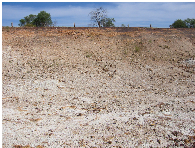
Figure 15.1. View of quarry showing upper zone of weakly ferruginised and laminated calcrete hard pan overlying mottled saprolite.
