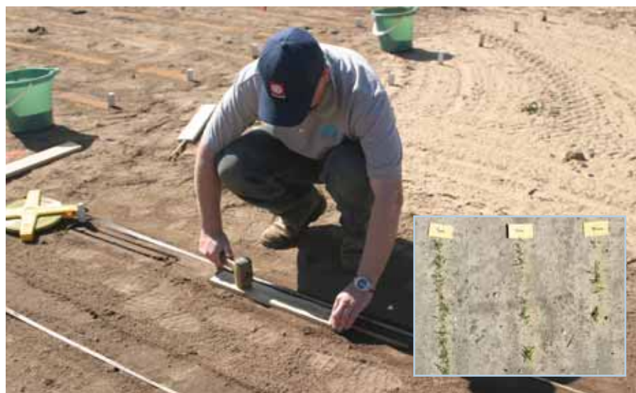
Depth was precisely controlled by a wooden dowel. INSET: Plots displaying superior germination of panic seedlings when sown (from the left) at 5 mm, 15 mm and 30 mm depths
