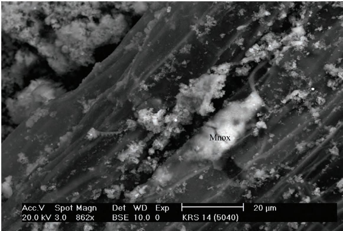
Figure 3.27. Iodine-bearing Mn oxide (Mnox) on organic matter and associated with minor disseminated pyrite. Sample KRS14, mound springs at Wheal Ellen. Back-scattered electron image (SEM).
