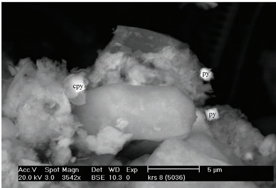
Figure 3.26. Disseminated subhedral to euhedral chalcopyrite (cpy) and pyrite (py) grains on quartz and kaolin. Sample KRS8. Back-scattered electron image (SEM).
