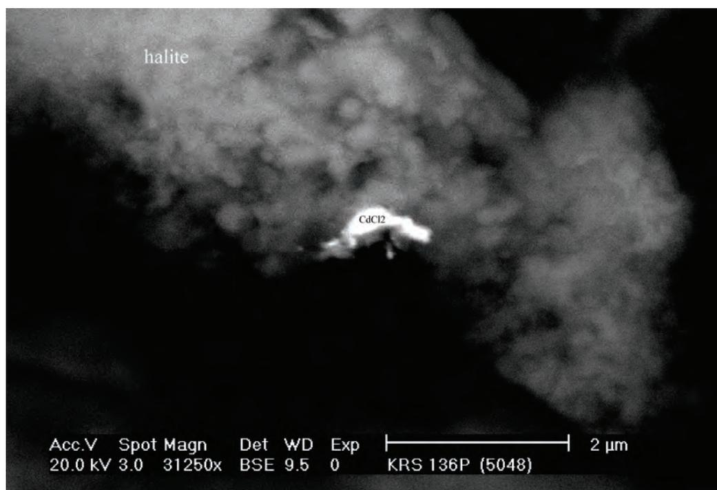
Figure 3.7. An anhedronal grain of CdCl<sub>2</sub> (CdCl<sub>2</sub>) associated with halite from a ferrihydrite precipitate from a narrow gully high on the side of a hill, near Charleston Conservation Park. Sample KRS136P. Back-scattered electron image (SEM).
