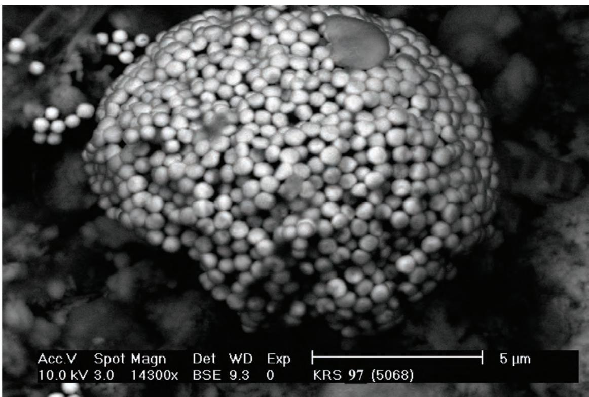
Figure 3.14. Pyrite framboid, with minor organic coatings, formed of rounded grains. Sample KRS97. Back-scattered electron image (SEM).
