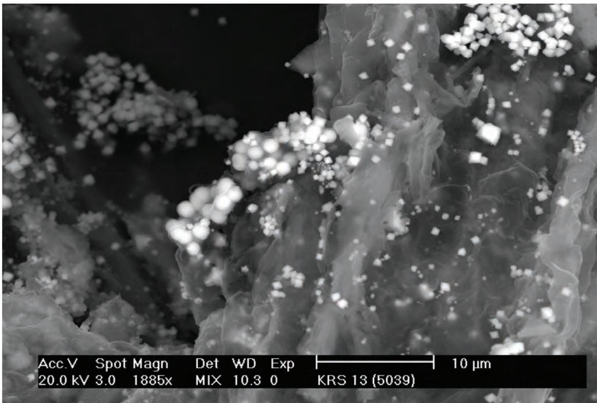
Figure 3.20. Aggregates of spherical sphalerite grains (centre) and pyrite cubes (top right) on organic matter. Sample KRS13, mound springs at Wheal Ellen. Back-scattered electron image (SEM).
