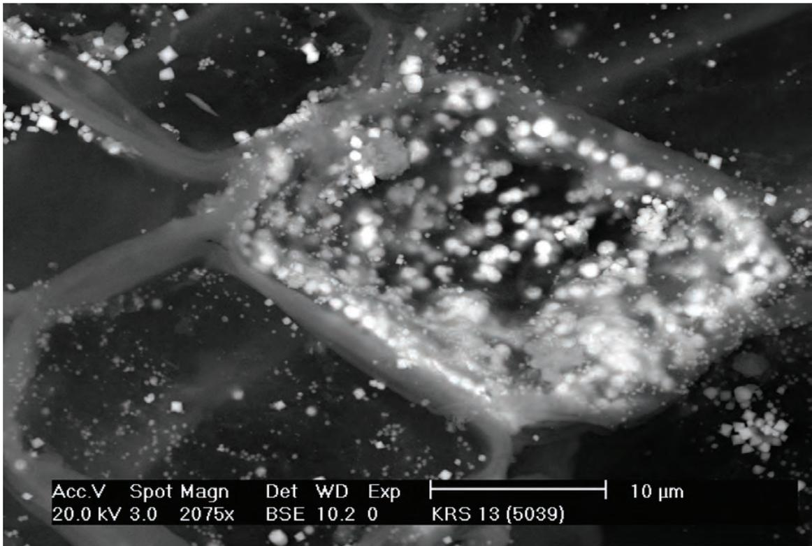
Figure 3.21. Spherical sphalerite grains lining plant cell walls. Sample KRS13, mound springs at Wheal Ellen. Back-scattered electron image (SEM).
