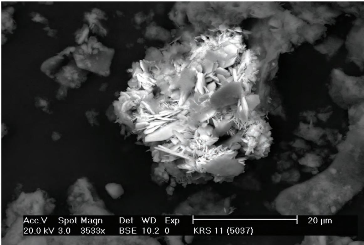
Figure 3.29. Aggregate of barite platelets associated with quartz and kaolin. Sample KRS11, Glenalbyn mine. Back-scattered electron image (SEM).
