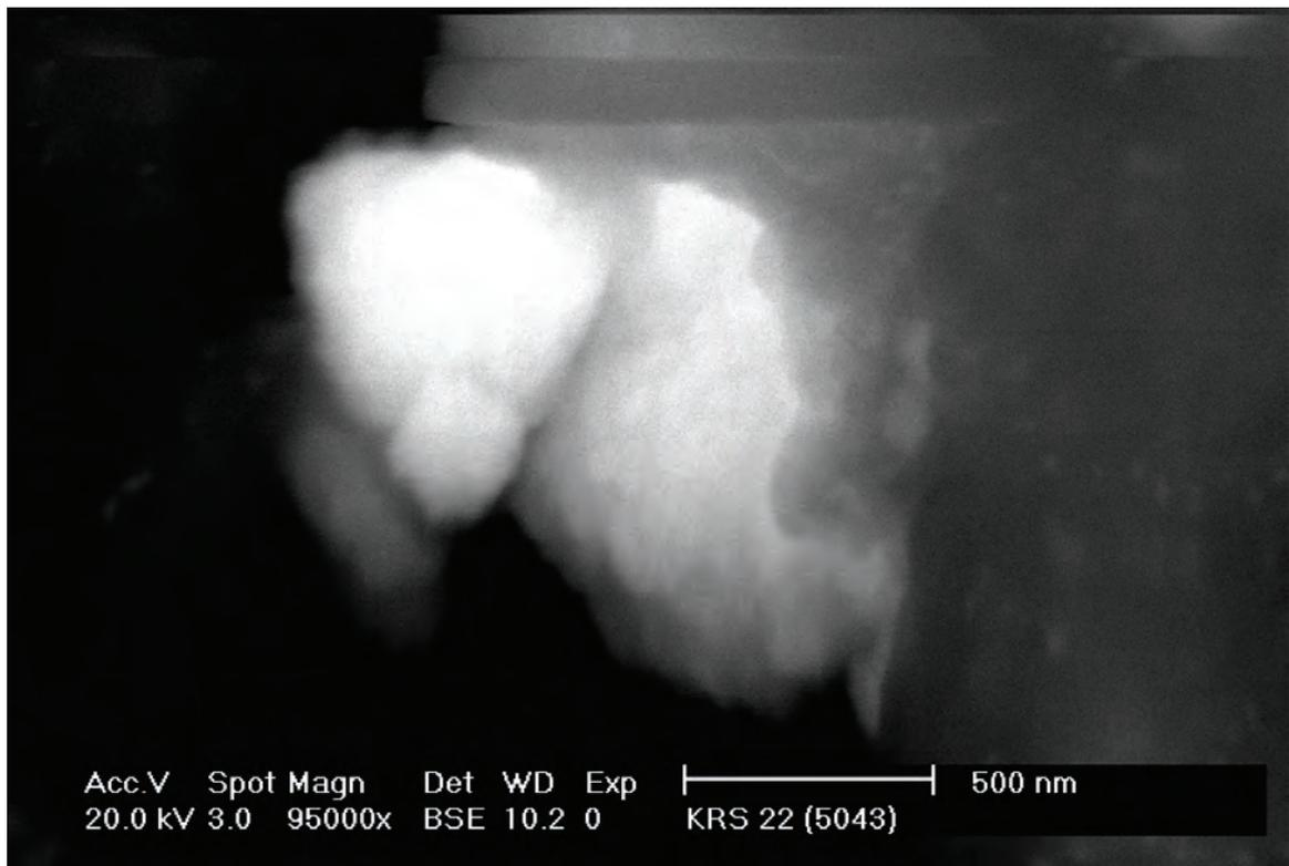
Figure 3.25. Aggregate of globular to botryoidal galena grains embedded in mica. Sample KRS22. Back-scattered electron image (SEM).
