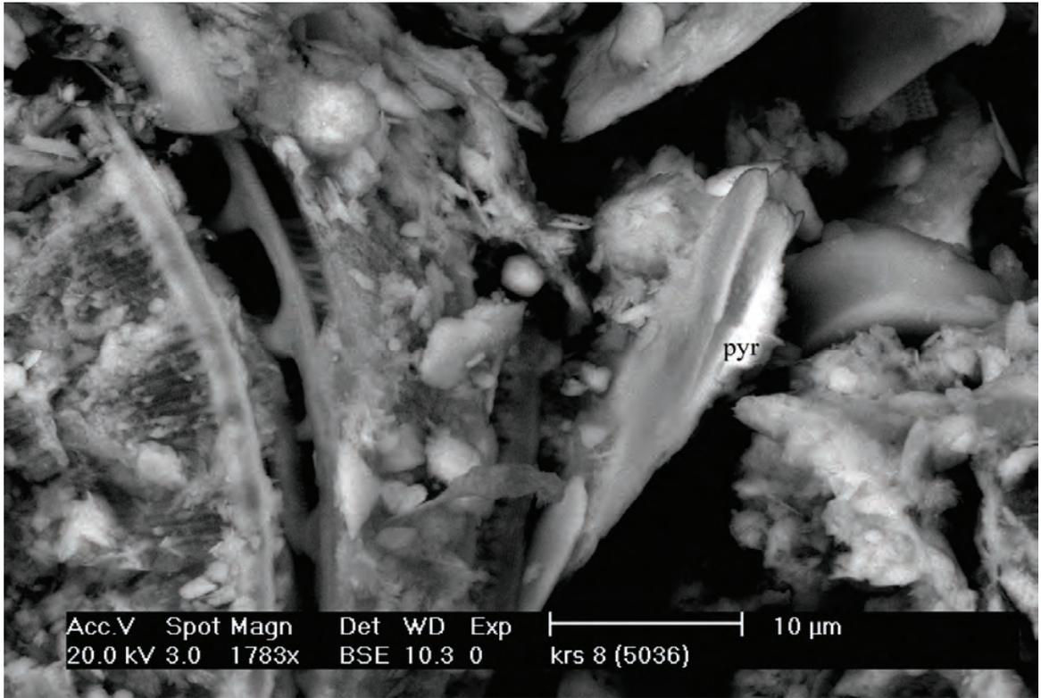
Figure 3.15. Partial pyrite (pyr) coating on organic matter. Sample KRS8. Back-scattered electron image (SEM).
