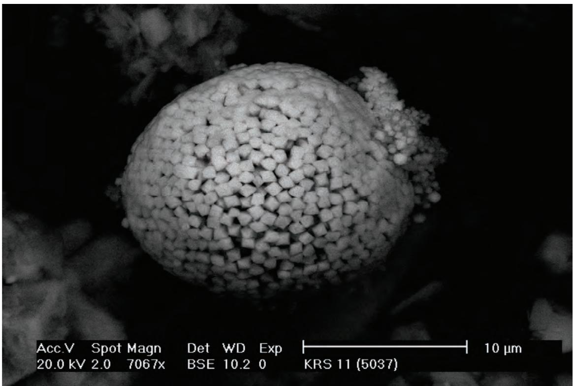
Figure 3.12. Pyrite framboid composed of cubes. Sample KRS11, Glenalbyn mine. Back-scattered electron image (SEM).
