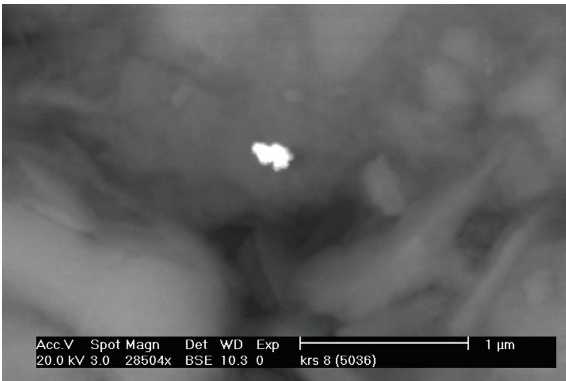
Figure 3.28. Anhedral grain of native gold embedded in kaolin. Sample KRS8. Back-scattered electron image (SEM).
