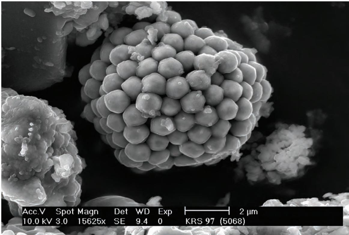
Figure 3.13. Pyrite framboid composed of pyritohedra. Sample KRS97. Back-scattered electron image (SEM).
