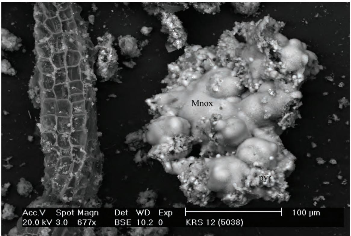
Figure 3.16. Pyrite (pyr) aggregates encrusting a botryoidal aggregate of cobaltian Mn oxides (Mnox) associated with plant material. Sample KRS12, mound springs at Wheal Ellen. Back-scattered electron image (SEM).
