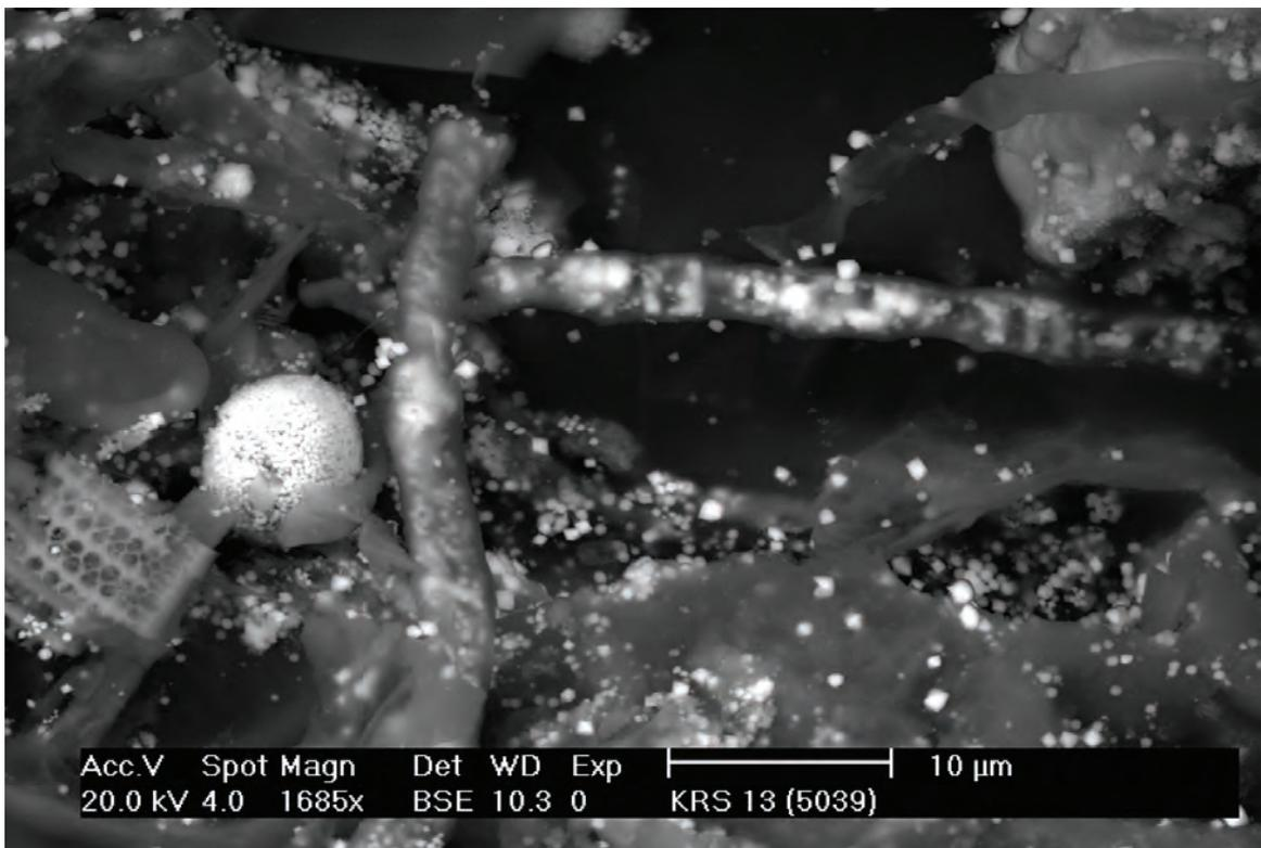
Figure 3.10. Pyrite framboid associated with a diatom fragment. The rootlets contain anhedronal sphalerite grains. Sample KRS13, mound springs at Wheal Ellen. Back-scattered electron image (SEM).
