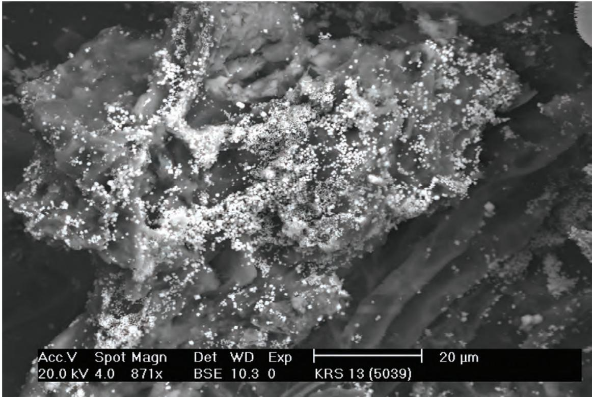
Figure 3.9. Fine-grained, disseminated pyrite grains on organic matter. Sample KRS13, mound springs at Wheal Ellen. Back-scattered electron image (SEM).
