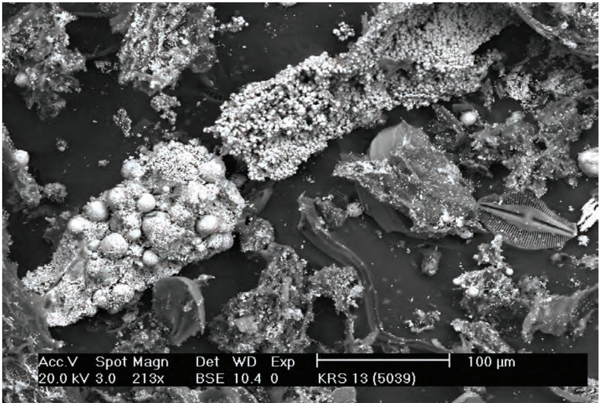
Figure 3.11. Aggregates of pyrite framboids and individual grains encrusting a rootlet. Individual framboids, disseminated pyrite cubes and rare diatoms occur in the matrix. Sample KRS13, mound springs, Wheal Ellen. Back-scattered electron image (SEM).
