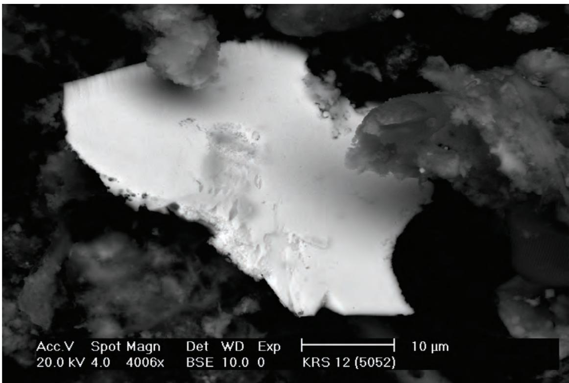
Figure 3.30. Anhedral barite platelet, associated with quartz and kaolin, with dissolution pits. Sample KRS12, mound springs at Wheal Ellen. Back-scattered electron image (SEM).
