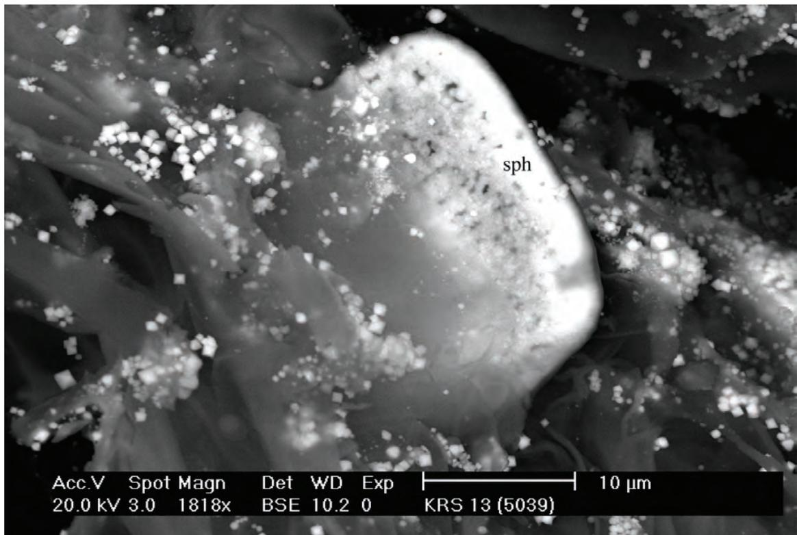
Figure 3.23. Rounded sphalerite (sph) grain embedded in organic matter and dusted by fine pyrite cubes. Sample KRS13, mound springs at Wheal Ellen. Back-scattered electron image (SEM).
