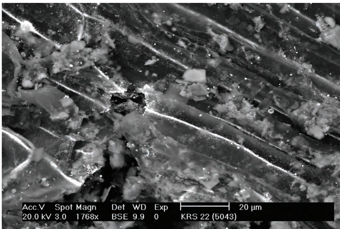
Figure 3.24. Very fine-grained linear aggregates of sphalerite, galena and pyrite precipitated between plant cell walls. Sample KRS22. Back-scattered electron image (SEM).
