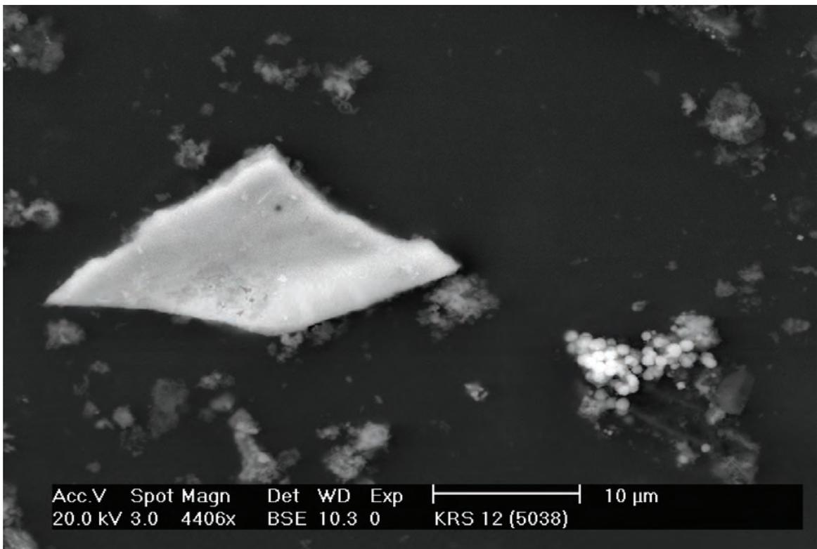
Figure 3.22. Sphalerite flake, with dissolution pits, associated with aggregates of spherical sphalerite grains (at right). Sample KRS12, mound springs at Wheal Ellen. Back-scattered electron image (SEM).
