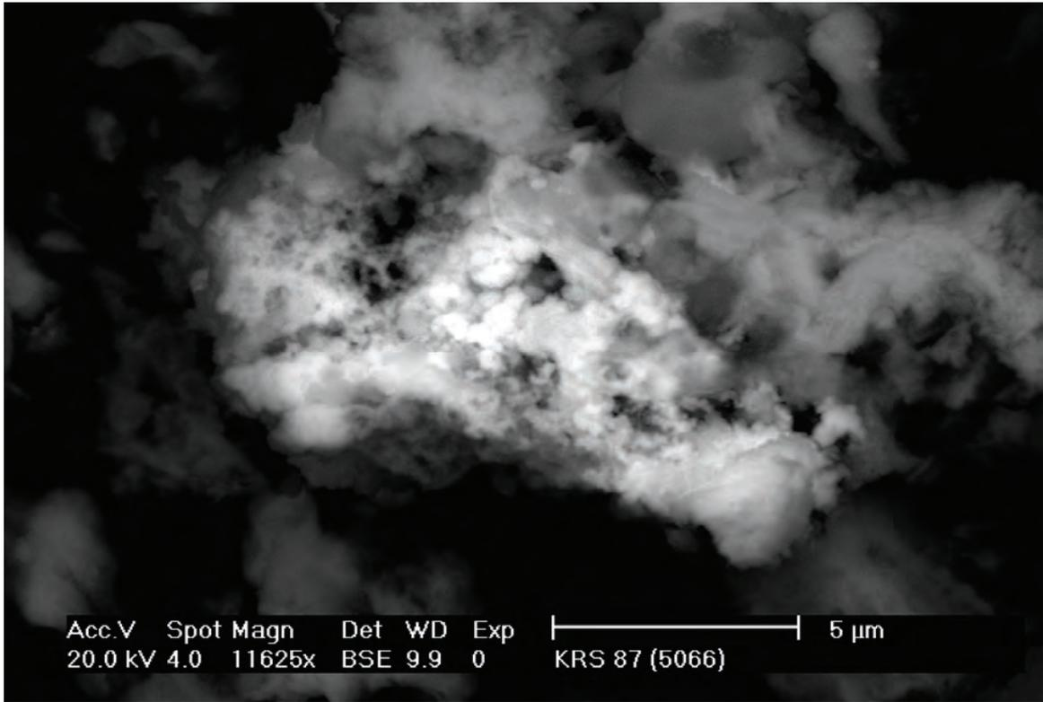
Figure 3.18. Aggregate of anhedral Fe monosulfide grains associated with kaolin and minor calcite. Sample KRS87. Back-scattered electron image (SEM).
