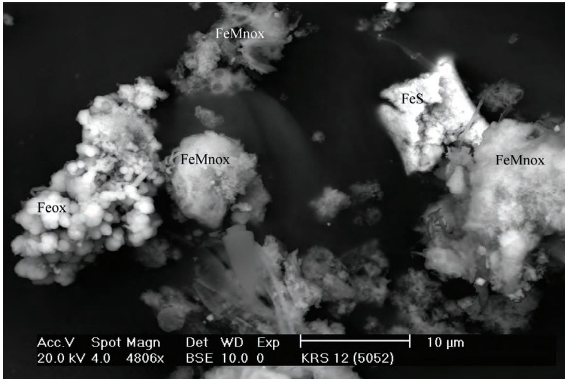
Figure 3.17. Subhedral grain of Fe monosulfide (FeS) associated with Fe-Mn oxide aggregates (FeMnox) and Fe oxides (Feox). Sample KRS12, mound springs at Wheal Ellen. Back-scattered electron image (SEM).
