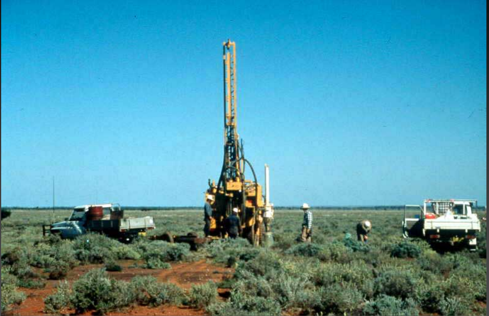
Drilling through regolith near Galena Hill, Broken Hill
