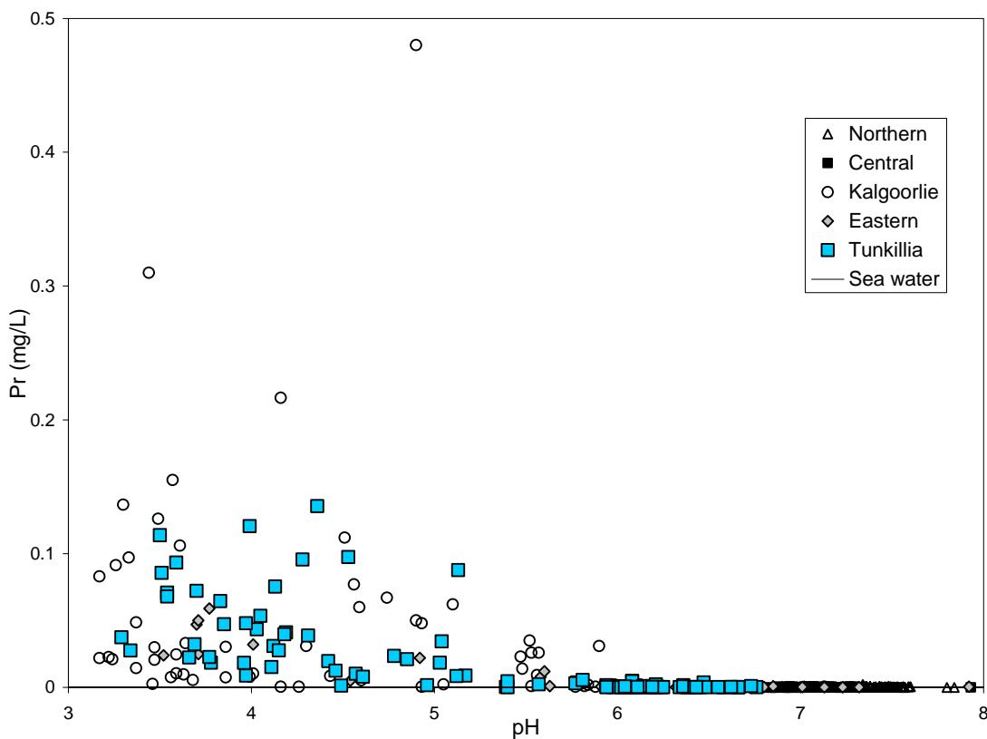
Figure A2.38: Pr vs. pH for groundwaters from Tunkillia and Western Australia.
