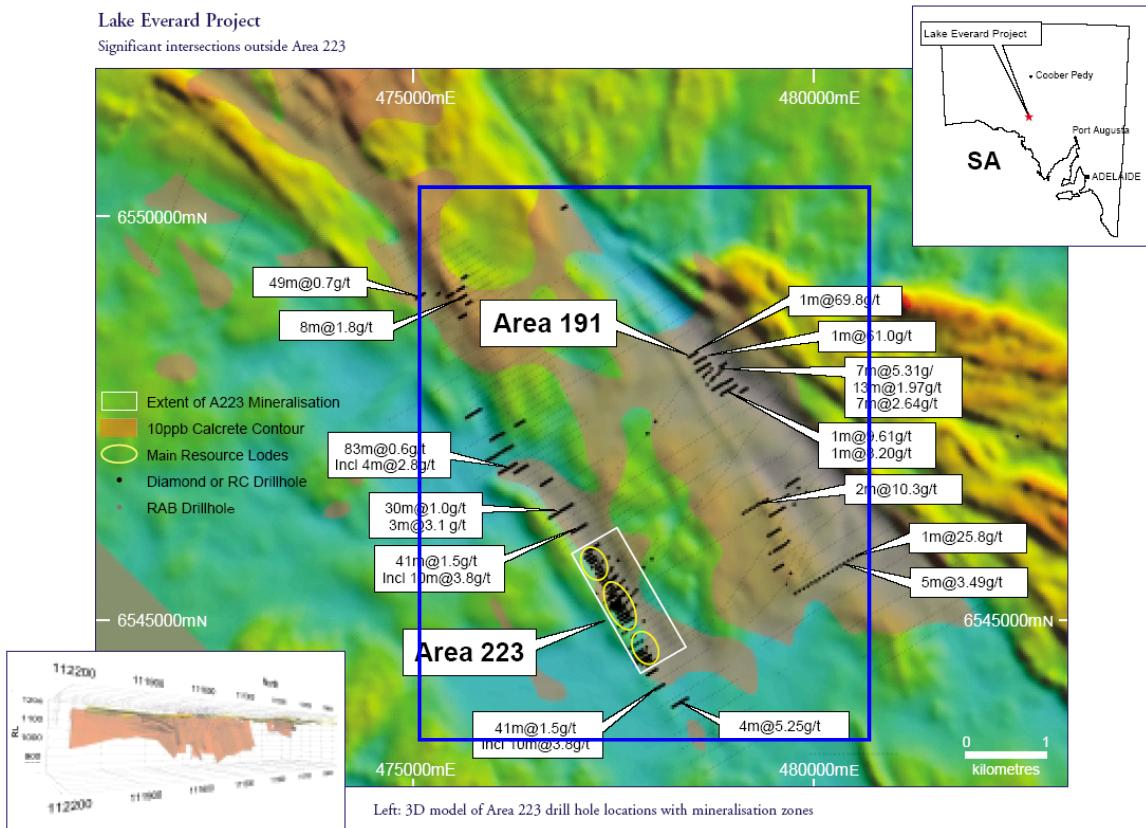
Figure 2: Drilling, calcrete Au and mineralisation for Area 223 (from Anon, 2003). The blue box represents the hydrogeochemical sampling area (Figure 4).
