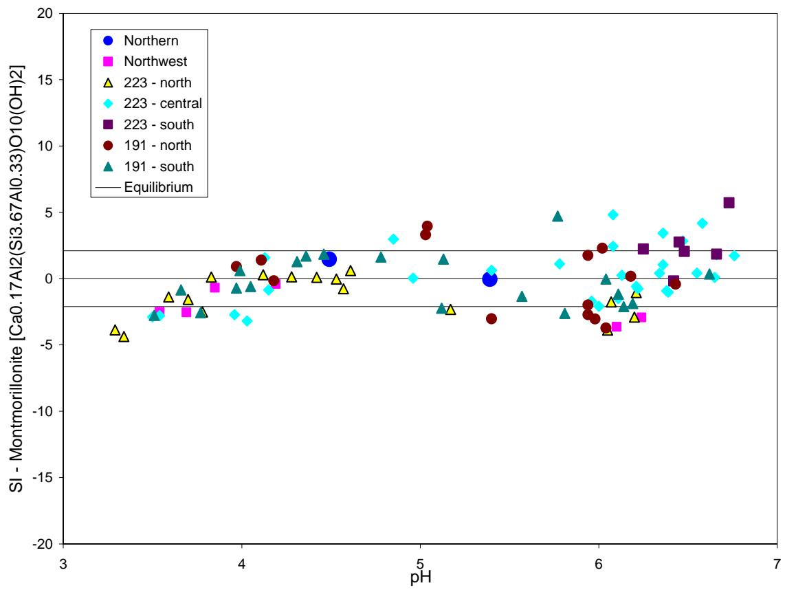
Figure A3.37: SI for montmorillonite for groundwaters from various areas at Tunkillia.
