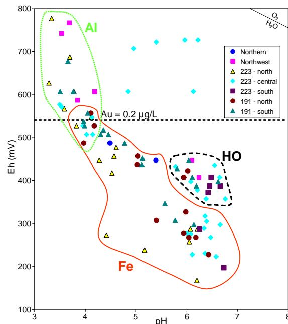
Figure 9: Eh vs pH for Tunkillia groundwaters, differentiated by area (Figure 4). The dashed line is the lower Eh limit at which Au has a solubility of  $0.2 \mu\text{g/L}$  relative to Au metal. Eh/pH controls are discussed in the text.
