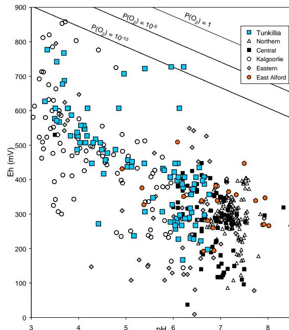
Figure 10: Eh vs pH for Tunkillia and other South and Western Australian groundwaters. In addition to the usual water stability line [ $\text{P}(\text{O}_2)=1$ ], the lines for  $\text{O}_2$  pressures of  $10^{-5}$  and  $10^{-10}$  atm are also shown.
