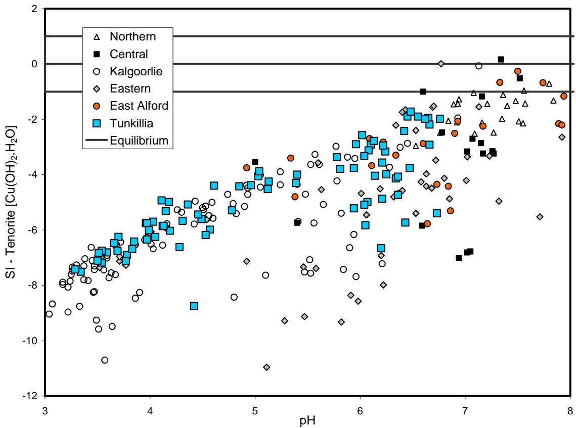
Figure A3.26: SI for tenorite for groundwaters from Tunkillia and Western Australia.
