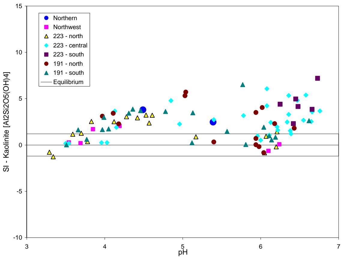
Figure A3.36: SI for kaolinite for groundwaters from various areas at Tunkillia.
