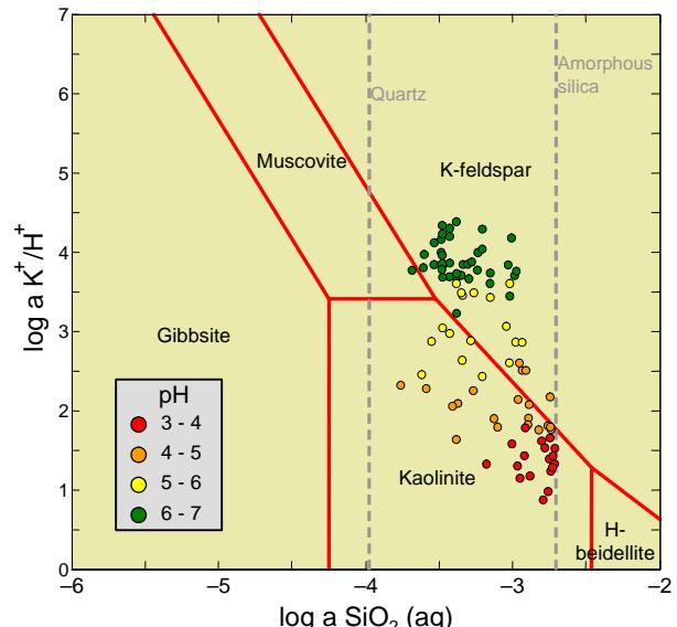
Figure 15: Tunkillia groundwater activity data (from PHREEQE), colour-coded by pH, overlain on a K-Al-Si-H<sub>2</sub>O equilibrium activity diagram (GWB; 25°C / 1 atm). Pyrophyllite suppressed.
