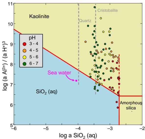
Figure 14: Tunkillia groundwater activity data (from PHREEQE), colour-coded by pH, overlain on a Al-Si-H<sub>2</sub>O equilibrium activity diagram (GWB; 25°C / 1 atm). All SiO<sub>2</sub> phases except amorphous silica suppressed.
