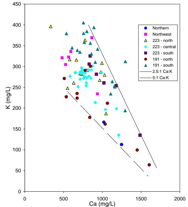
Figure 8: Dissolved K vs Ca at Tunkillia, differentiated by area (Figure 4). The four lowest and three highest salinity waters are removed for clarity.
