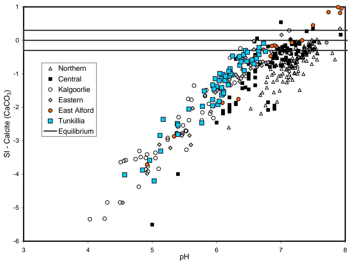
Figure A3.4: SI for calcite for groundwaters from Tunkillia and Western Australia.
