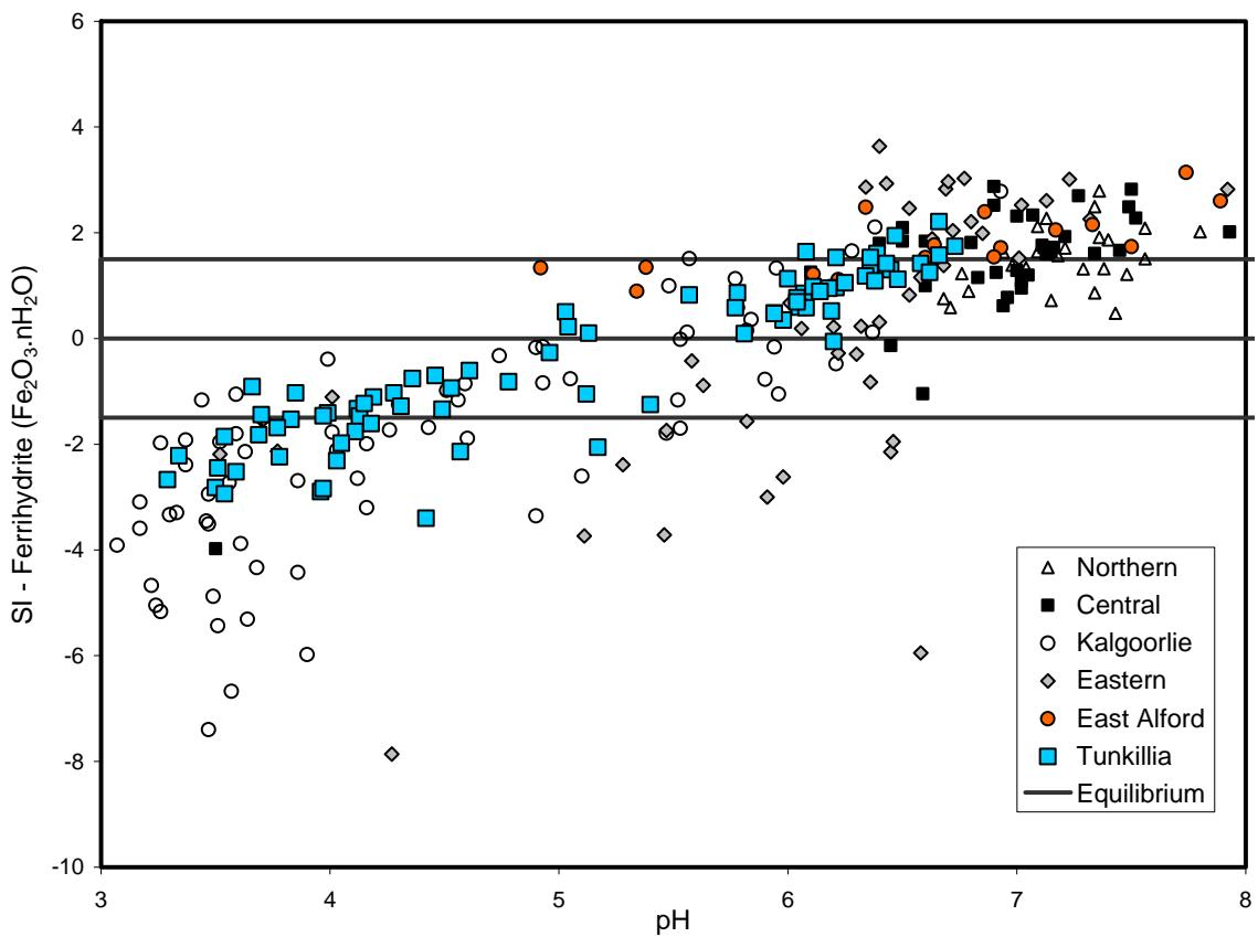
Figure A3.19: SI for ferrihydrite for groundwaters from Tunkillia and Western Australia.
