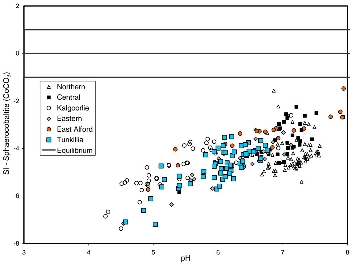
Figure A3.25: SI for sphaerocobaltite for groundwaters from Tunkillia and Western Australia.
