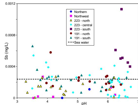
Figure 37: Dissolved Sb vs pH at Tunkillia, differentiated by area (Figure 4).
