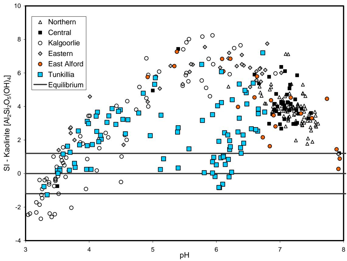
Figure A3.21: SI for kaolinite for groundwaters from Tunkillia and Western Australia.
