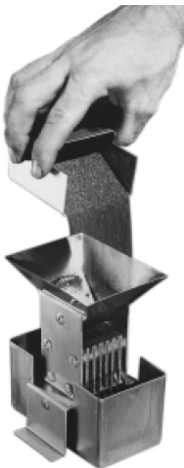
Figure 17. Jones-type Sepor™ precision riffle splitter used to mass reduce the samples for various geochemical analyses.
