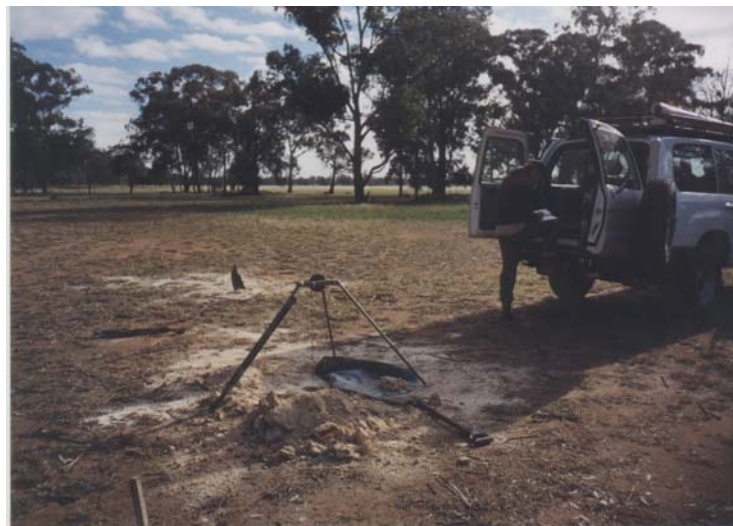
Figure 3. Regolith logging with a small, easy-to-use geophysical logging system, mounted in a 4WD vehicle.
