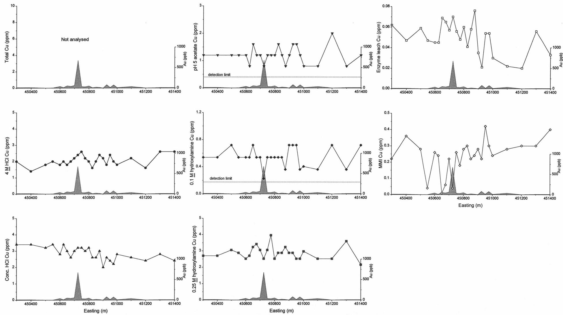
Figure A11.7: Total and extractable Cu from Safari line 6732300N.
