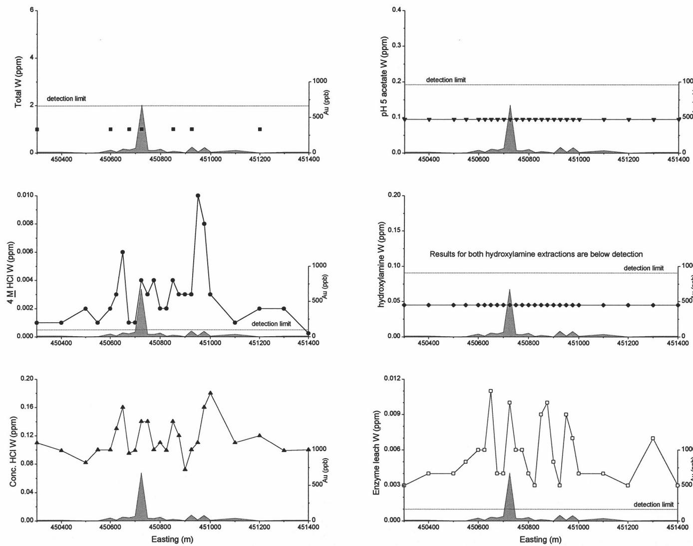
Figure A11.12: Total and extractable W from Safari line 6732300N.
