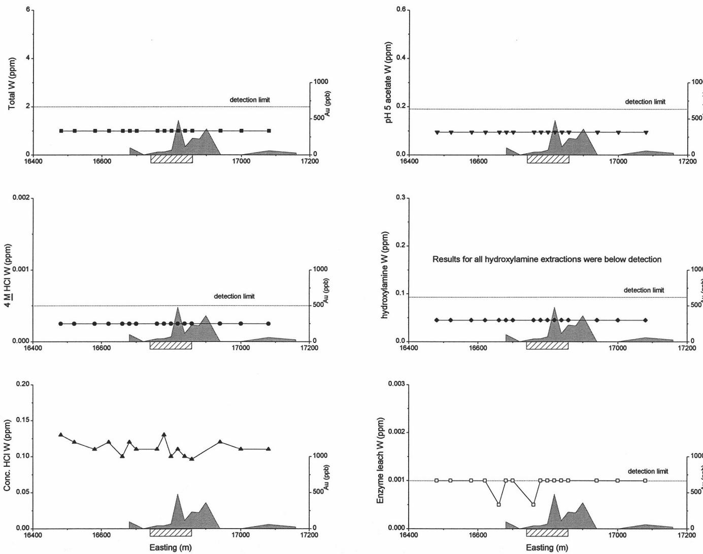
Figure A9.12: Total and extractable W from Bronzewing line 9800N.
