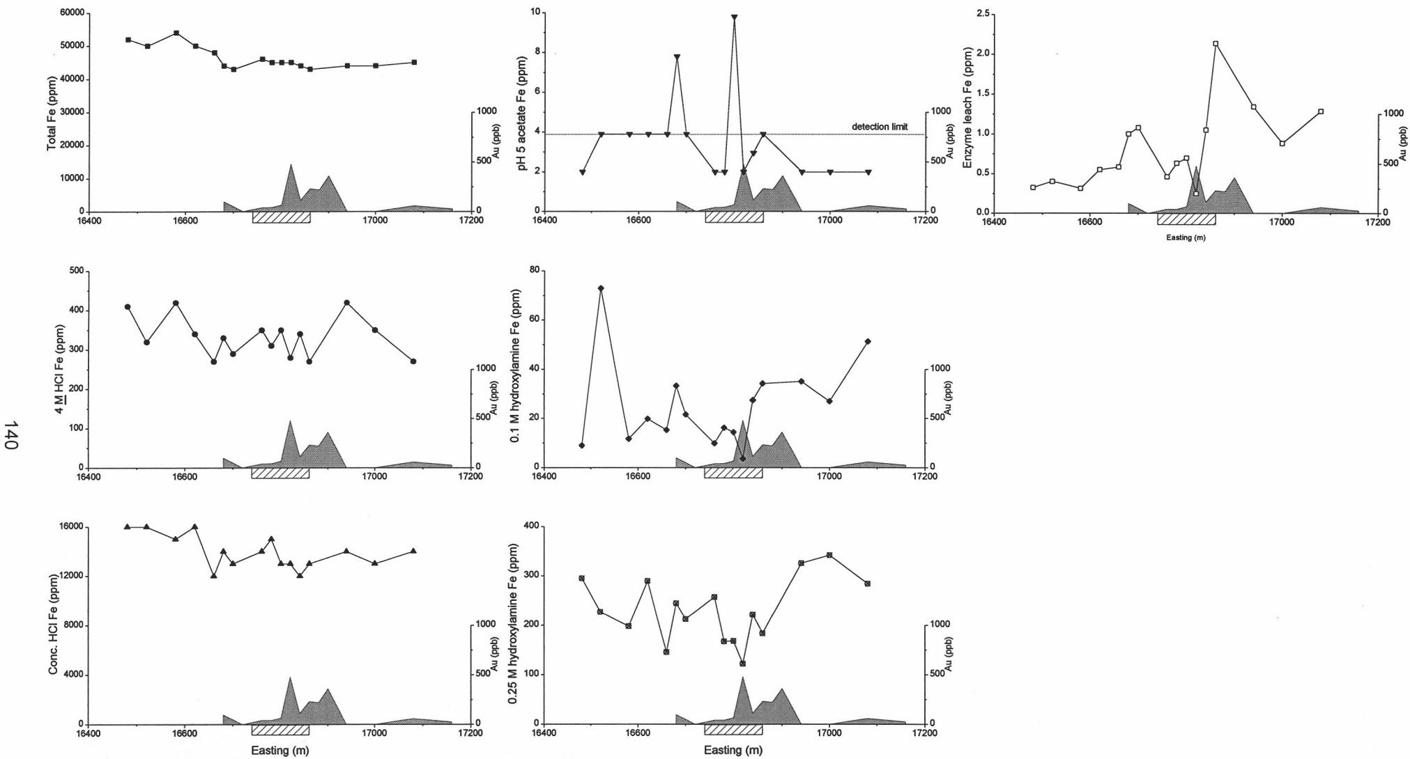
Figure A9.8: Total and extractable Fe from Bronzewing line 9800N.
