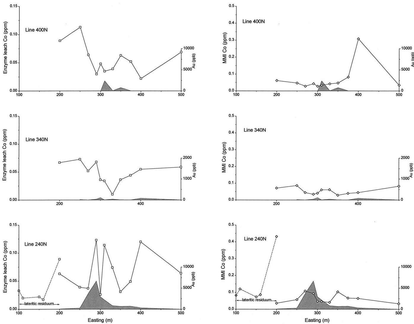
Figure A8.17: Enzyme leach and MMI Co from Fender lines 400, 340 and 240 N.
