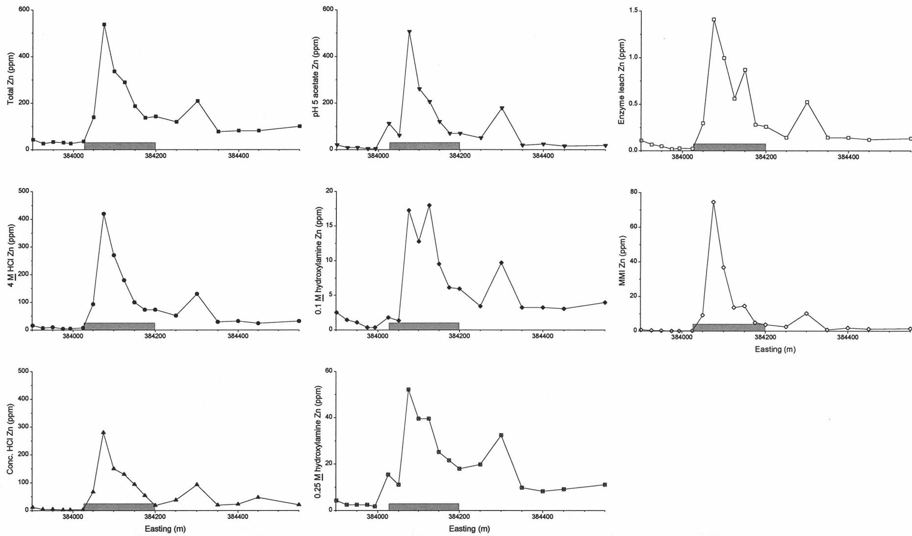
Figure A13.13: Total and extractable Zn from Apollo line 526080N.
