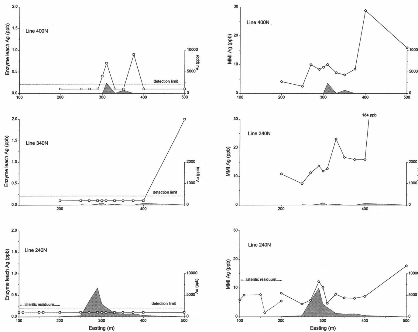
Figure A8.3: Enzyme leach and MMI Ag from Fender lines 400, 340 and 240 N.
