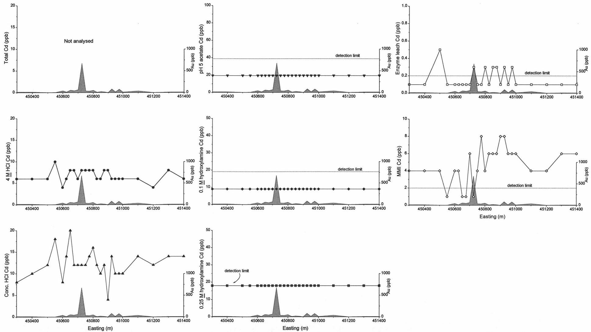
Figure A11.4: Total and extractable Cd from Safari line 6732300N.
