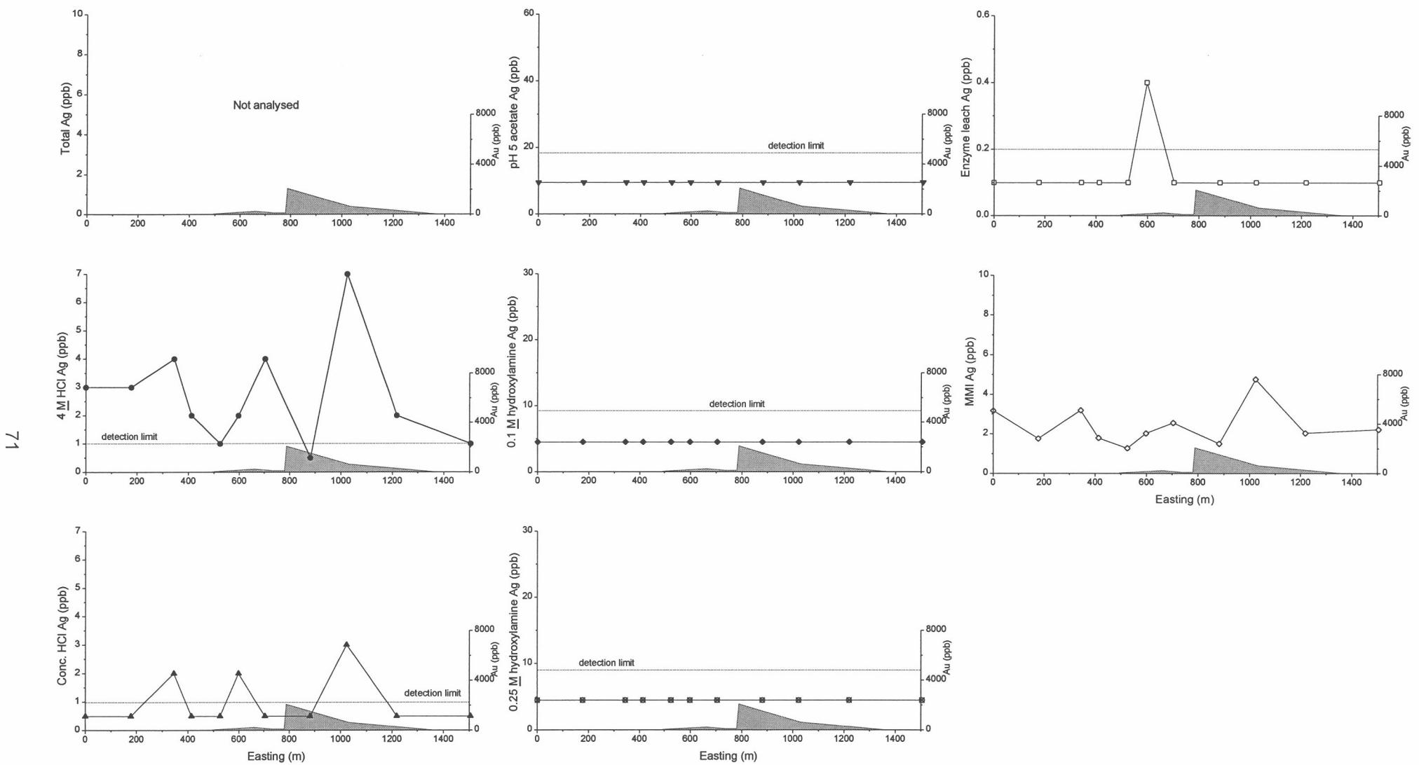
Figure A7.2: Total and extractable Ag from Baxter traverse A.
