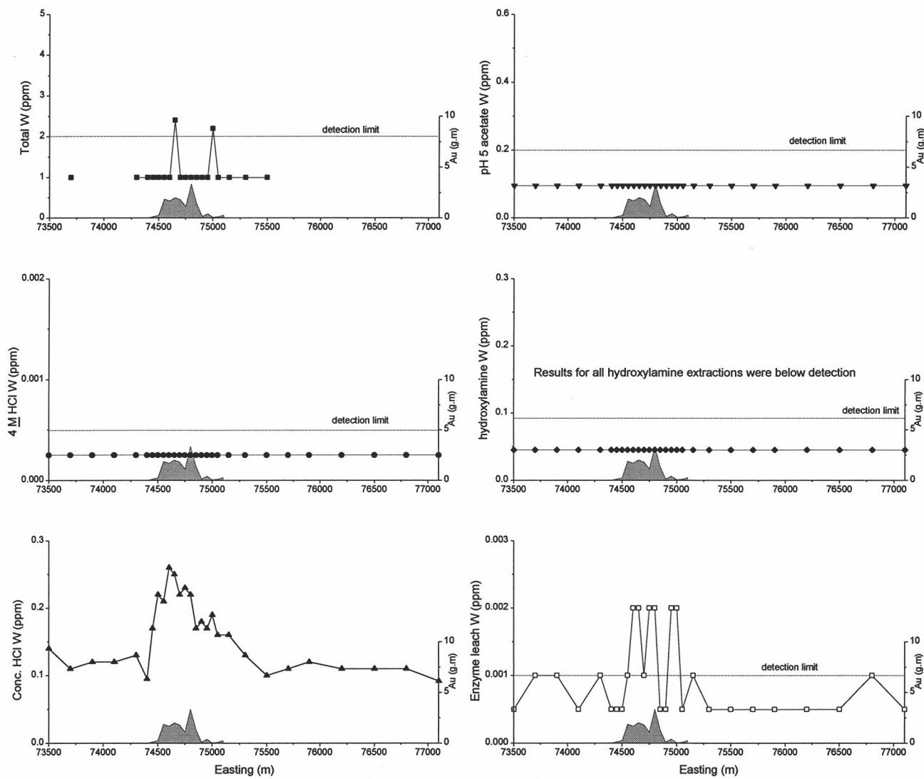
Figure A10.12: Total and extractable W from Curara line 27500N.
