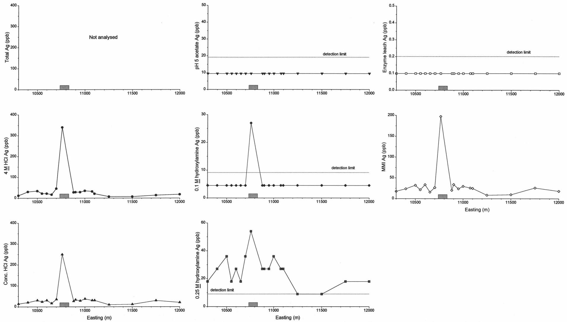
Figure A12.1: Total and extractable Ag from Steinway line 4250N.
