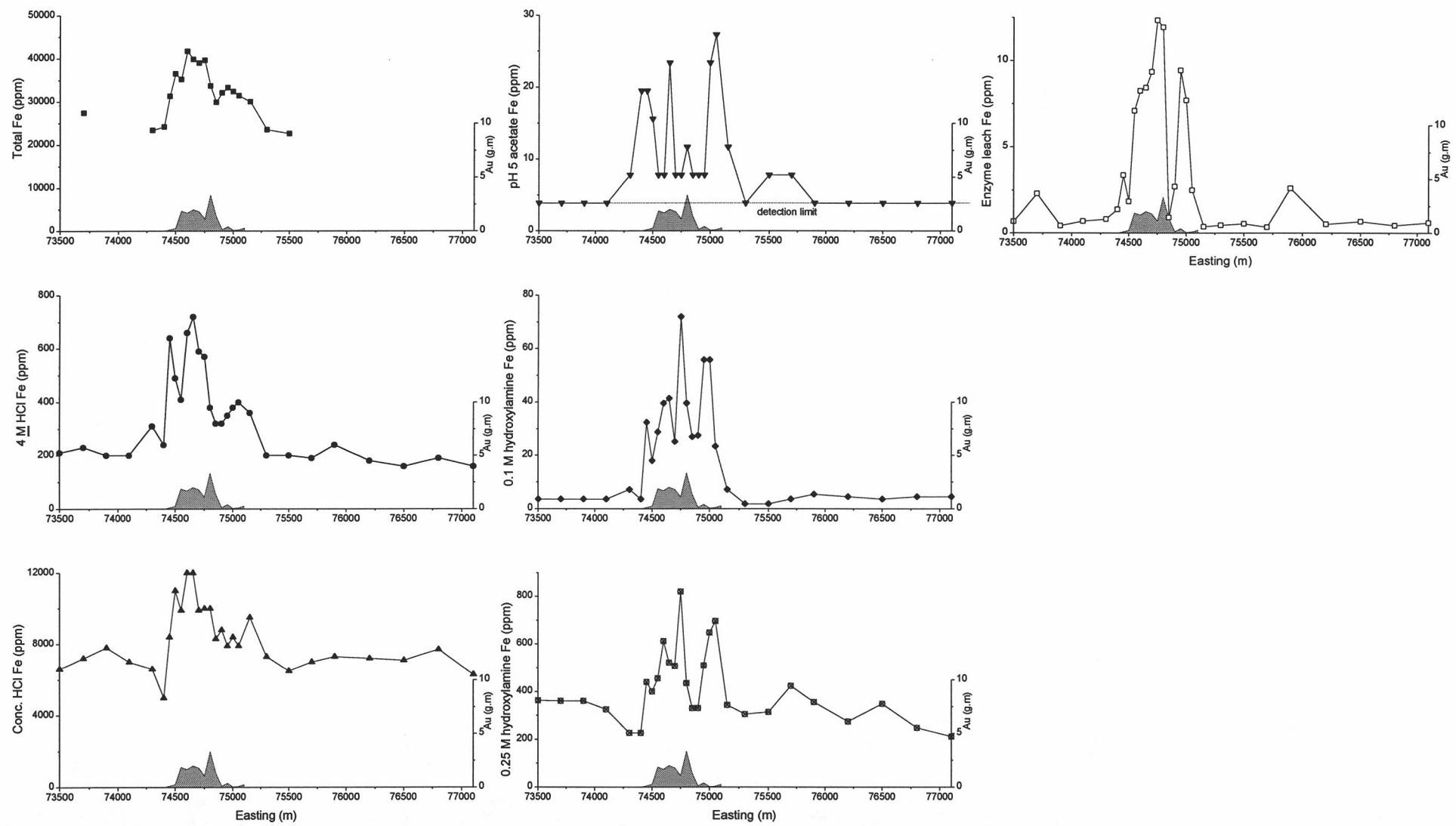
Figure A10.8: Total and extractable Fe from Curara line 27500N.
