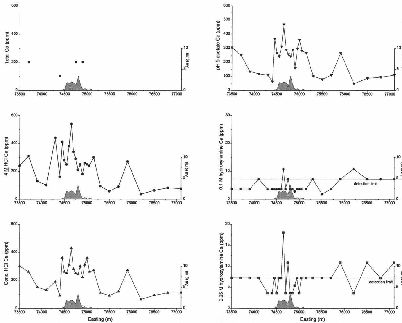
Figure A10.3: Total and extractable Ca from Curara line 27500N.
