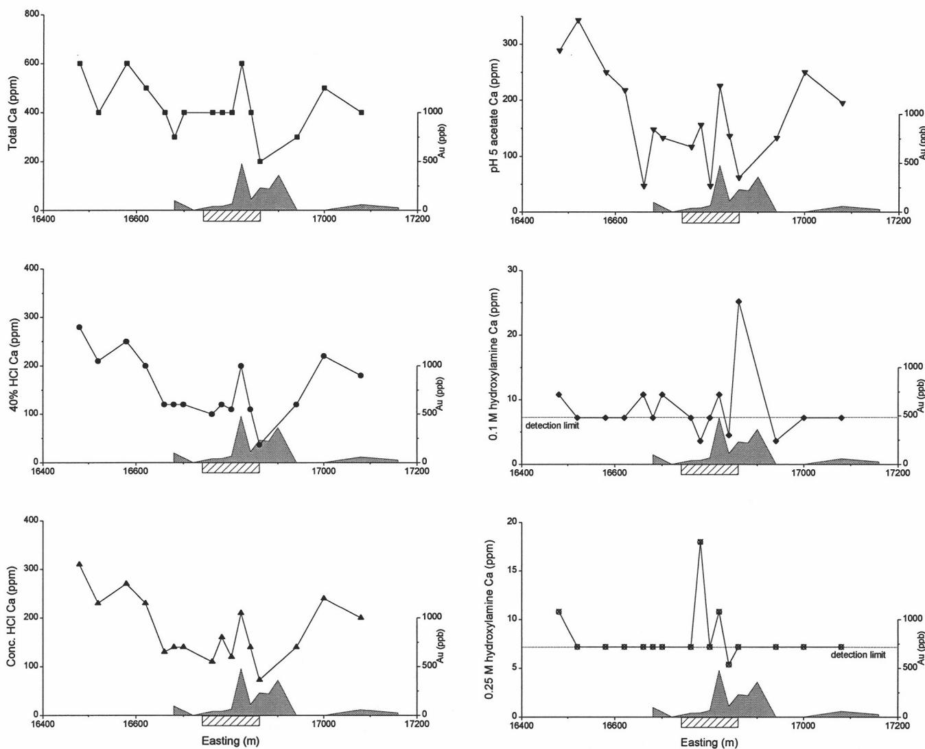
Figure A9.3: Total and extractable Ca from Bronzewing line 9800N.
