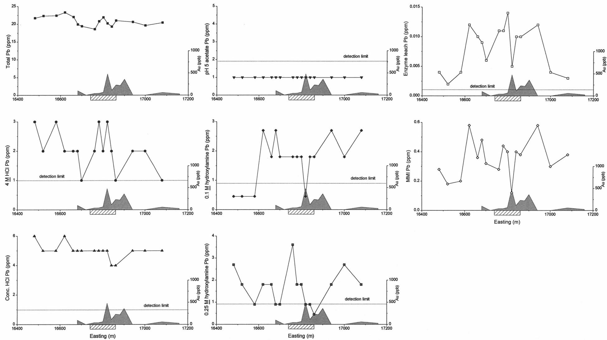
Figure A9.11: Total and extractable Pb from Bronzewing line 9800N.
