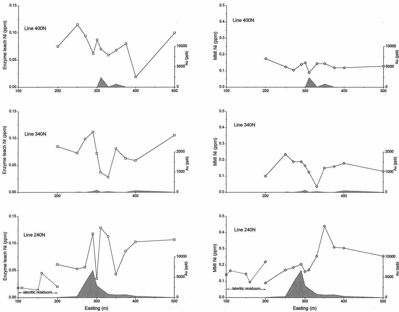
Figure A8.28: Enzyme leach and MMI Ni from Fender lines 400, 340 and 240 N.
