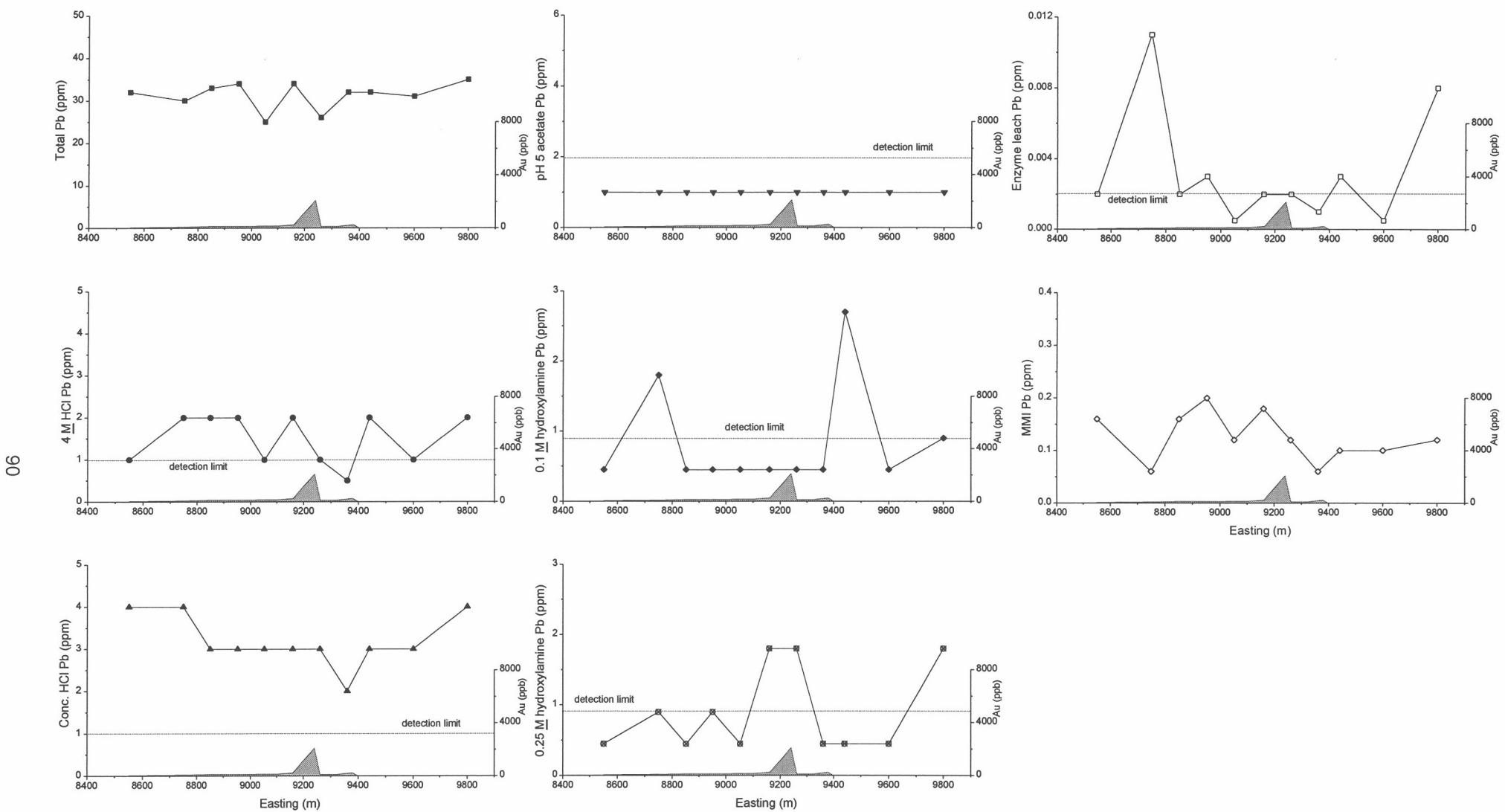
Figure A7.21: Total and extractable Pb from Baxter line 12600N.
