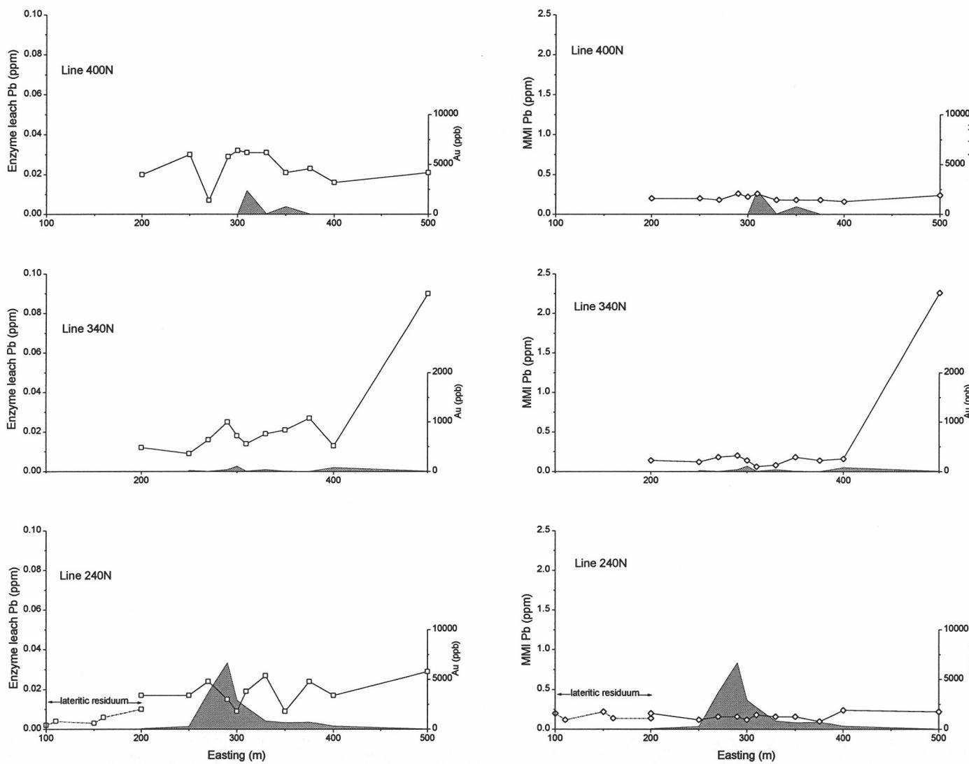
Figure A8.31: Enzyme leach and MMI Pb from Fender lines 400, 340 and 240 N.
