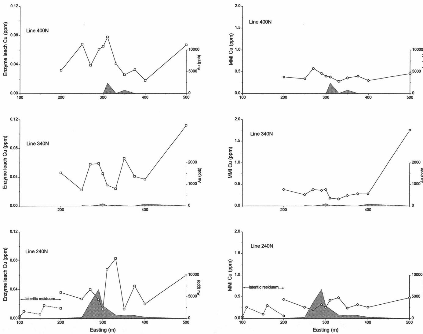
Figure A8.20: Enzyme leach and MMI Cu from Fender lines 400, 340 and 240 N.
