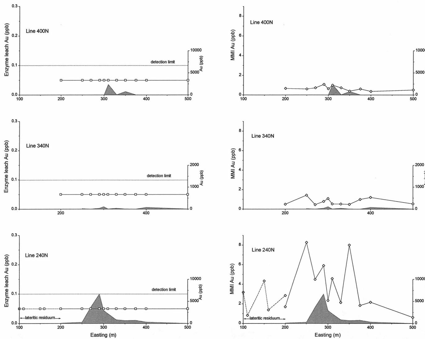
Figure A8.6: Enzyme leach and MMI Au from Fender lines 400, 340 and 240 N.
