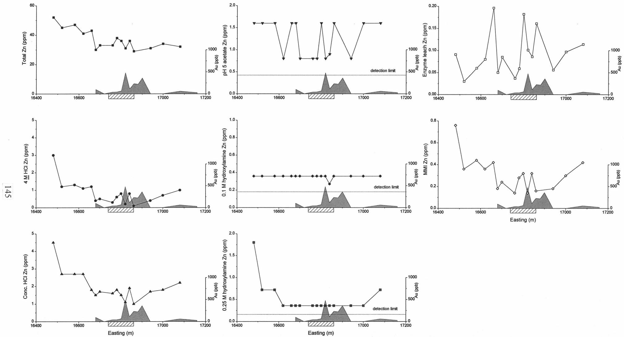
Figure A9.13: Total and extractable Zn from Bronzewing line 9800N.
