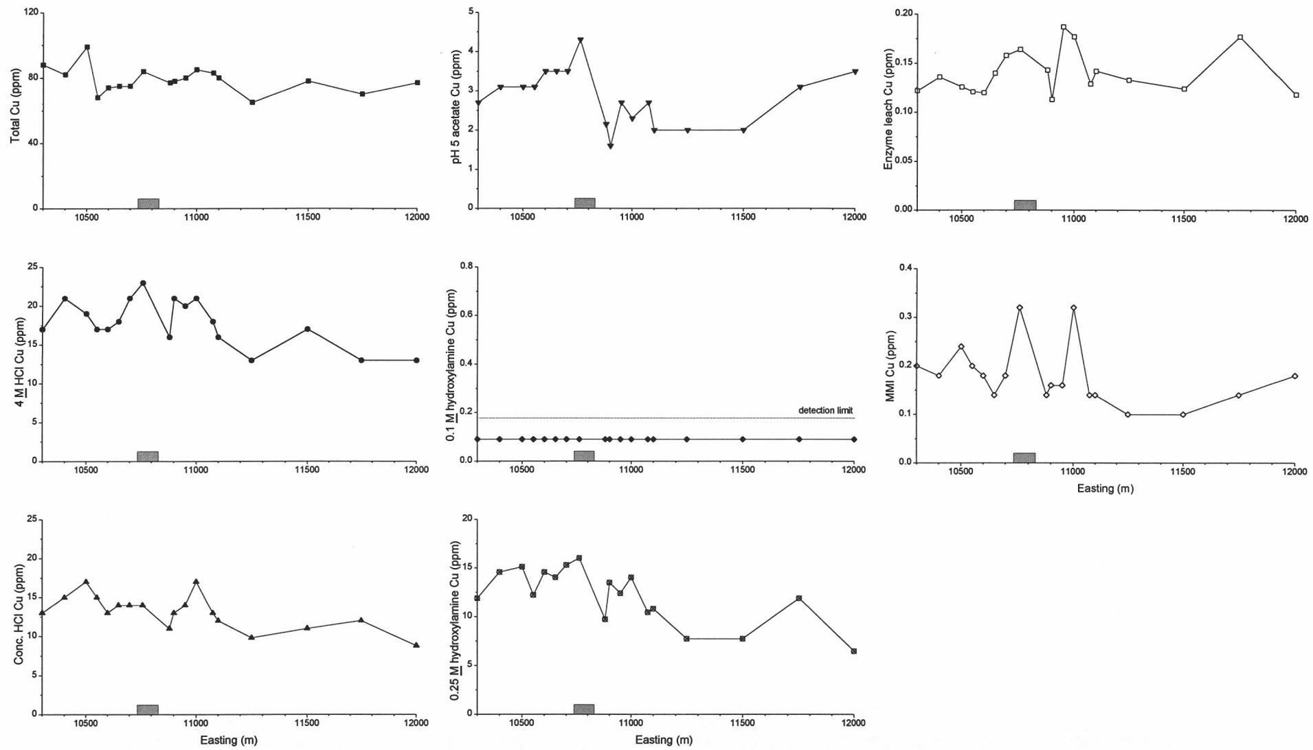
Figure A12.7: Total and extractable Cu from Steinway line 4250N.
