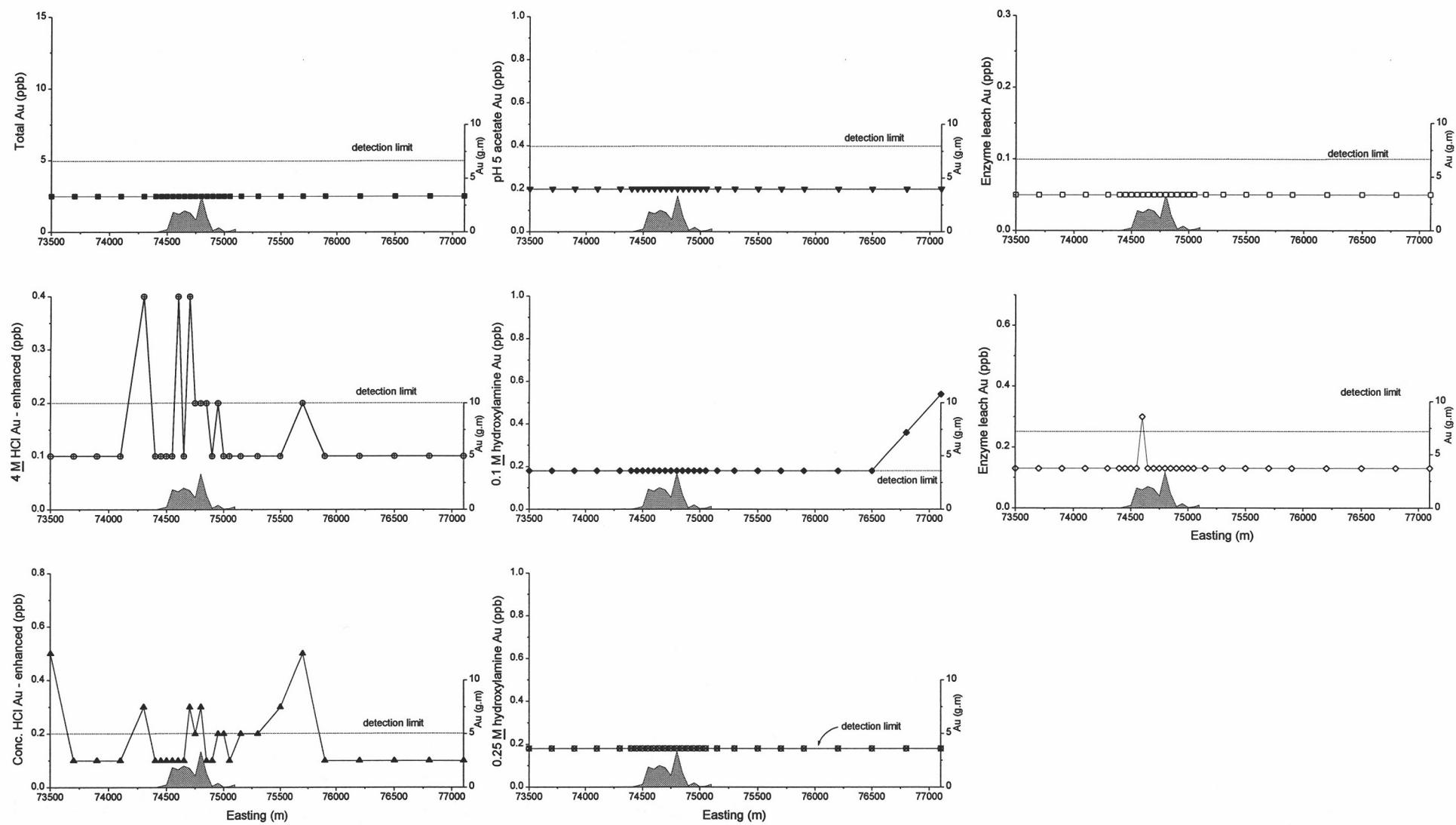
Figure A10.2: Total and extractable Au from Curara line 27500N.
