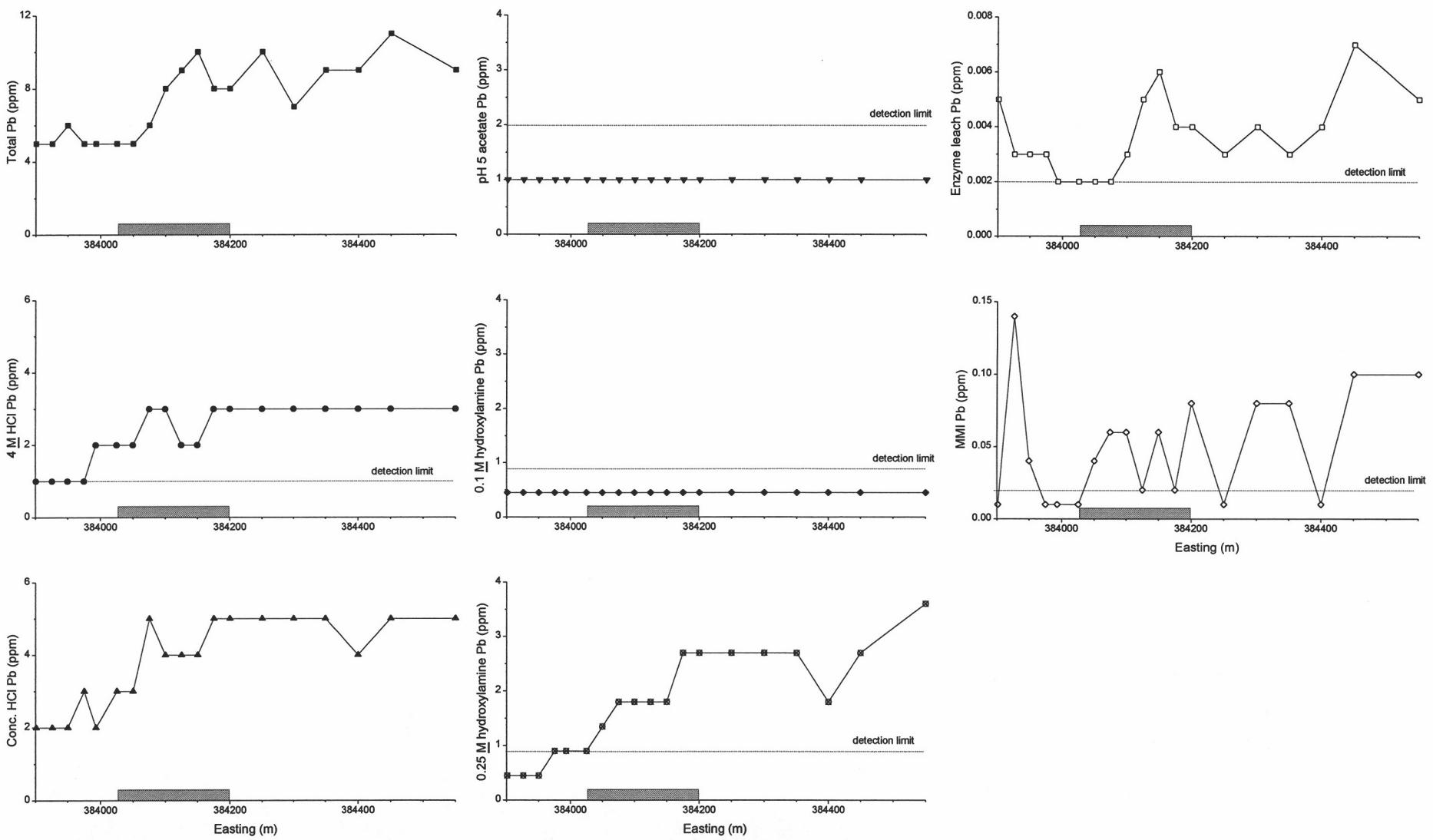
Figure A13.11: Total and extractable Pb from Apollo line 526080N.
