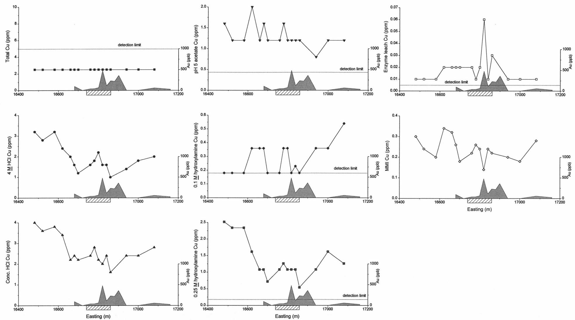
Figure A9.7: Total and extractable Cu from Bronzewing line 9800N.
