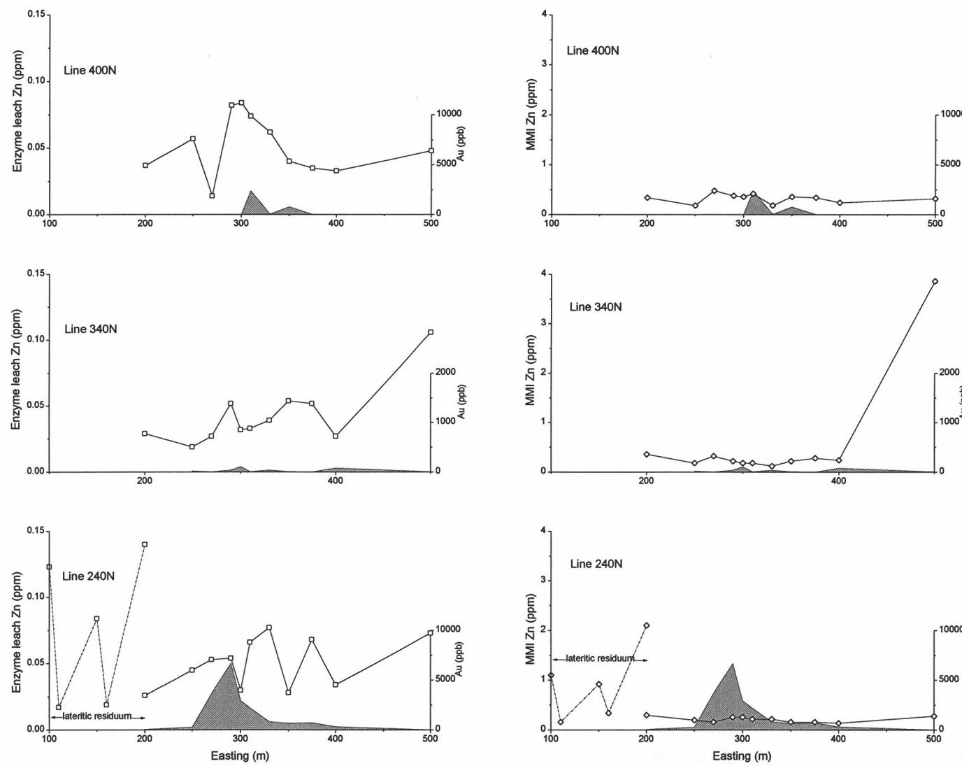
Figure A8.36: Enzyme leach and MMI Zn from Fender lines 400, 340 and 240 N.
