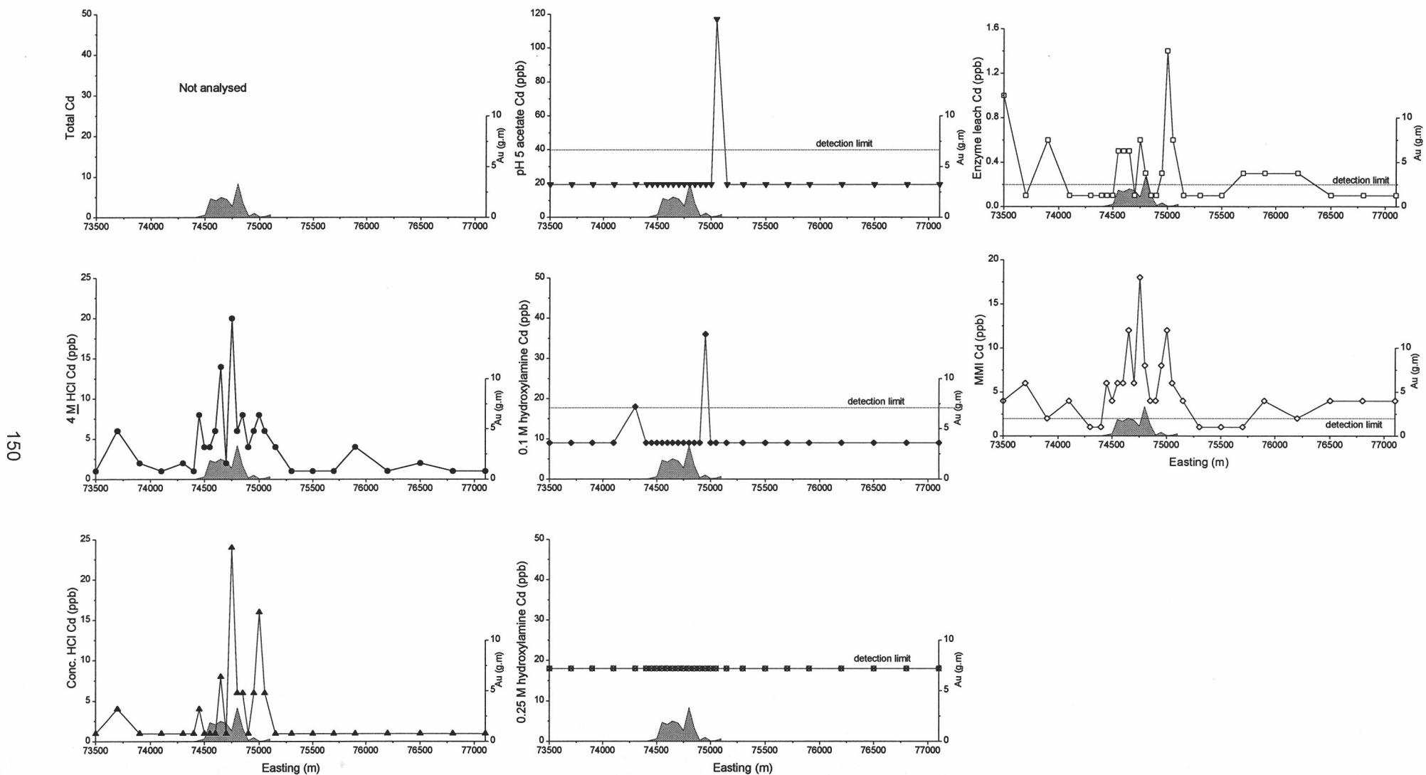
Figure A10.4: Total and extractable Cd from Curara line 27500N.
