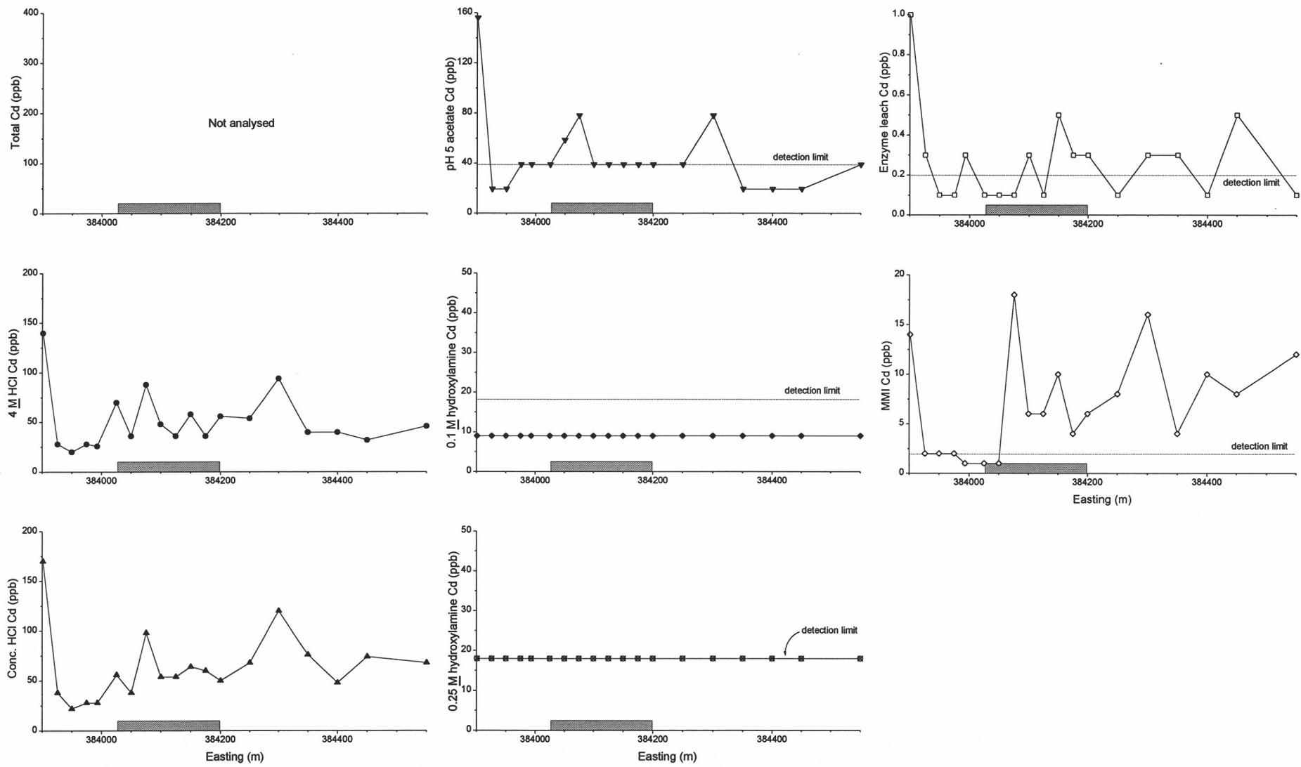
Figure A13.4: Total and extractable Cd from Apollo line 526080N.
