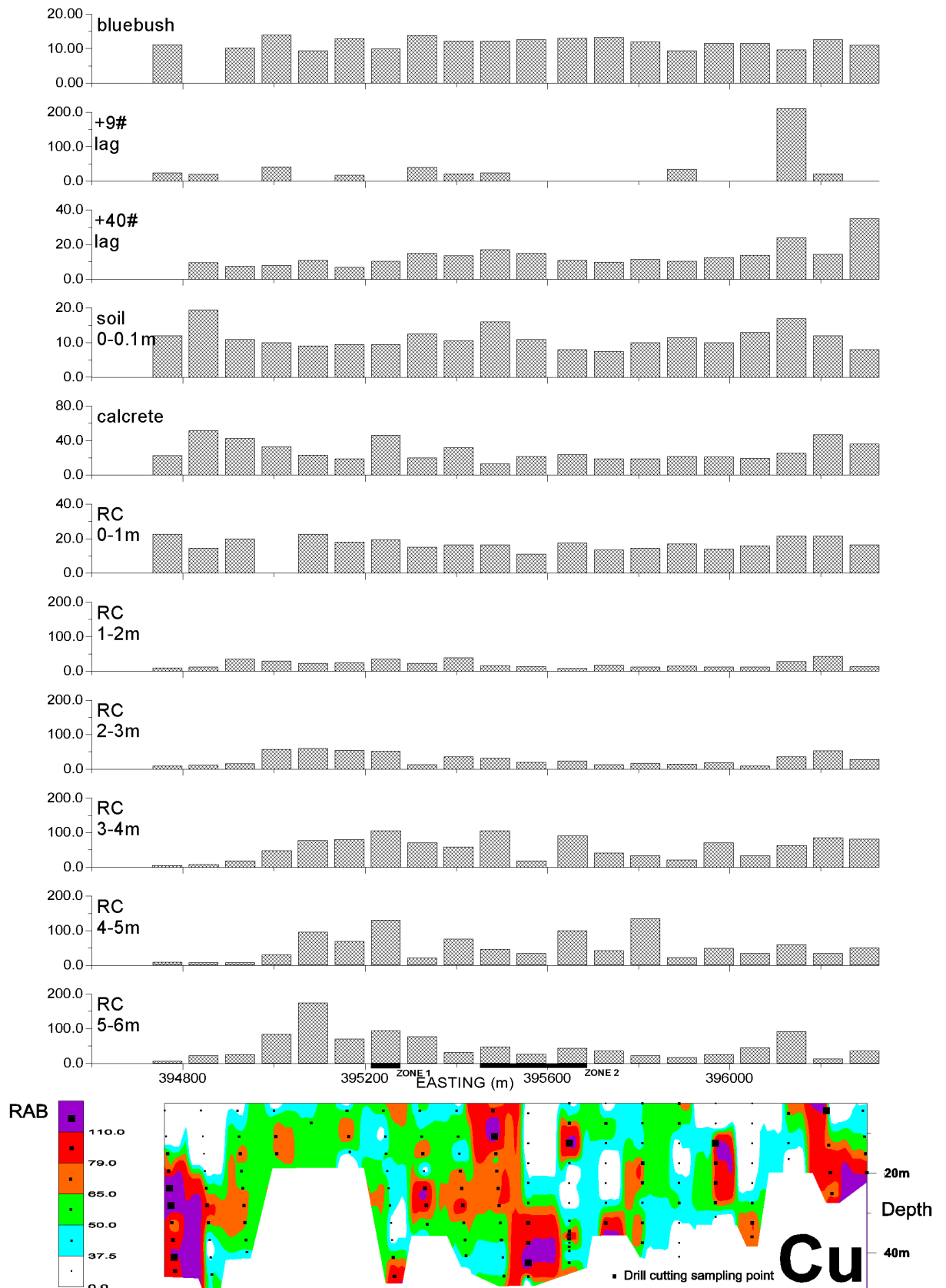
Figure A2.11a: Cu distributions in vegetation and regolith components. Data in ppm. Black rectangles (Zones 1–2) locate mineralisation. Contouring using Minimum Curvature gridding technique.
