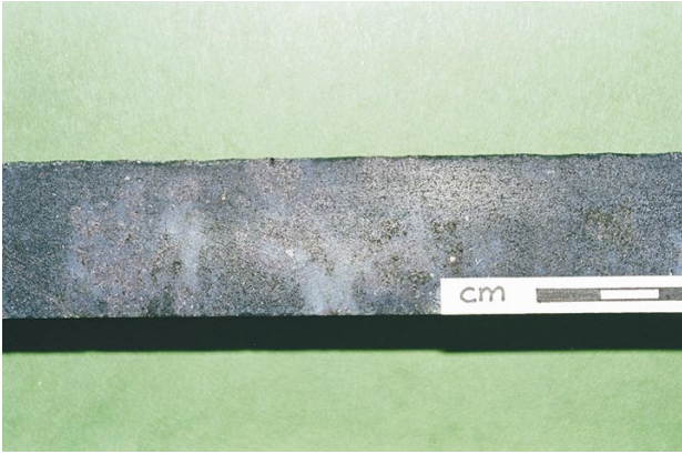
(a) Diamond drill 1/4 core (hole 97CDH1361, depth 40.43-40.51 m) Christie Gneiss felsic garnet-orthopyroxene-cordierite gneiss, Sample R367481. (Photo 45689)
