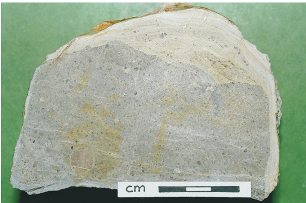
(b) Common silcrete, (grey billy) silcrete-mantled sandy silcrete, pedogenic, from pit GCP100 (depth of ~2.75 m) Sample R367478. (Photo 45519)
