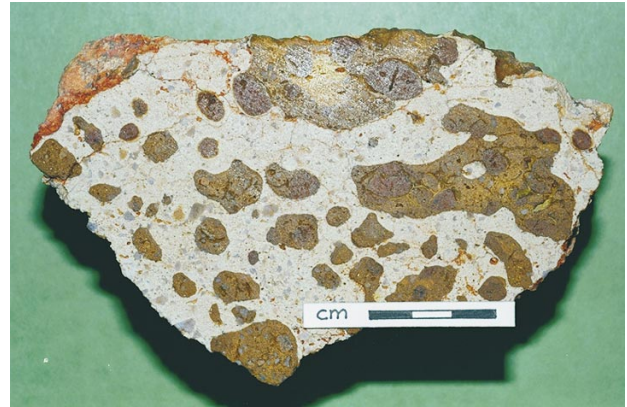
(d) Silicified sandy claycrete containing ferruginous material exhibiting a replacement texture, from a drillhole sump N of Mt Challenger (depth ~1 m, Field No. GC034) Sample R213520. (Photo 45675)
