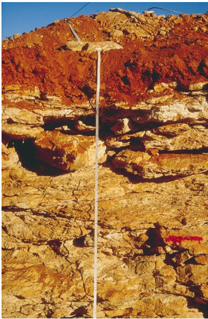
(b) Pit GCP106, SE face, top metre (red mark at 1 m) with central logged and sampled profile marked by measuring tape (Photo 45470)
