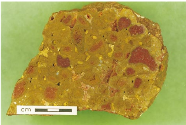
(b) Iron-rich grab sample consisting of siliceous, cutaneous ferruginous nodules and quartz. Sample R213976 from pit GCP129 spoil heap. (Photo 45666)
