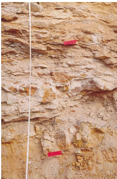
(c) Pit GCP110, SE face, ~1-2 m (red mark at 1 and 2 m) with central logged and sampled profile marked by measuring tape. (Photo 45501)
