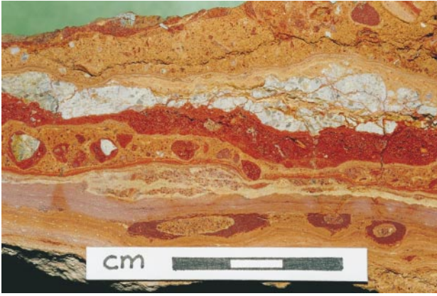
(a) Laminated silica-bearing calcrete from pit GCP110 (depth 1.0 m) sawn face (wet) revealing a complex multi-coloured interior; Sample R214109. (Photo 45566)
