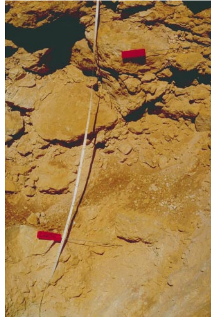
(c) Pit GCP122, SE face, ~1-2 m (red mark at 1 and 2 m) with central logged and sampled profile marked by measuring tape. (Photo 45478)
