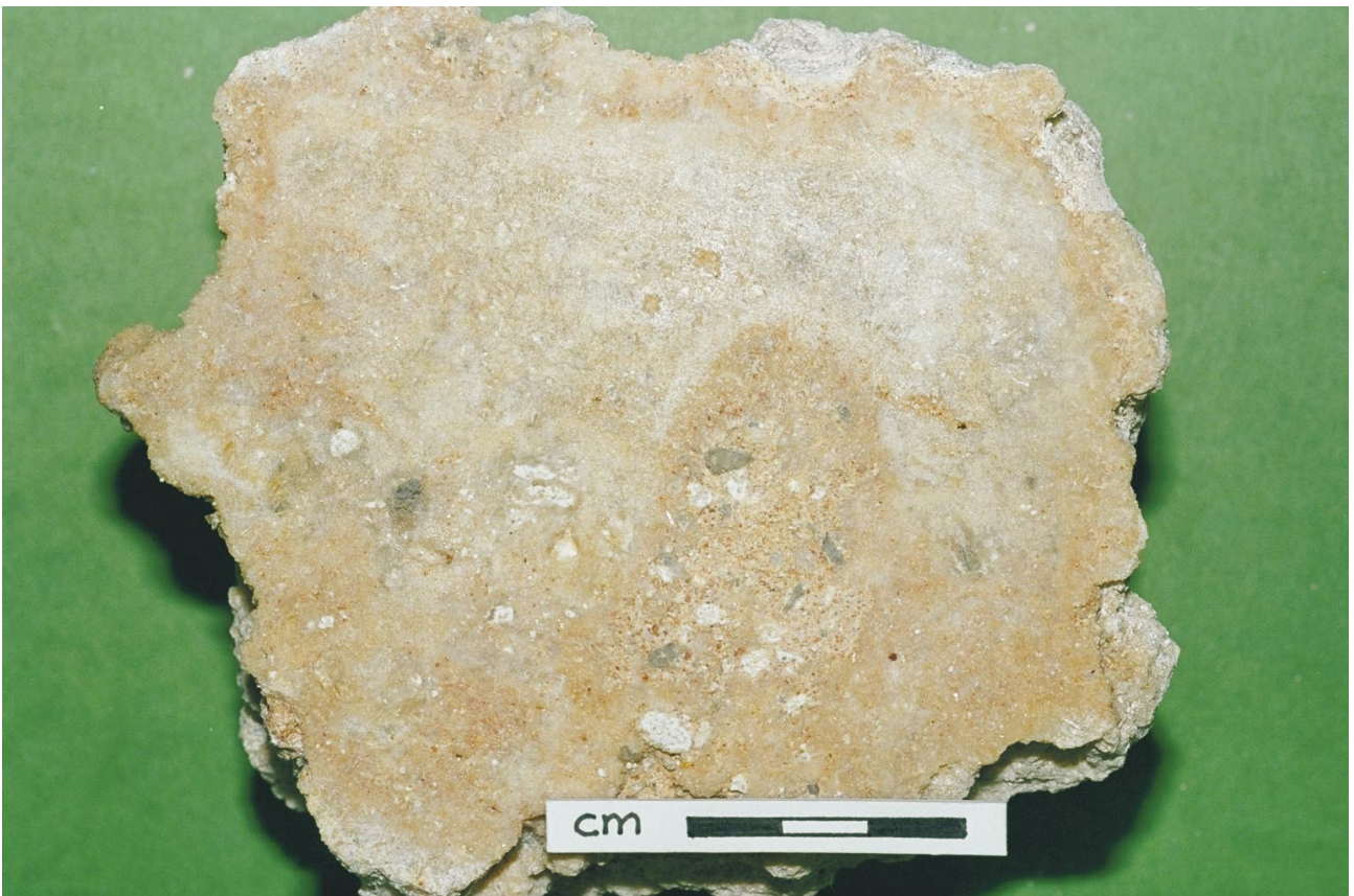
Massive gypsum with minor anhydrite and trace lithic fragments from pit GCP122 (depth 2.7 m), Sample R214049. (Photo 45614)
