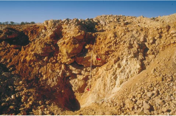
(a) Pit GCP123, wide angle view, SE face with logged and sampled profile marked by measuring tape. (Photo 45473)
