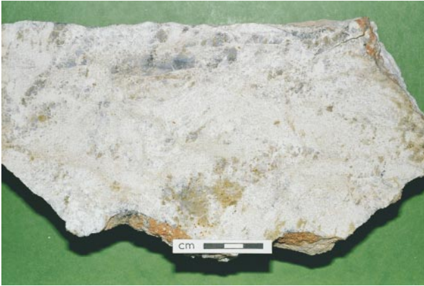
(a) Gold-bearing saprolite (100 ppm, weathered felsic gneiss) from pit GCP122 (depth 190-205 cm) directly above Challenger 1 mineralisation, sawn face (wet), Sample R214046. (Photo 45613)
