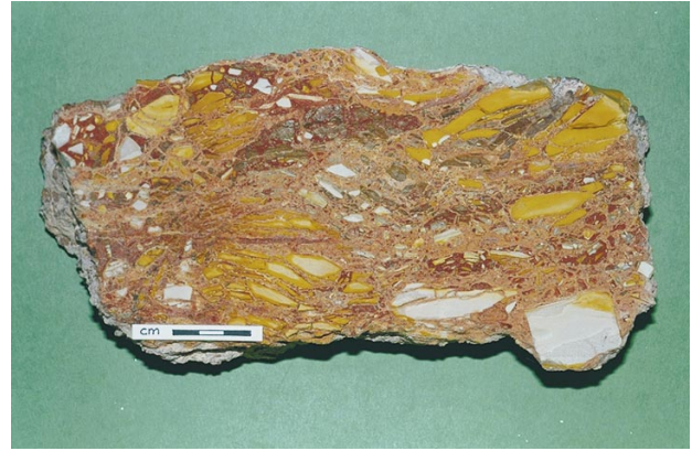
(c) A silica breccia, calcrete-cemented, generated from a surficial detritus accumulation (talus breccia). Components: large porcelanite fragments, ferruginous claycrete fragments, and quartz - all cemented by calcrete with minor hyaline silica, from pit GCP100 (grab h, depth ~1 m) Sample R367482. (Photo 45527)
