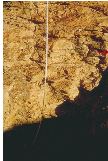
(d) Pit GCP106, SE face, 2.5-2.75 m (red mark at 2 m) with central logged and sampled profile marked by measuring tape. (Photo 45472)
