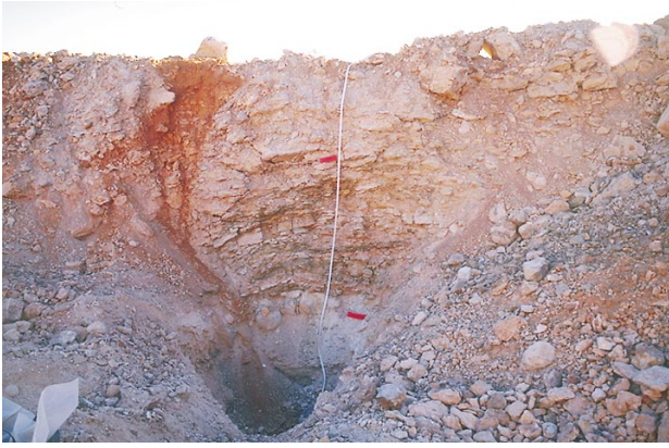
(a) Pit GCP100, wide angle view, NW face with logged and sampled profile marked by measuring tape. (Photo 45504)
