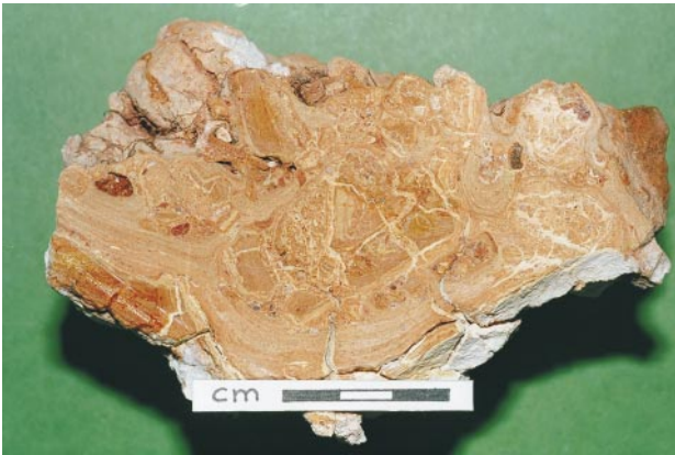
(b) Laminated calcrete aggregate from pit GCP129 (depth 15-25 cm) sawn face (wet), Sample R213981. (Photo 45665)
