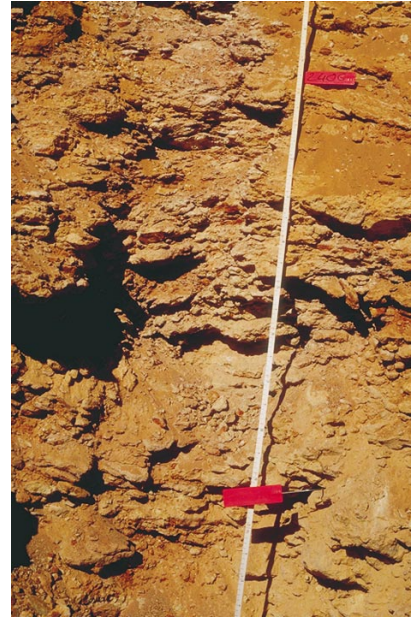
(c) Pit GCP115, SE face, ~1-2 m (red mark at 1 and 2 m) with central logged and sampled profile marked by measuring tape. (Photo 45487)
