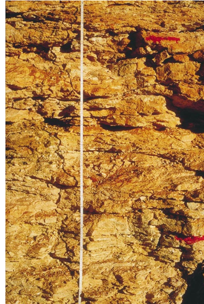
(c) Pit GCP106, SE face, ~1-2 m (red mark at 1 and 2 m) with central logged and sampled profile marked by measuring tape. (Photo 45471)
