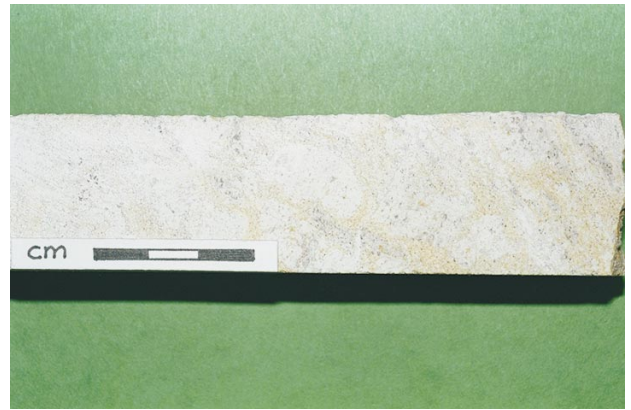
(e) Diamond drill 1/4 core (hole 97CHDH1361, depth 4.77-4.85 m) kaolinitic bleached upper saprolite, Sample R367486. (Photo 45694)
