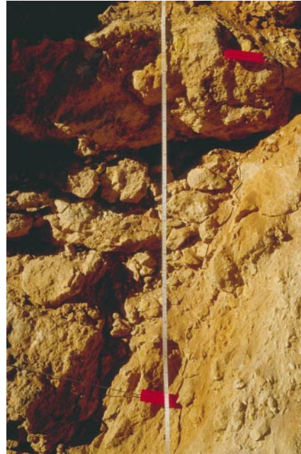
(c) Pit GCP123, SE face, ~1-2.2 m (red mark at 1 and 2 m) with central logged and sampled profile marked by measuring tape. Note: base of pit not photographed due to shadowing. (Photo 45475)
