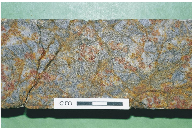
(c) Diamond drill 1/2 core (hole 97CHDH1361, depth 26.62-26.72) weakly weathered Christie Gneiss felsic garnet gneiss, Sample R367484. (Photo 45690)
