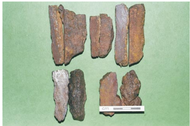
(e) Surface lag of ferruginised, strongly weathered rock with 1.3 ppm Au from near GCP122, Sample R214180. (Photo 45686)
