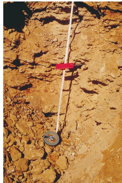
(d) Pit GCP115, SE face, 2.5-3 m (red mark at 2 m) with central logged and sampled profile marked by measuring tape. (Photo 45498)
