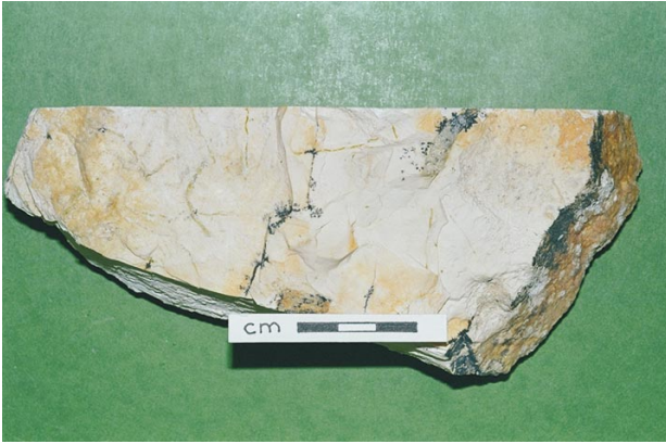
(a) Porcelanite - silicified siltstone (pale grey) exhibiting manganese oxyhydroxide dendrites (black) and some pale yellow ferruginous stains on fractures and partings. From pit GCP106 (depth ~2.7 m) Sample R214134. (Photo 45550)
