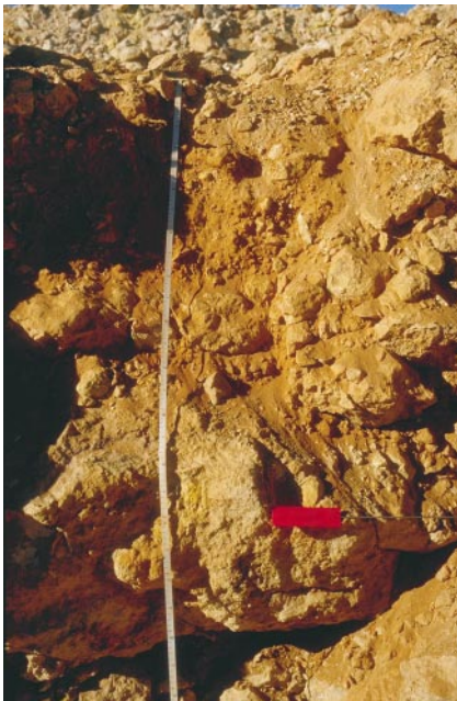
(b) Pit GCP123, SE face, top metre (red mark at 1 m) with central logged and sampled profile marked by measuring tape. (Photo 45474)
