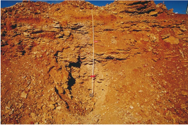
(a) Pit GCP115, wide angle view, SE face with logged and sampled profile marked by measuring tape. (Photo 45485)
