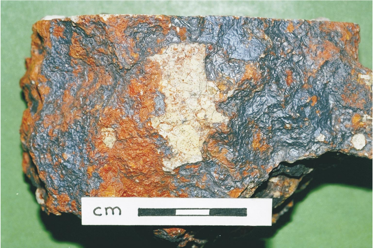
Black Mn oxide coating and orange Fe oxide staining on a block of clay-cemented conglomerate from pit GCP129 (depth 2.6-3.0 m), Sample R213974. (Photo 45655)
