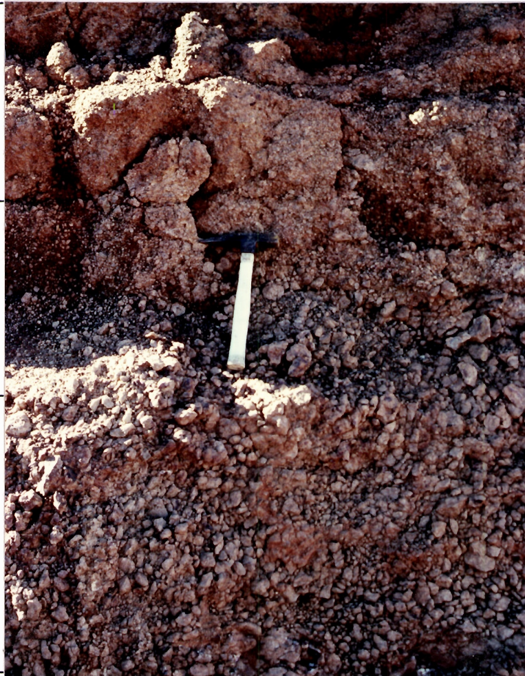
Fig.15A. Vertical profile showing weakly indurated nodular-pisolitic duricrust overlying collapsed ferruginous saprolite, location north east rim of McCaffery Pit.
