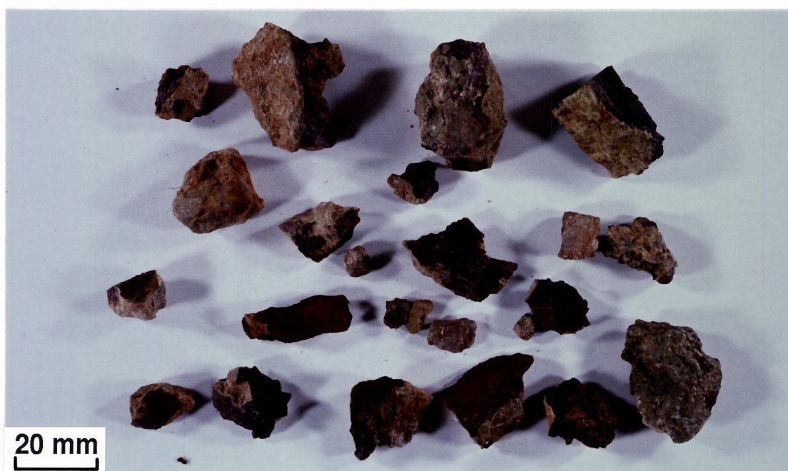
Fig.37B. Fragments of ferruginous saprolite showing reddish-brown to dark brown internal surfaces, Sample No. 07-1175, McCaffery Pit.
