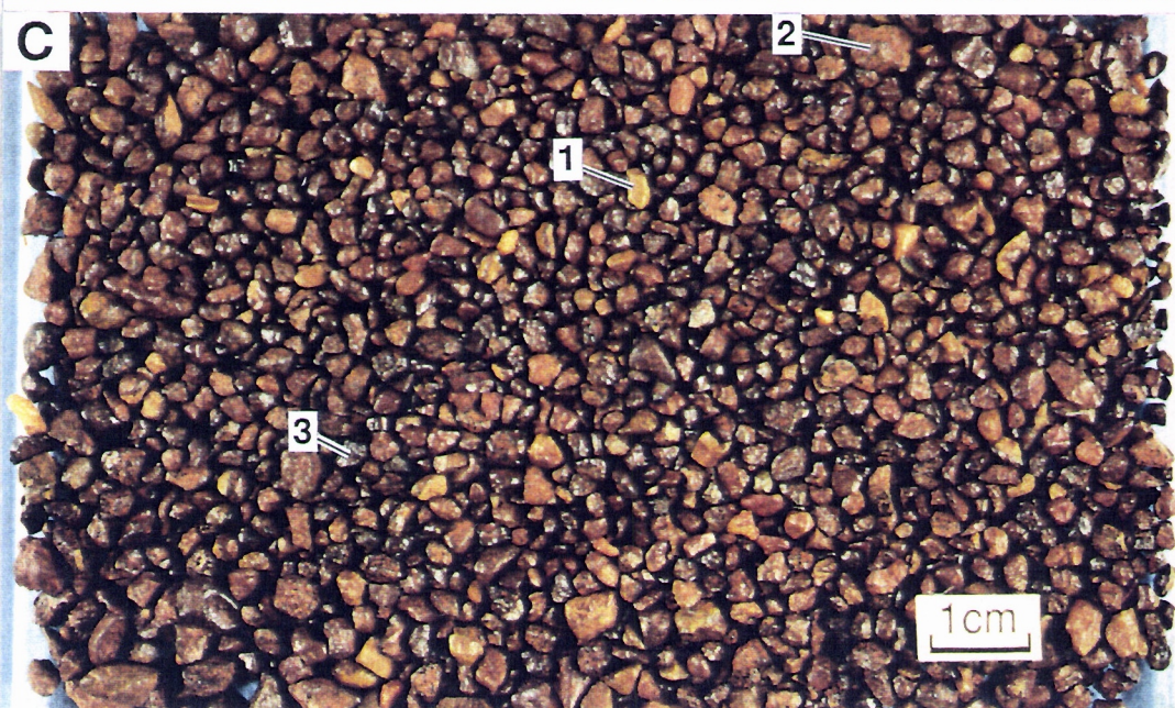
Fig.27C. Detail of fine lag of mixed origin showing fragments of ferruginous saprolite (1), lateritic pisoliths/nodules (2) and ferruginous granules (3). Sample 07-1330, Meatoa area.
