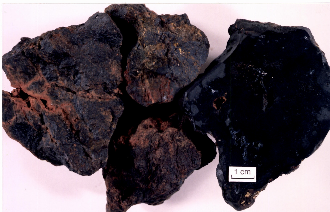
Fig.37C. Ferruginous cobbles of iron segregations, Sample No. 07-1221, 259744E, 6896694N.
