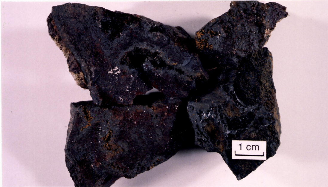
Fig.38A. Iron segregations showing box work texture after sulphides, Sample No. 07-1181, McCaffery Pit.
