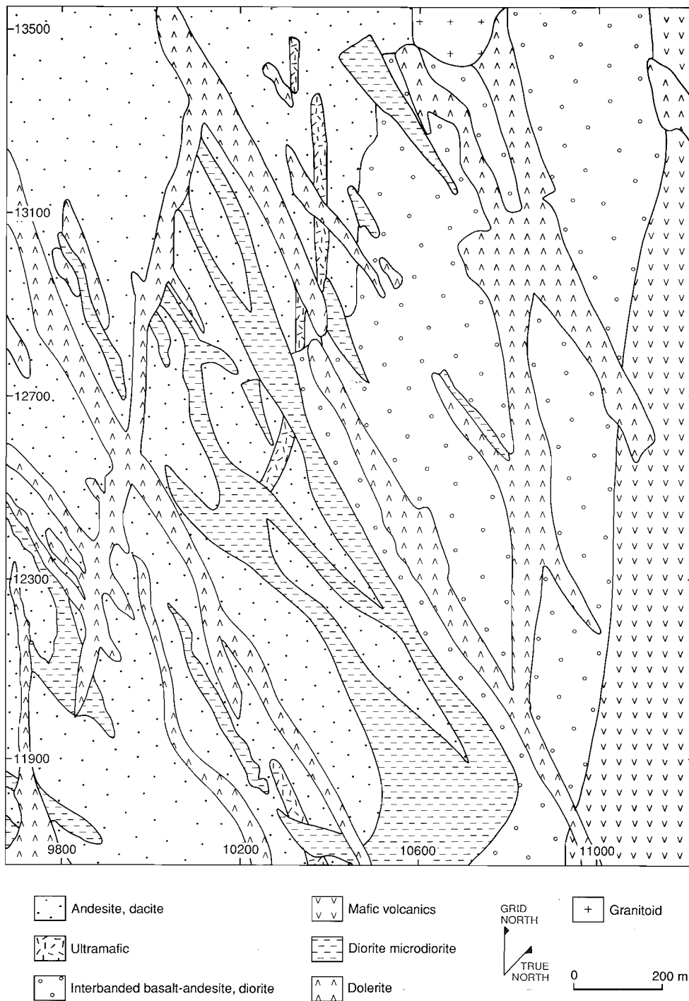
Fig. 24. Bedrock geology map of Pit A and its surroundings (modified after Symons et al., 1990).
