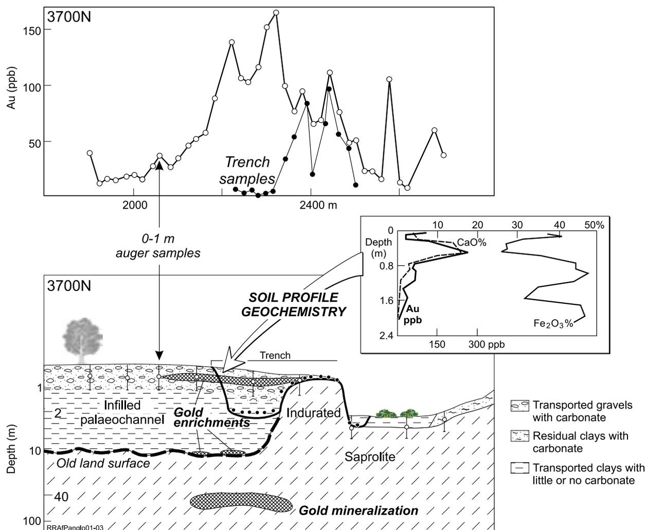
Figure 2. Section through 3700N (see Figure 1) showing topographic relationships and the distribution of calcrete and Au mineralisation. Shallow carbonate-rich samples from the trench give significant response to buried mineralisation, whereas deep, carbonate-poor samples have background Au contents. (after Lintern *et al.*, 1995)
