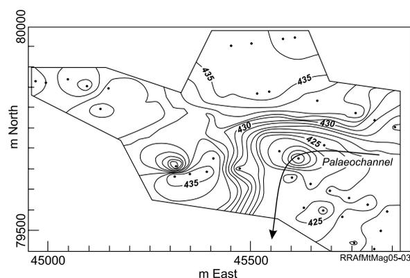
Figure 5. Contoured palaeotopography of eroded basement at Stellar showing the deeply eroded and curved palaeochannel to the southeast. Local grid coordinates.
