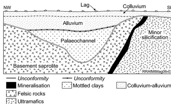
Figure 6. Regolith geology at Quasar showing an eroded basement, a palaeovalley infilled with mottled clays and cover of colluvium–alluvium.
