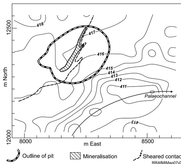
Figure 7. Contoured basement topography at Quasar with curved palaeovalley to the southeast. Local grid coordinates.
