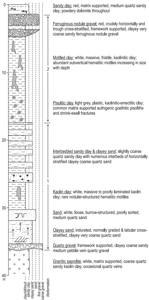
Figure 3. Composite lithostratigraphic column for the fills of inset-valleys sourced from weathered granite, as occurs in the centre of the LBE drainage basin.
