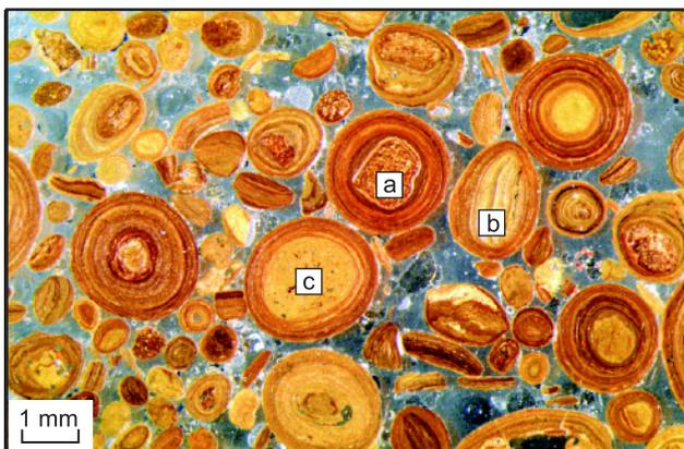
Figure 5. Thin section photomicrograph of goethitic pisoliths in kaolinitic-smectitic clays of AF2. Note variety of nuclei, including: (a) fossilized wood fragments, (b) fragments of older goethitic pisoliths, and (c) fragments of sandy clay.
