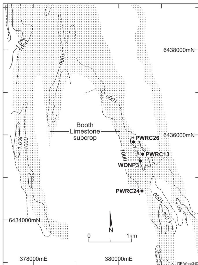
Figure 3. Distribution of maximum Zn (1000 ppm and 1.0% contours) in weathered bedrock from RAB drilling. Shaded area indicates distribution of Booth Limestone. The main Wonawinta area is in the SE quadrant.
