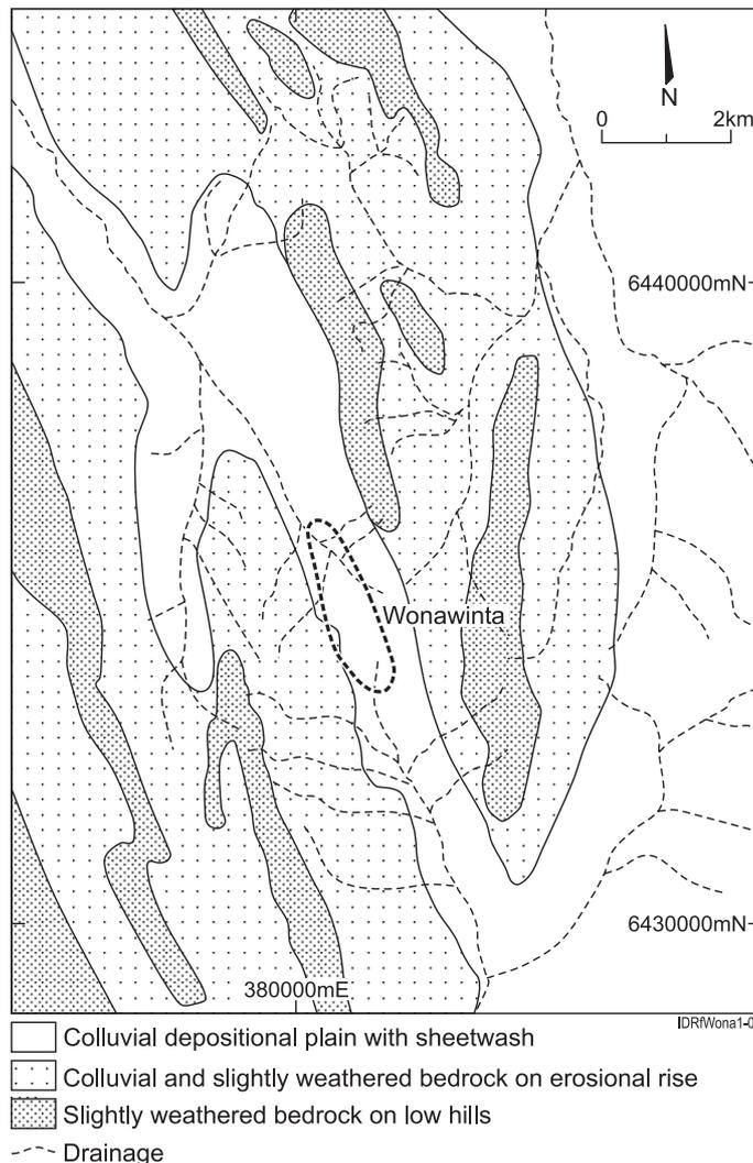
Figure 1. Local regolith geology of the area surrounding the Wonawinta prospect showing the dominant landform features and the distribution of colluvial material and weathered bedrock
