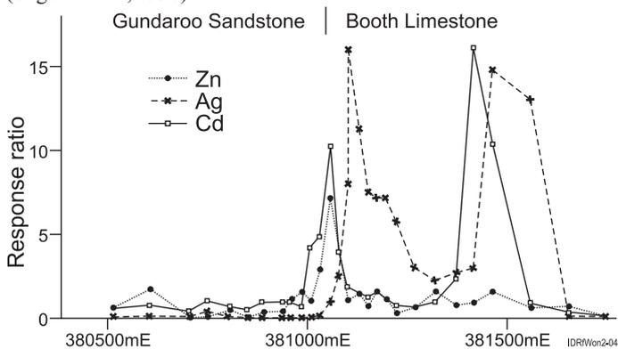
Figure 2. Partial leach soil sampling across Wonawinta on local grid line 10400N showing response ratio values for Zn, Ag and Cd. Response ratios are calculated by dividing by the batch median. Surface projection of Gundaroo Sandstone and Booth Limestone indicated.
