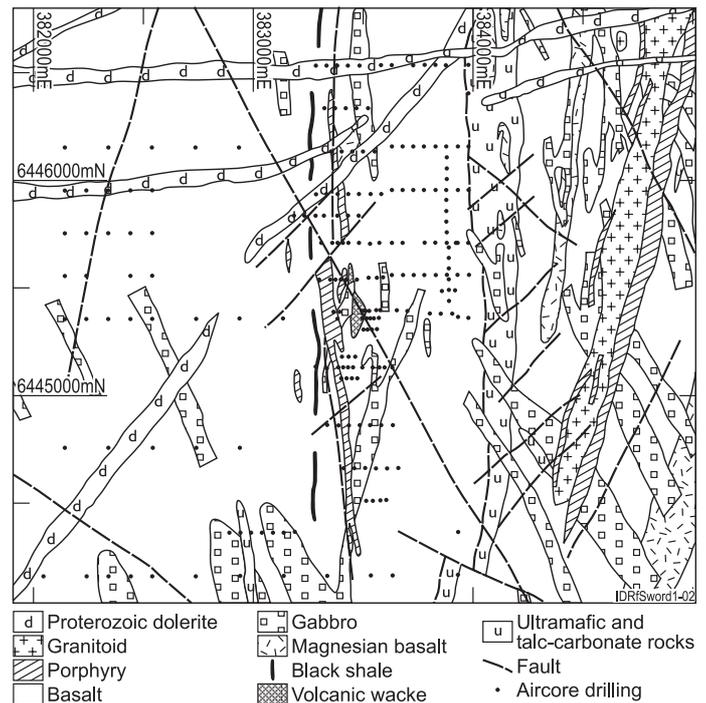
Figure 1. Geological map of the Swordfish prospect showing the aircore drilling. Figure 2 covers the western two thirds of Figure 1.
