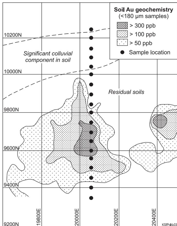
Figure 4. Plan of the ACM <180 μm Au in soil anomaly; sample locations refer to transect in Figure 5.
