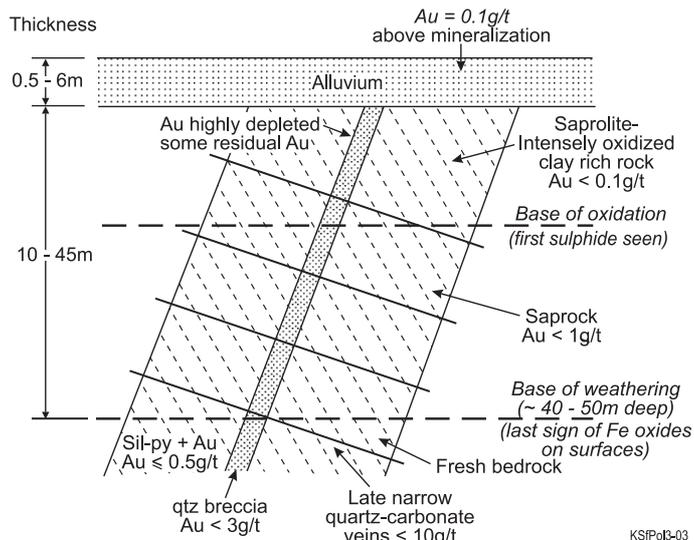
Figure 3. Schematic profile through weathered mineralization, Police Creek.
