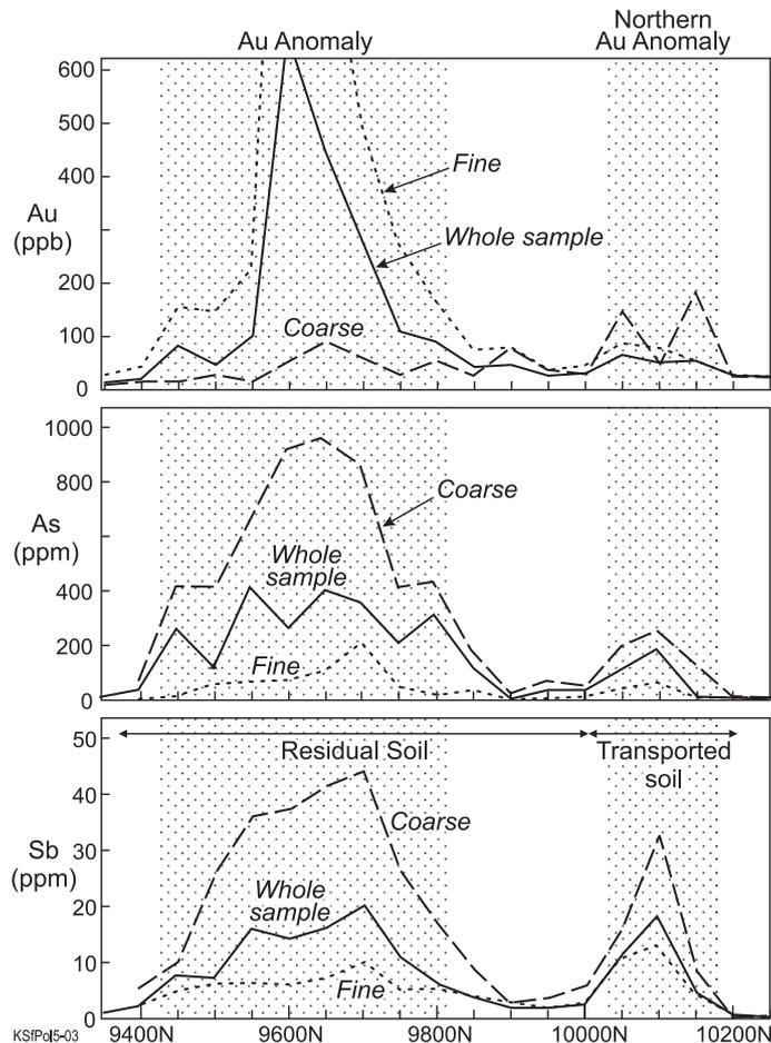
Figure 5. Distributions of Au, As and Sb in the fine (<75 μm), coarse (<180 μm) fractions and whole soil along traverse 20050E (see Figure 4 for location of traverse).
