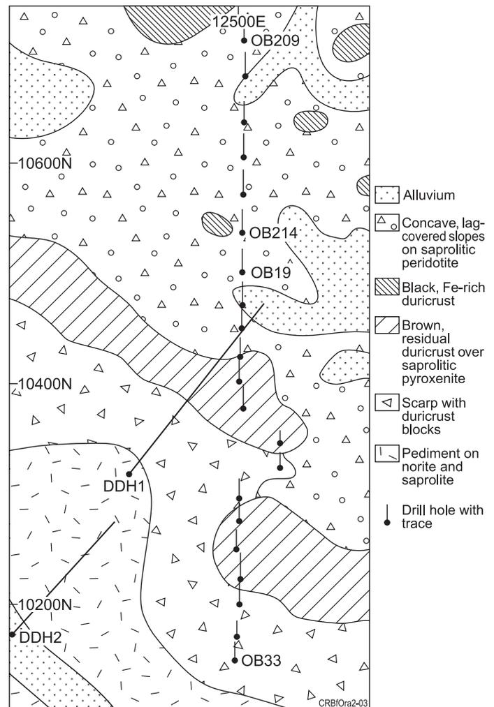
Figure 2. Regolith geology of part of the Ora Banda PGE prospect, indicating sites of lag sampling and drilling.
