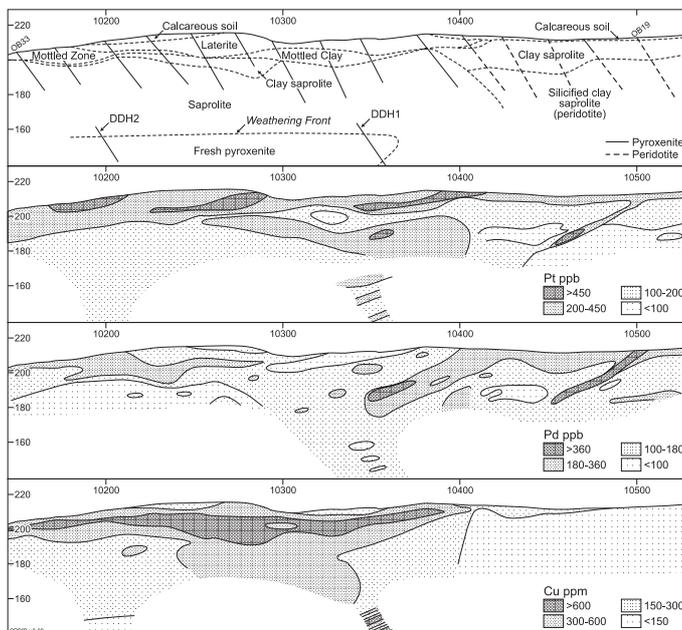
Figure 3. Drill section 12500E, Ora Banda, indicating regolith and bedrock geology, and distributions of Pt, Pd and Cu. Tracks of diamond drill holes show where they pass through the section (compare Figure 2).
