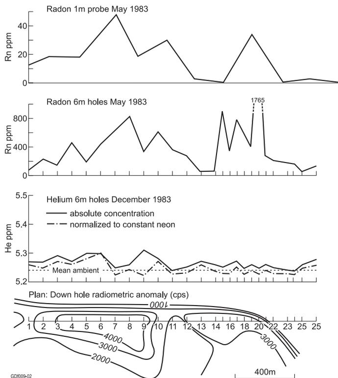
Figure 4. Concentrations in overburden gas of helium (6 m depth) and radon (1 m and 6 m depth), Mulga Rock deposit (from Butt and Gole, 1985).
