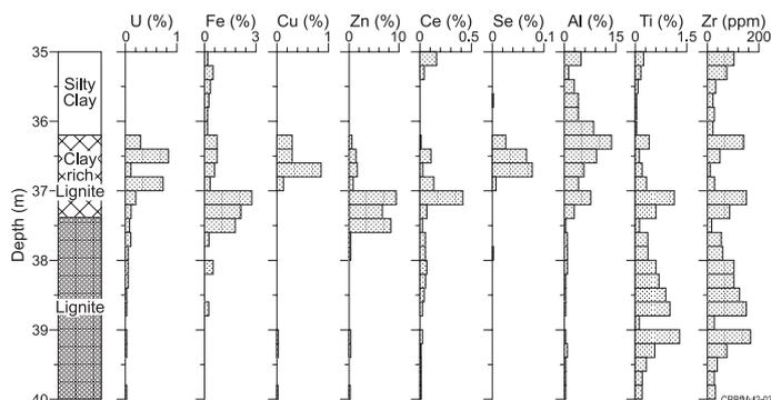
Figure 2. Representative downhole geochemical profile, Ambassador Deposit. The redox front is within the clay-rich lignite. Materials above 35 m are barren.
