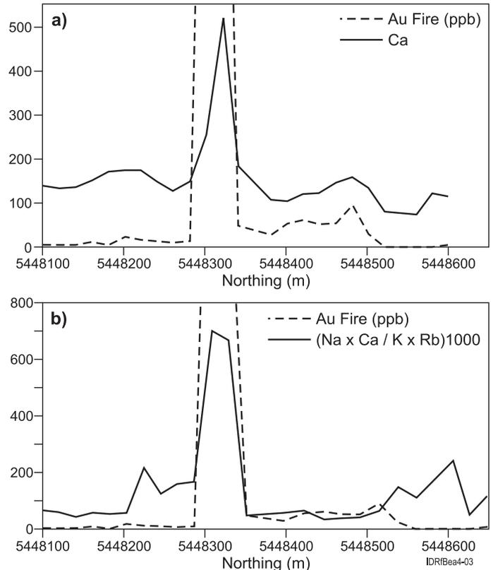
Figure 4. Match of Au by fire assay in the soil B horizon and Ca in the acid insoluble residue of the same sample, across the Volunteer Reef (section AA in Figure 2), line 500050E, Lefroy. Na and Ca enrichment and K and Rb depletion over the reefs can be used as reef indicators, enhanced as the index  $(Na \times Ca / K \times Rb)1000$ . The smaller peak at 5448500N indicates the Land O'Cakes Reef. See Figure 2.
