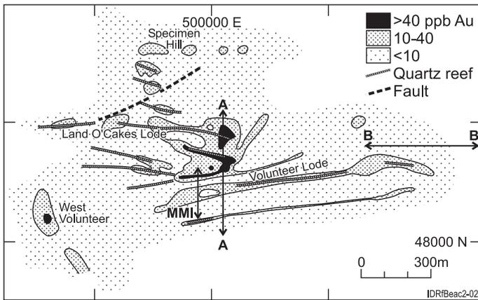
Figure 2. Soil B horizon soil Au anomaly over the Volunteer and Land O'Cakes Lodes, at Lefroy (Keele 1996). For cross section MMI see Figure 3. For cross section AA see Figure 4. For line BB results see text.
