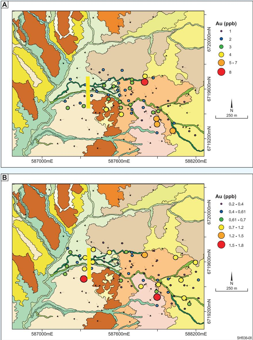
Figure 41: Gold contents from samples taken from 'White Elephant' catchment where a mineralised alteration zone (yellow line) is buried by > 5 m Mesozoic and Cenozoic sediments. (A) 75–200 µm size fraction from soils (B) black bluebush twigs. Map datum GDA.
