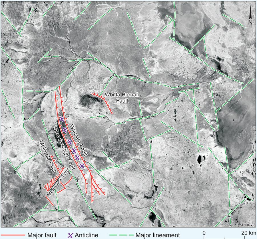
Figure 33: Morphotectonic map of active fault and fold structures in the Tibooburra–Milparinka area.
