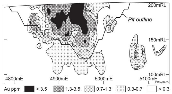
Figure 2. Cross section (15150mN) through the McKinnons deposit.
