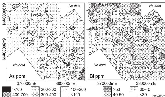
Figure 3. Contoured plots of gridded As and Bi fine fraction (<200 μm) soil data, using a partial dilute HCl digest, showing depletion haloes.
