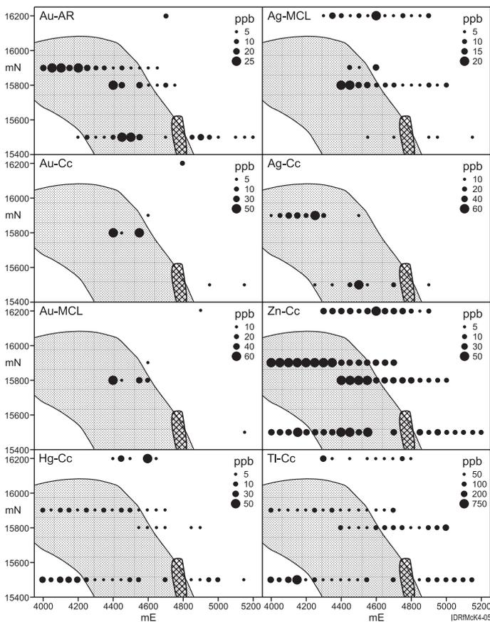
Figure 5. Circle plots of magnetic lag samples analysed for Au and Ag after Aqua regia (AR), Conc. HCl (Cc) and Micro cyanide leach (MCL) digests on orientation traverses N of the McKinnons Au Mine. The IP chargeability anomaly is the stippled area, the Au mineralization intercept is the cross-hatched zone and potential lode Au trends outlined.
