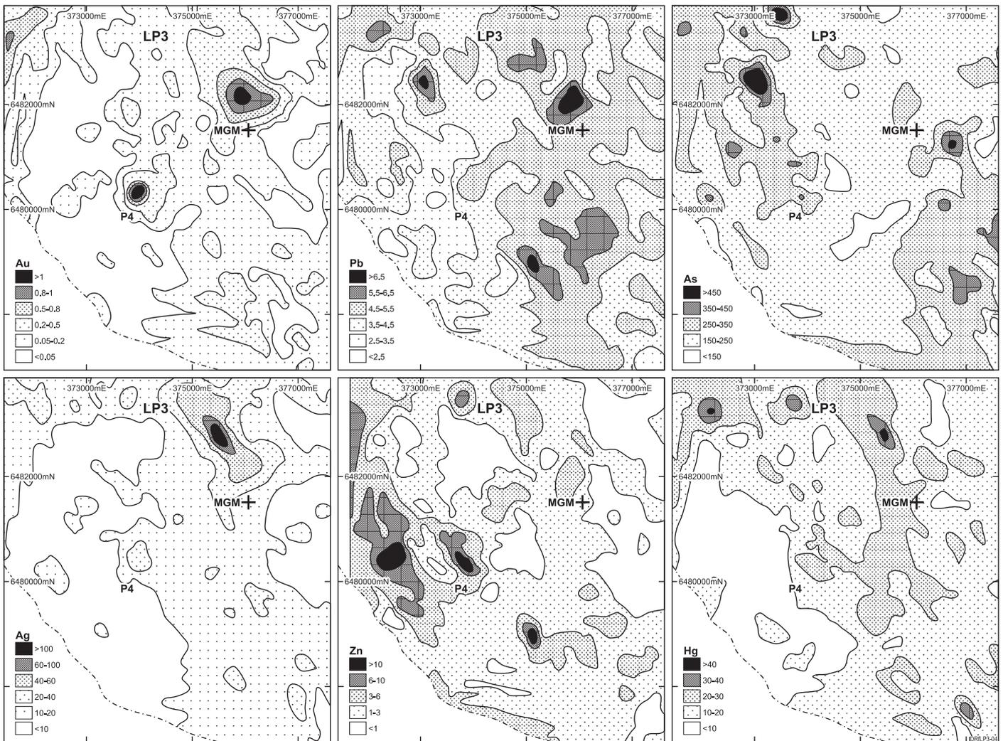
Figure 3. Partial leach (dilute HCl) geochemistry of the <75 μm soil fraction of Au (ppb), Pb (ppm), As (ppb), Ag (ppb), Zn (ppm) and Hg (ppb) of the area in Figure 1. Also shown are the P4 mineralization (P4) and the McKinnons Gold Mine (MGM).
