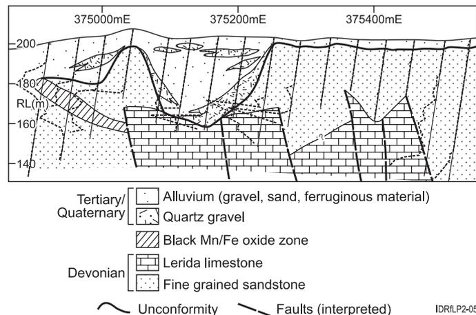
Figure 2. Geological and Zn geochemical section across Anomaly LP3 on oblique traverse centred at 375213E 6483689N.
