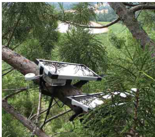
Stephen Burgess installing the wireless sap flow system in a giant sequoia, Kings Canyon National Park, California
