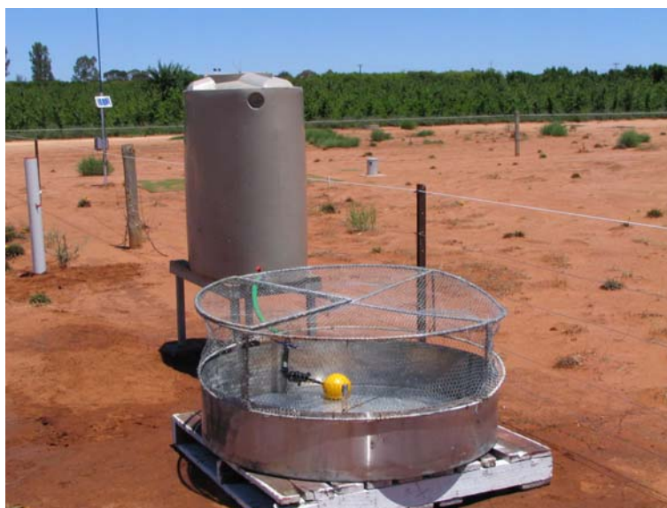
Figure 4: The evaporation pan set-up at the Loxton Research Centre (picture by Julie Corriveau).
