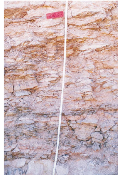
Plate 28: Pit GCP100, NW face, top 1-2 m (red mark at 1 m) central logged profile indicated by tape (Lintern and Sheard, 1999b). (photo 45506).
