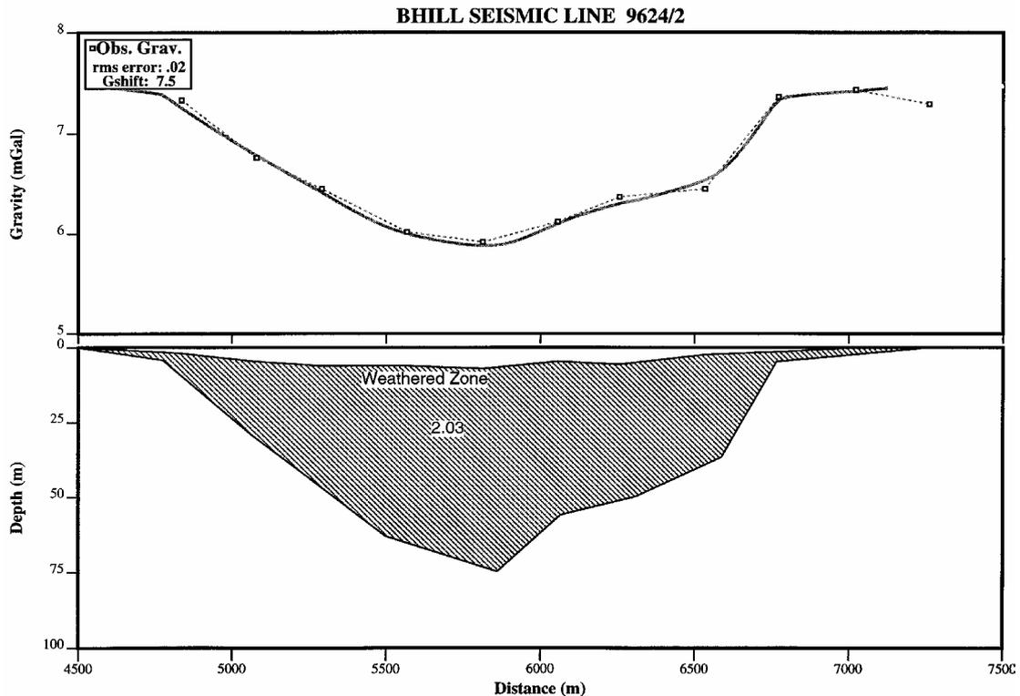
Figure 2. Gravity profile and 2D model of a palaeochannel filled with alluvium of density  $2.03 \text{ t/m}^3$  showing the depth to fresh bedrock of density  $2.67 \text{ t/m}^3$ . This example is from GA seismic line 9624/2 south of Broken Hill, described by Gibson, et al. (1997) and Foster and Shirliff (1998).
