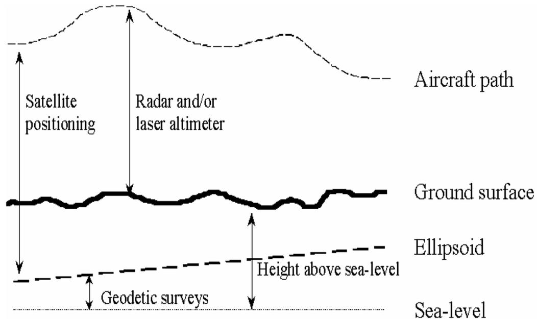
Figure 6. Method for deriving elevation (ie. the height above sea level) from airborne measurements. A GPS system on the aircraft measures the height of the aircraft above the ellipsoid. An altimeter measures the height of the aircraft above the ground (“terrain clearance”). The separation between the ellipsoid and sea level is known from geodetic surveys. Height above sea level is calculated as height above the ellipsoid plus the ellipsoid – sea level separation minus the terrain clearance.
