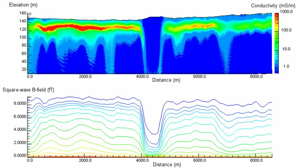
Figure 14. CDI conductivity section and TEMPEST Z component window response amplitudes for line 10390, Lake Harris, South Australia. The 1D assumption in CDI calculation results in “drooping moustache” edge artifacts at strong lateral contrasts in conductivity. Examples are evident at distances of 4000 and 4650 m along this line. Weakly elevated conductivity values extending from the conductive near-surface layer to depth at 0-200 m, 2700-3000 m and 7000 m are more subtle edge effects.
