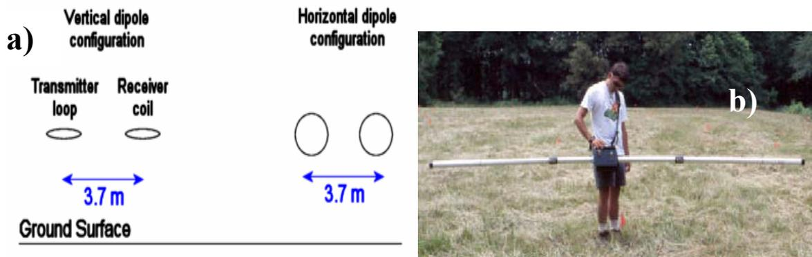
Figure 7. a) Transmitter loop and receiver coil configuration for the EM31 frequency domain ground EM instrument showing both vertical and horizontal dipole configurations. b) EM31 instrument in operation.
