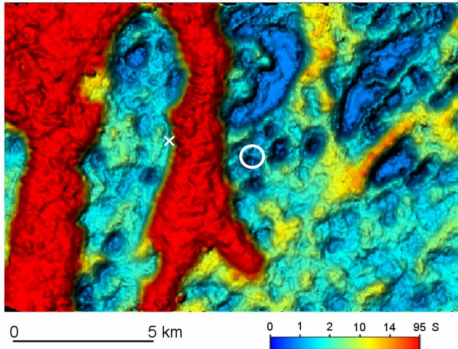
Figure 11. Image of conductance of the conductive unit defined by a variable conductivity with a minimum threshold of 30 mS/m, calculated from TEMPEST AEM data for the Challenger area, South Australia. The location of the Challenger deposit is shown with a white circle. The location of a borehole into one of the deep channels is shown with a white cross.
