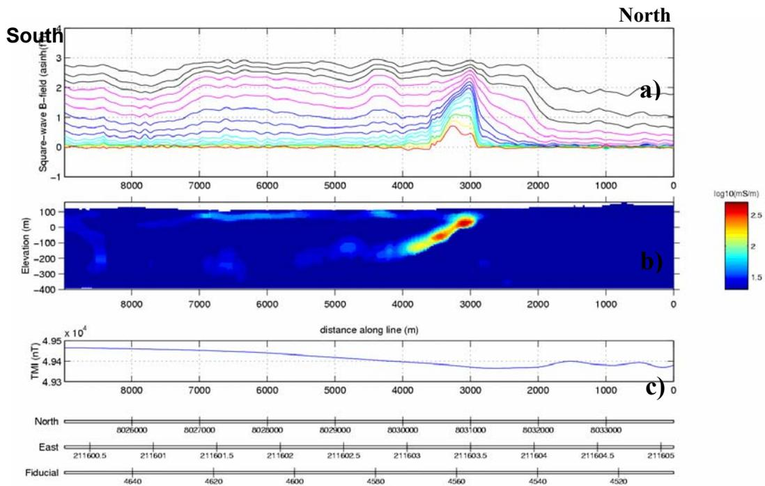
Figure 9. a). TEMPEST AEM Z-component square-wave B-field response profiles. b). conductivity section; and, c). total magnetic intensity profile for line 10281 (211600 mE) over the Walford East base metal prospect, Queensland (Lane, et al., 2000).
