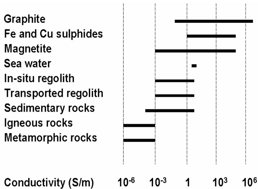
Figure 1. The range of conductivity values for various rocks and minerals.
