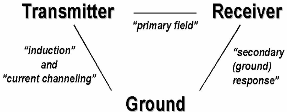
Figure 2. Interactions for an EM system.
