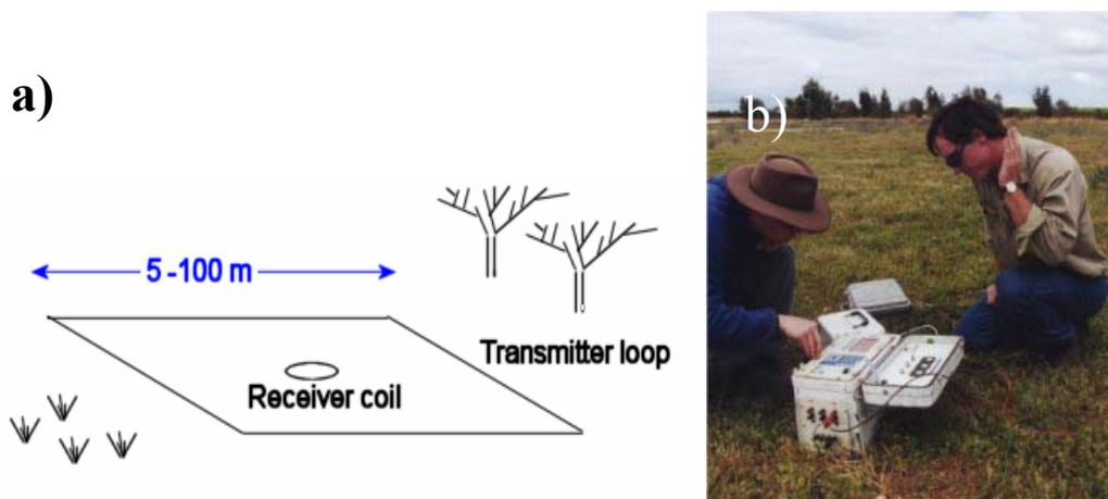
Figure 8. a). Transmitter loop and receiver coil configuration for typical in-loop time domain ground EM. b). Time-domain ground EM instruments (NanoTEM transmitter and GDP data recorder). (Photo courtesy: Mike Wall, University of Adelaide).
