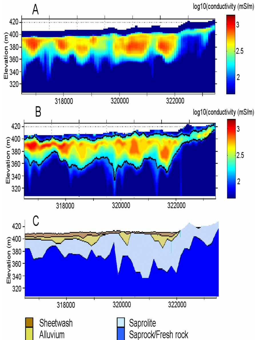
Figure 10. Conductivity sections for a) PROTEM ground EM and b) TEMPEST airborne EM data along line 6626720 mN at Grant's Patch, Western Australia. The upper and lower bounds of a 'conductive unit' with a minimum threshold of 100 mS/m are shown over the TEMPEST section. The regolith profile derived from drilling c) is also shown (Worrall, et al., 2001).
