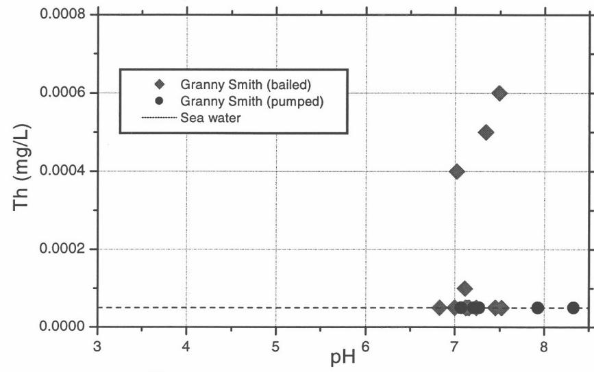
Figure A4.35: Thorium vs. pH for groundwaters from Granny Smith.
