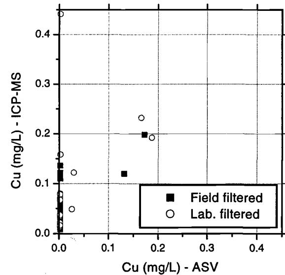
Figure A2.4: Cu (ICP-MS) vs. Cu (ASV).
