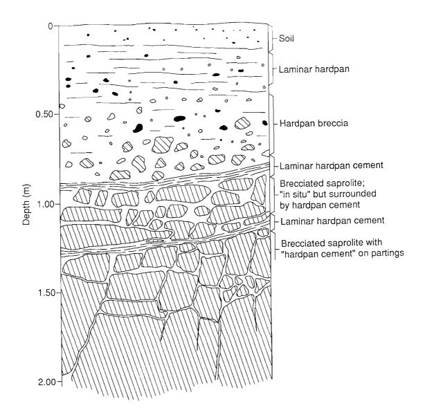
Figure 1. Section through typical hardpan profile, Youanmi goldmine, illustrating gradational contact between colluvium and saprolite.
