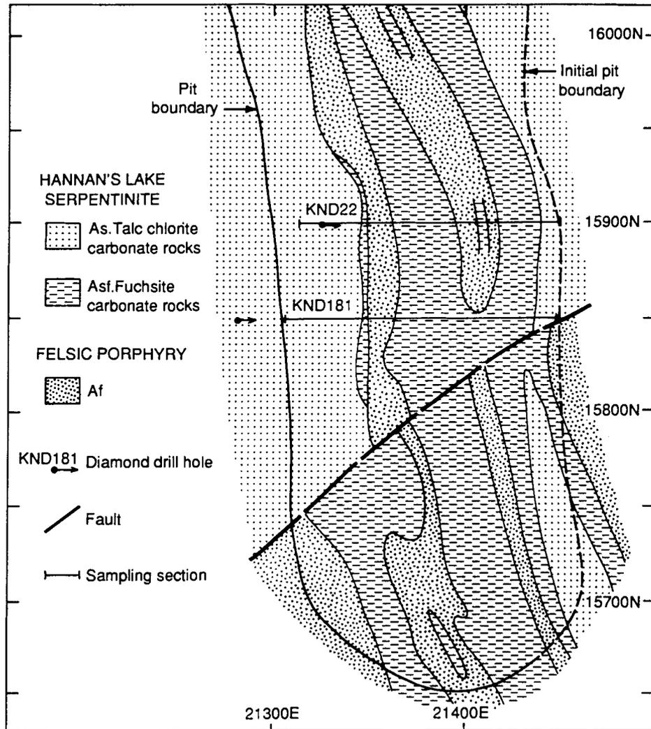
Figure 1: Geology of the southern end of the Mystery Zone, Mt. Percy, projected to 400 m RL, indicating the two sections selected for study. Information derived from pre-mine drilling, supplemented north of 15750N by in-pit mapping (T. Bradley, KCGM) and data from this study.
