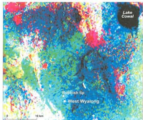
**Figure 8:** Radiometric image showing area with mottled granite saprolite and magnetic pisolith lag (light blue/green) north of West Wyalong.
