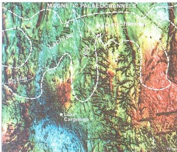
**Figure 7:** Magnetic image from Lake Cargelligo area showing magnetic palaeochannels.
