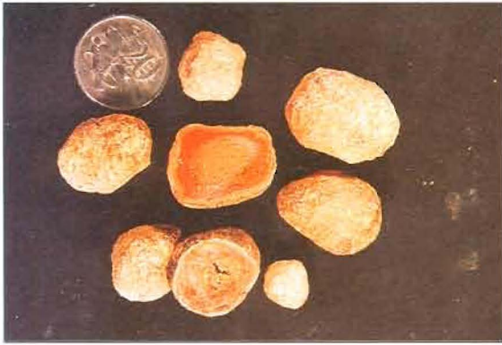
Figure 3(a): Photographs of selected morphological facies for regolith carbonate accumulations. a) nodular carbonate facies from the Marnpi profile
