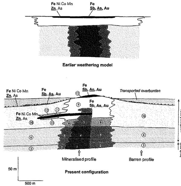
Fig. 2 Colour gradient and lateral dispersion around the McKinnons deposit.
