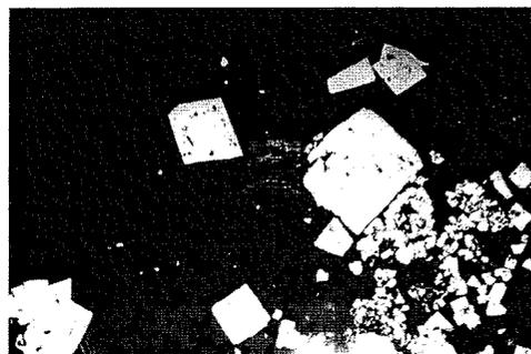
Supergene pyrites (large) against corroded primary pyrites (small)
