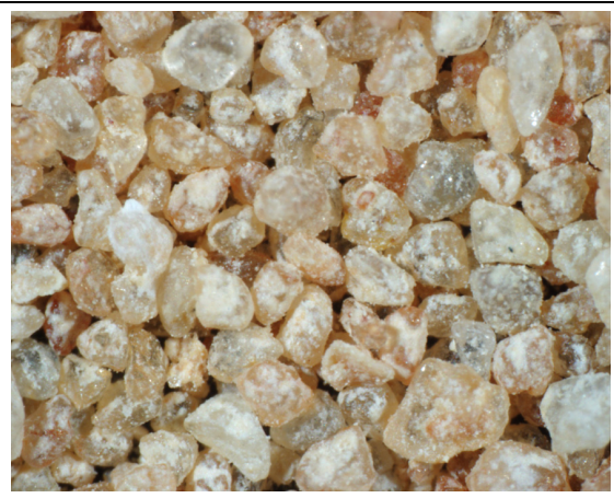
Plate 2: Ooldea Range (W. of Immarna Siding) dune sand displaying rounded to subrounded quartz grains with a dusting of carbonate and clay. Plate scale 2.8 x 2.25 mm. (Sample IA1/3.5, R2142810).
