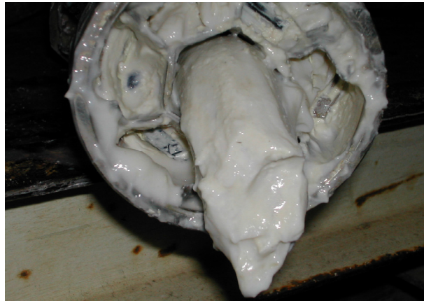
Figure 1. Clogging of pump and impellers by amorphous Al(OH) 3 (from James-Smith et al. 2005).
