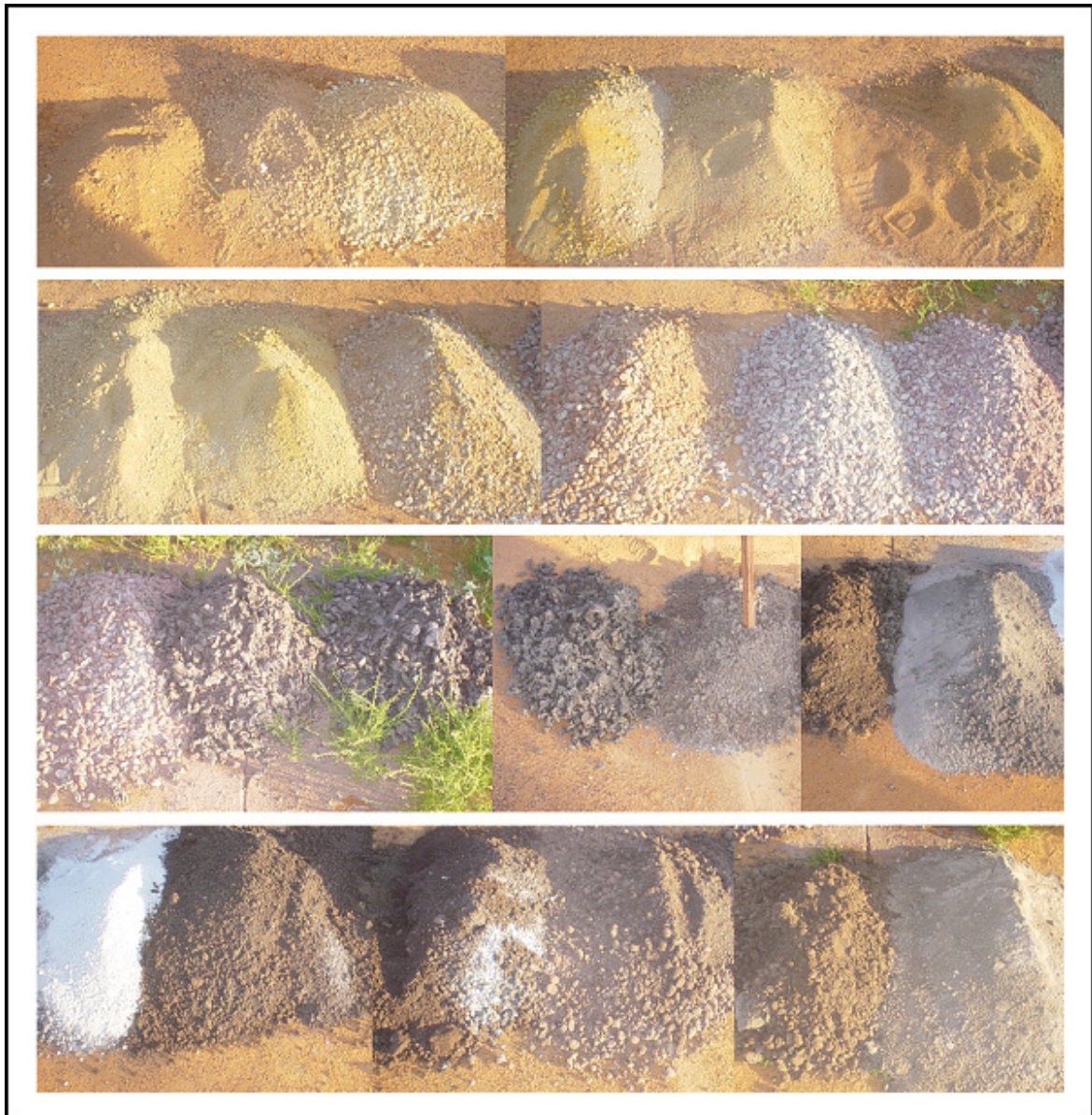
Figure 5, Images of the fresh drill cuttings recovered by Havilah Resources NL
