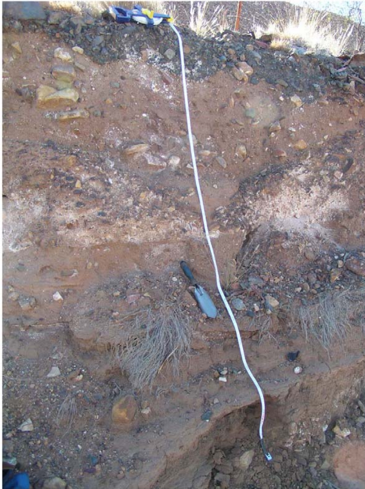
Figure 4: Photograph of cut riverbank OB3. The dark coloured, upper most layer is rich in slag deposits and has the highest corresponding sediment Zn with a value of 3960 ppm (Figure 3). Mid way down the section the sequence appears to have undergone oxidation with the precipitation of a probable calcium sulphate deposit on the outer surface.
