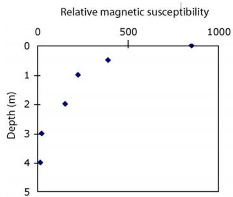
**Figure 3:** Variation of magnetic susceptibility with depth for larger pisoliths at the Jacaranda pit profile, Andoom.
