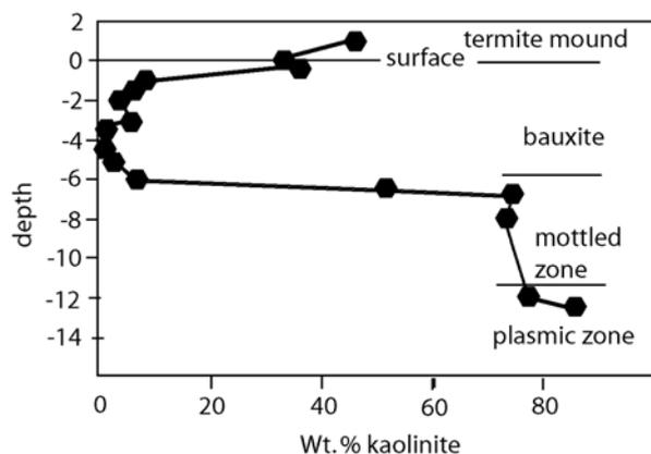
**Figure 4:** Kaolinite content through the plasmic, mottled and bauxite horizons, in soil at the surface and in a Cathedral termite nest wall.
