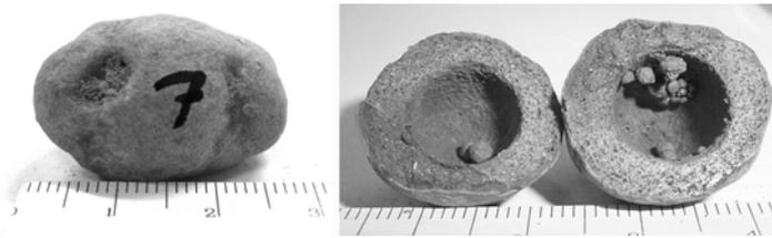
**Figure 5:** Nodule from the Weipa bauxite. Left, entire, showing aperture plugged by small particles. Right, sectioned, showing hollow interior and a few adventitious ooliths.
