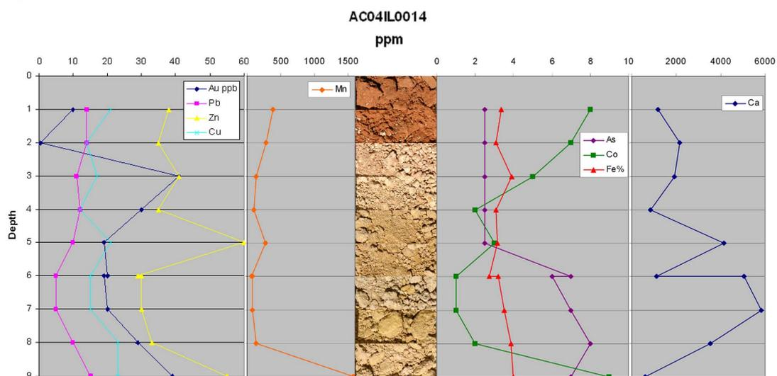
**Figure 4:** AC04IL0014, downhole geochemistry with photos of the dry samples.
