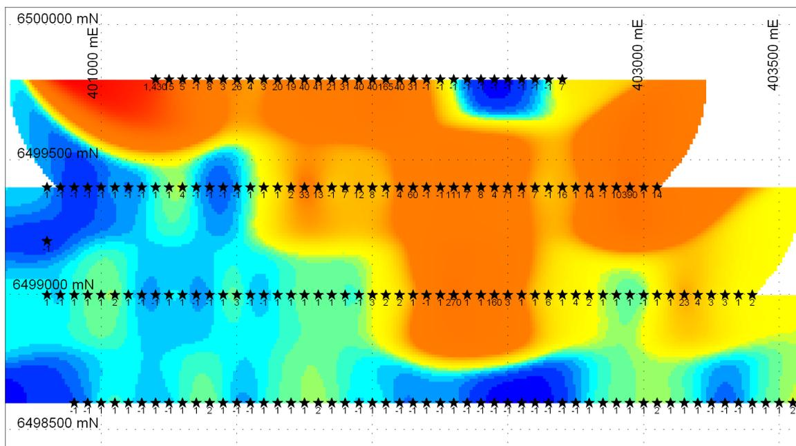
**Figure 6:** IDW grid for Au ppb, split in two zones with a 10 m cell size, 500 m search and display radius and a high exponential rate of decay (8).
