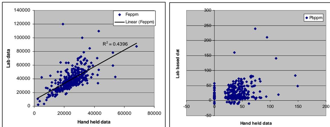
**Figure 3:** Scatter plots for hand-held XRF versus laboratory ICP OES data for Fe (left) and Pb (right).
