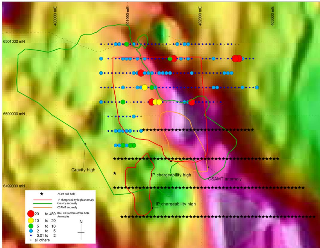
**Figure 2.** Map of the Illewong prospect with interpreted CSAMT, gravity and IP anomalies overlying a coloured total magnetic intensity image. The RAB98 drilling survey results are shown as ppb Au. The collar locations of the AC04 survey conducted for this study are shown as stars.
