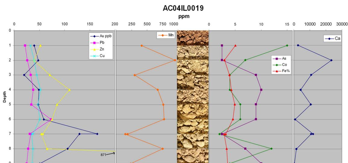
**Figure 5:** AC04IL0019, down hole geochemistry with photos of the dry samples.
