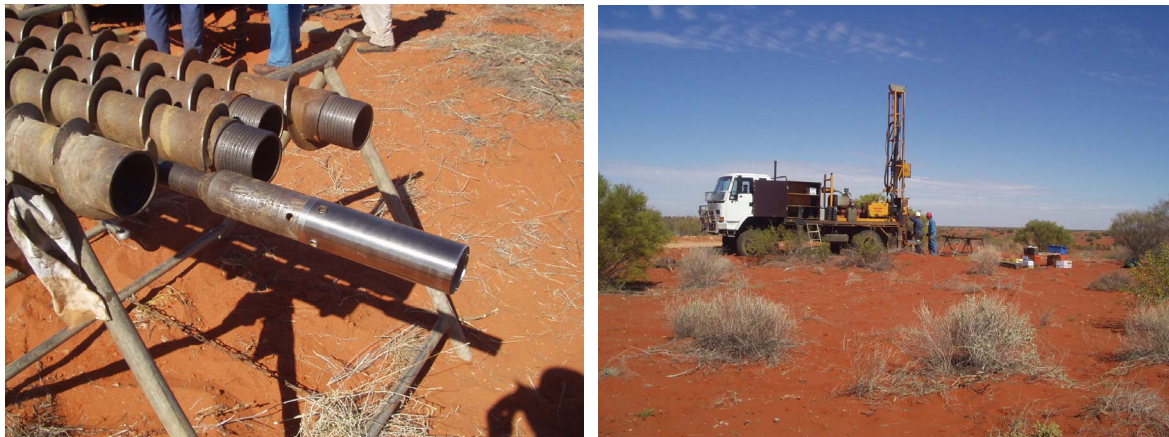
Figure 1 (left): 24cm OSL sampling tube for use with hand-operated or truck-mounted auger system. Figure 2 (right): Truck-mounted drilling rig using augers and sampler during collection in the Simpson Desert.
