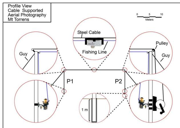
**Figure 1:** Design of cable supported platform for low altitude aerial photography
