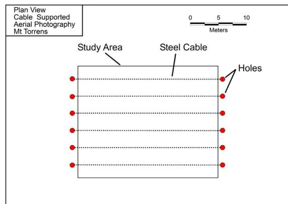
**Figure 2.** Plan view of cable supported platform for low altitude aerial photography
