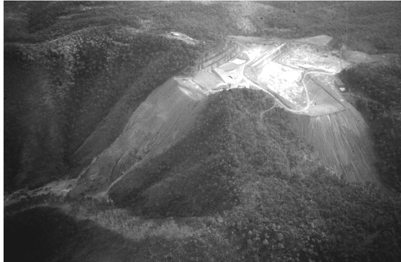
Figure 2: Gumigil Chrysoprase Mine. The mine has cut approximately 75m into the regolith of the Marlborough Ophiolite.
