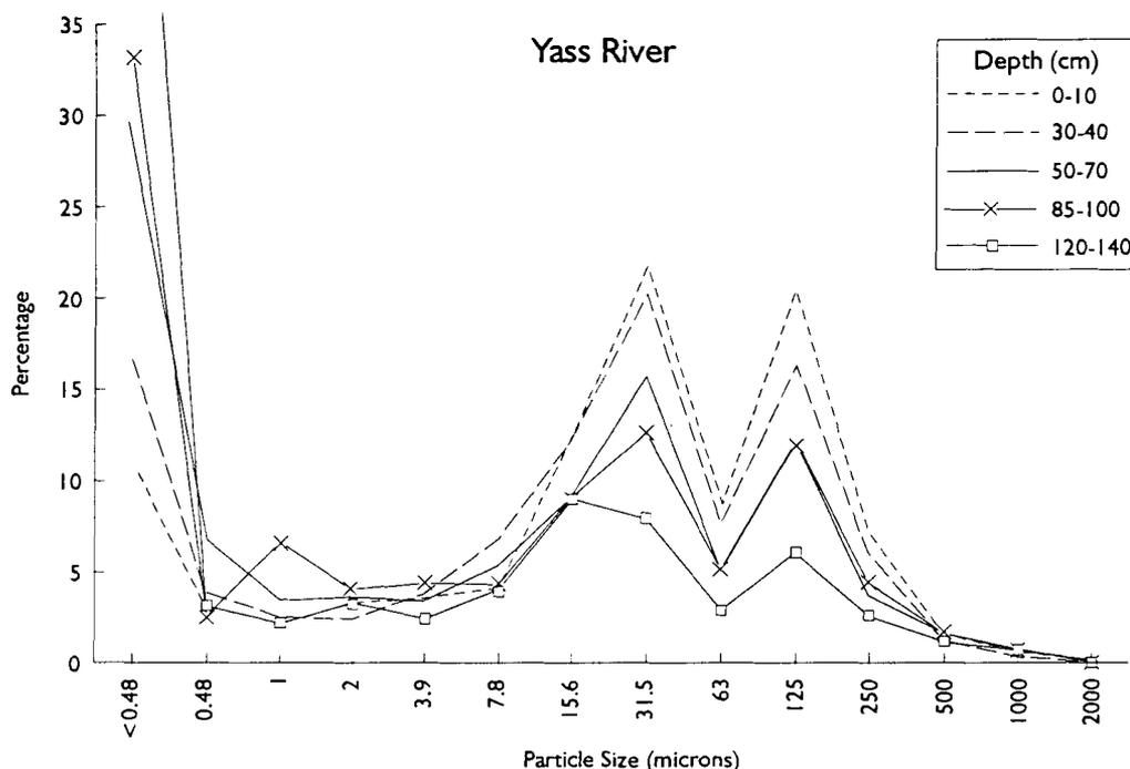
Figure 13. Particle size analysis for soils, Yass River.
