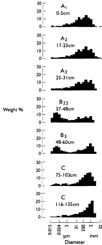
Figure 5. Particle-size histograms, Sutton Profile (after Walker et al., 1988)
