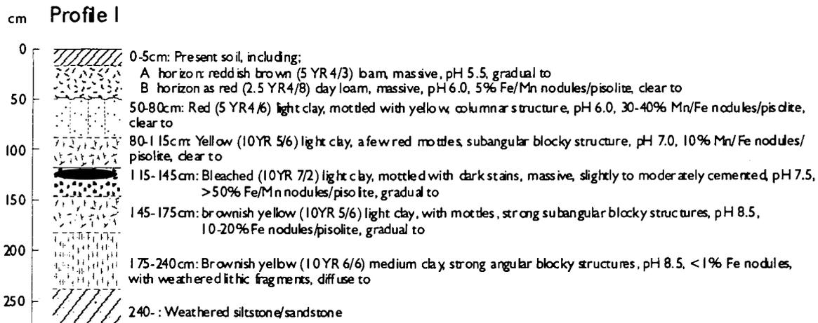
Figure 8. South Gundaroo road cutting and profile details.
