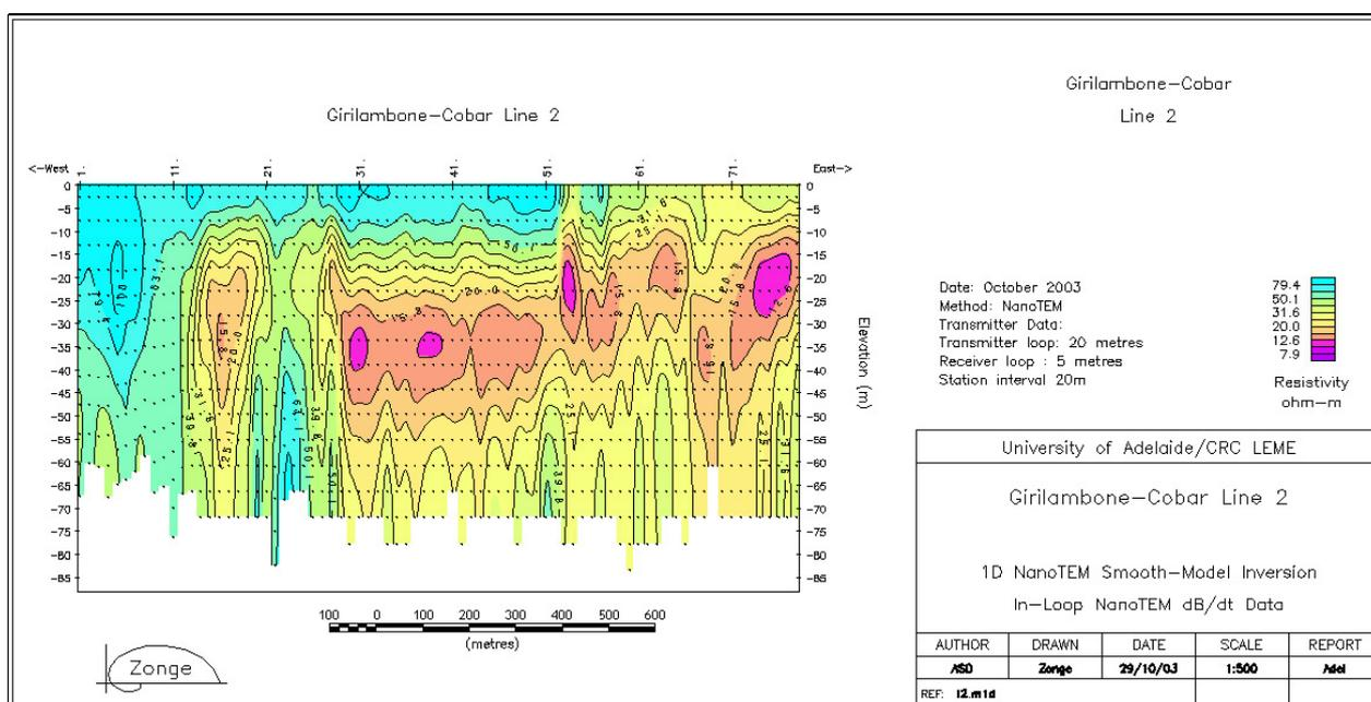
**Figure 4.2.** Depth-resistivity profile across a well-defined, shallow magnetic palaeochannel east of site 4 (from Davey & Joseph, 2004).
