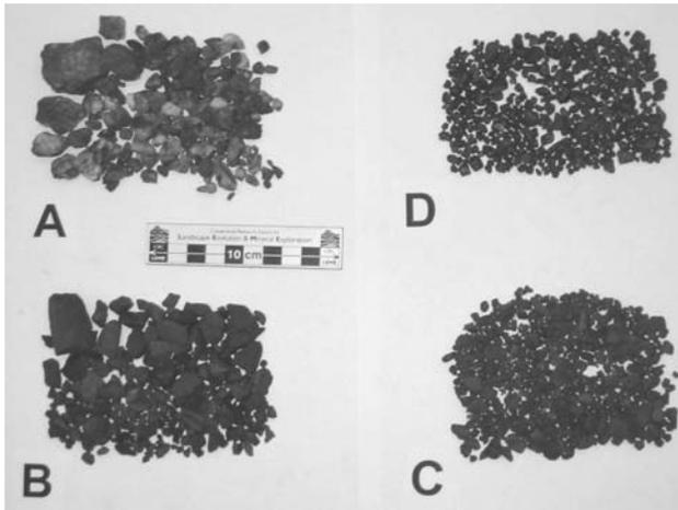
**Figure 2.4.** Separated lag fractions from Sample site 3, Yarrowonga Anomaly. (A) quartz fraction (B) lithic fraction (C) magnetic ferruginous fraction (D) non magnetic ferruginous fraction.
