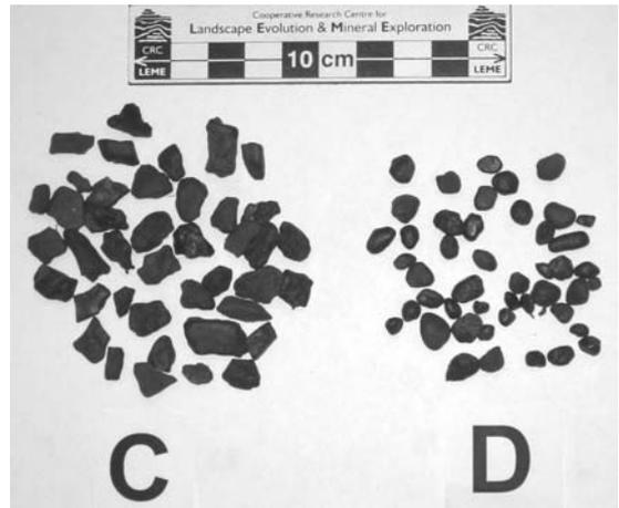
**Figure 2.5.** Magnetic ferruginous fraction separated into (C) angular and (D) rounded components.
