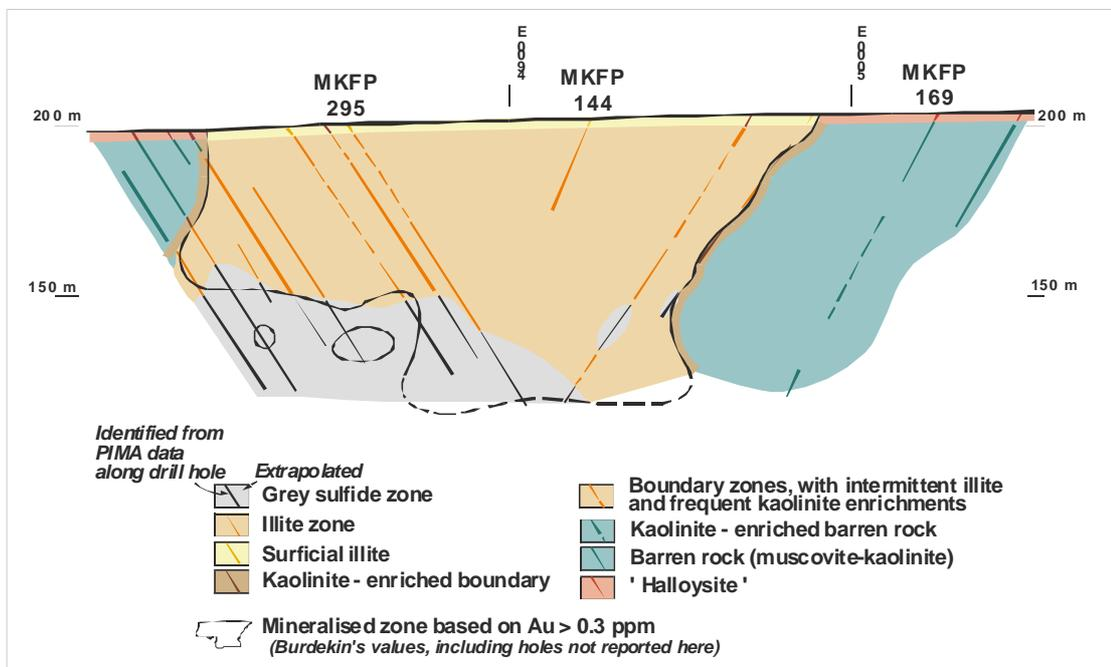
**Figure 3.2.** Cross section through the weathering zone of the McKinnons gold deposit showing the mineralogical variation, in particular the distribution of illite and kaolinite (from Marshall *et al.*, 1996).
