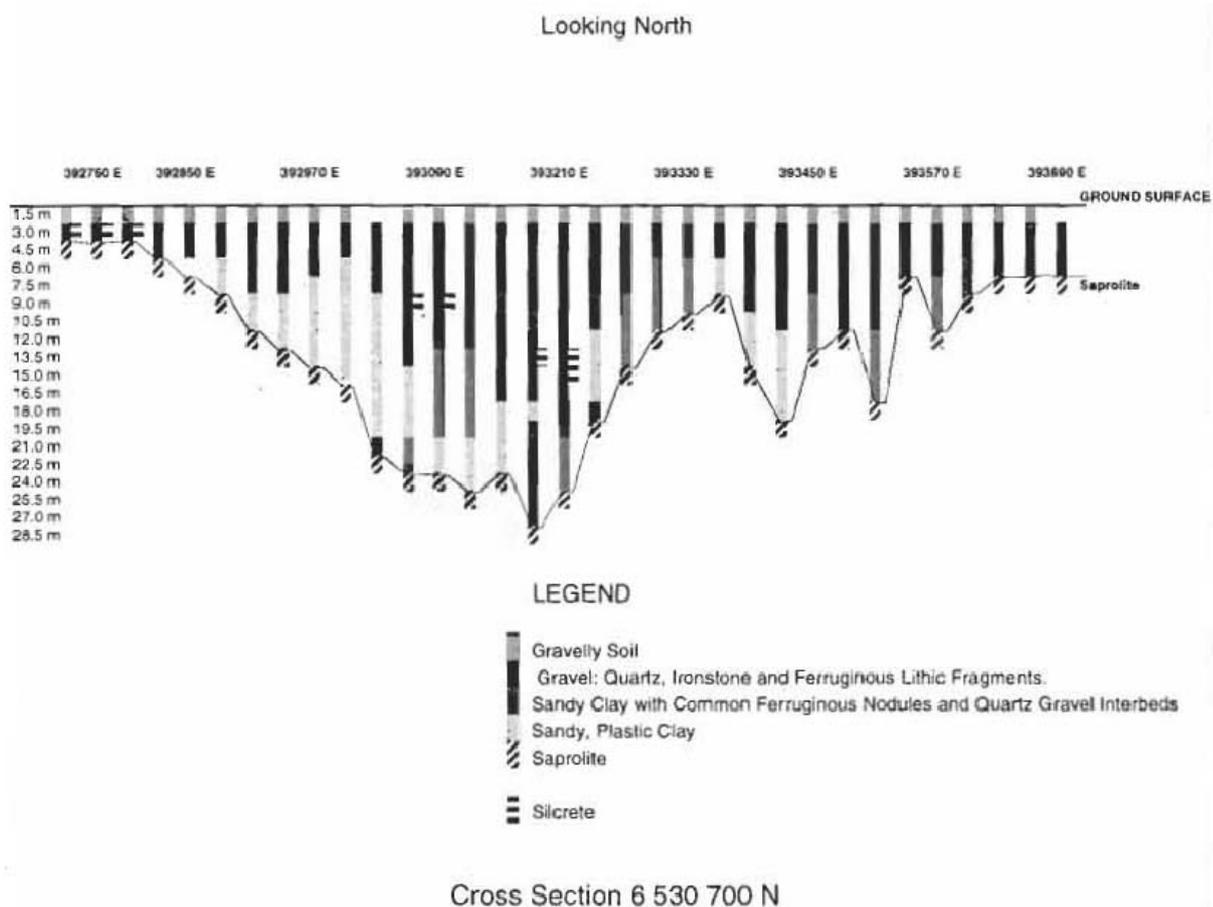
**Figure 1.2.** Cross section through the Bourke road palaeochannel system (from Ford, 1996).
