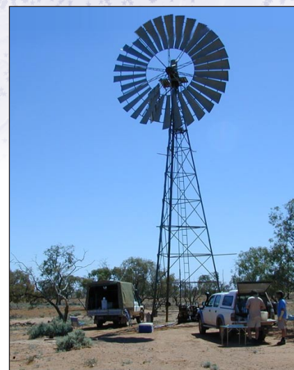
▲ Figure 1. Sampling groundwater from a windmill-driven pastoral bore in the southern Curnamona Province.
